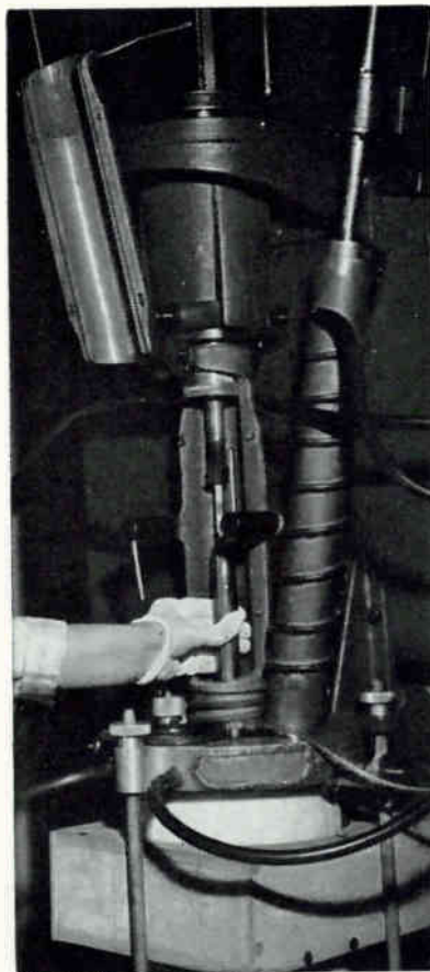
Crystal is removed through port
