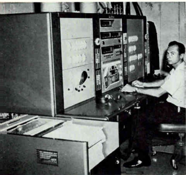
Monitor display console. Capsule observer position, right; capsule communicator position, center; aeromedical position, left
