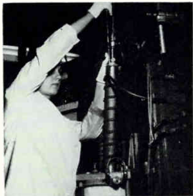
Billet is loaded into feed tube of crystal puller
