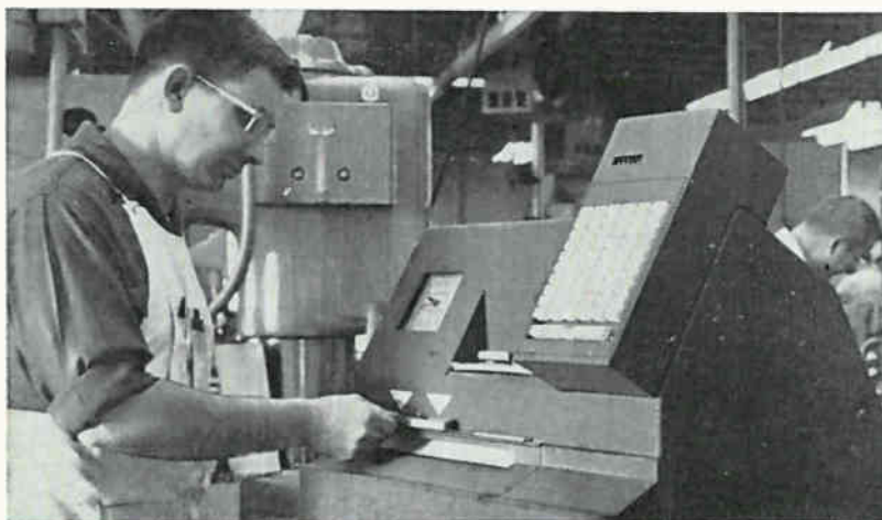
Unit by Standard Register provides data collection in both machine and man readable language for ultimate processing in solid-state translator, or manual keypunch
