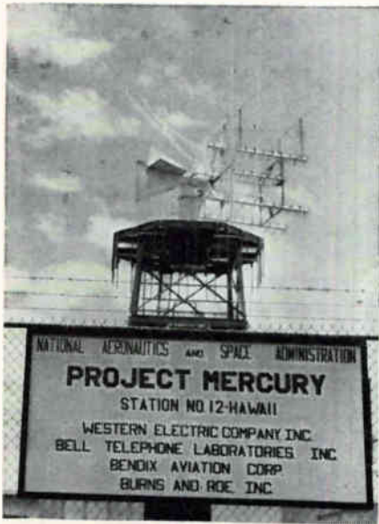
Entrance to Kokee Park Project Mercury site. Transmitting dipole is mounted on quad helix antenna (rear)
