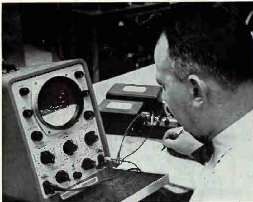
Operator observes scope display of simulated missile in flight. Source of each signal is labeled on scope. All signals are within performance limits except Vibration and Voltage 2
