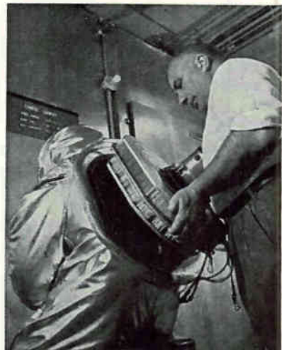
Thermoelectric unit by Westinghouse is fitted into back of experimental Navy climatic suit
