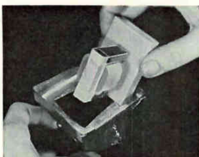
Transformer assembly is positioned
