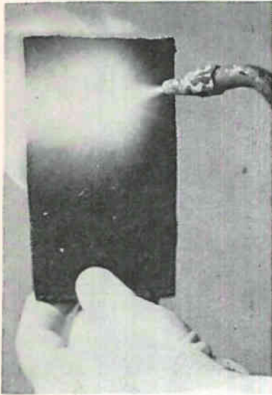
A ten-ply laminate of Pluton fabric, reinforced with a phenolic resin, withstands 2,750 C. Operator's fingers are just three inches from the hot spot
