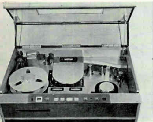
Video recorder to be introduced by Sony Corp. The two-head unit is compact, transistorized, has pushbutton control of console
