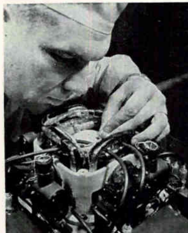
Prototype of 'electrically suspended' gyro is being developed by Minneapolis-Honeywell for Polaris sub navigation system
