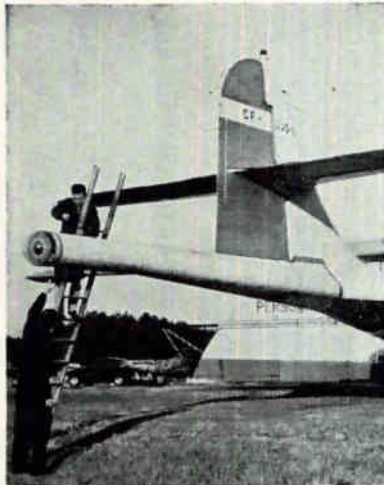
Tail cone (left) and nose frame mountings of EM detector elements equip Canadian Aero Service aircraft for electromagnetic surveys. Radiation counter, magneto meter and doppler radar are also carried
