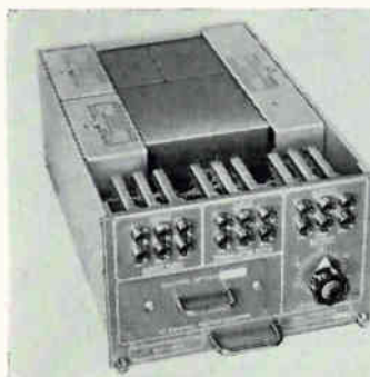
Two Multiplexers, Type 248 Model 1, are required for full utilization of the capacity of a radio transmitter. One is used to transmit telegraph, telephone, or facsimile signals from two vf circuits to the radio channel designated as sideband A. The second Multiplexer performs the same function for sideband B. In this way four vf circuits are applied to the twin-channel radio transmitter.
