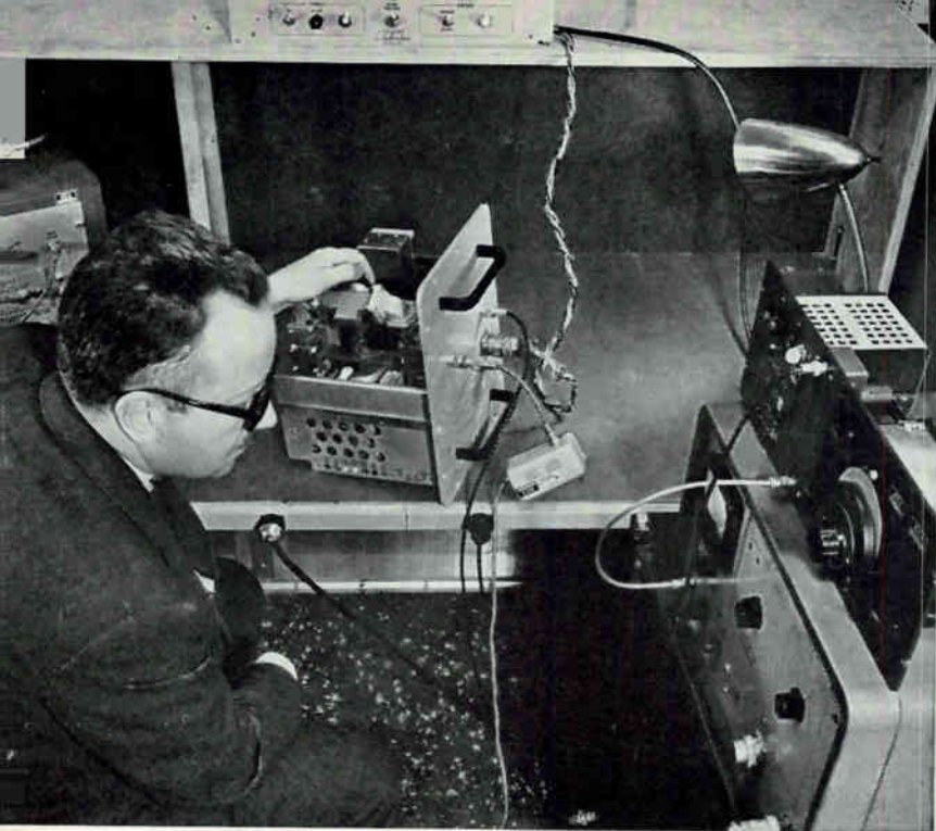
Photo at left shows author adjusting parametric preamplifier. The rear of the preamplifier unit is seen at right
