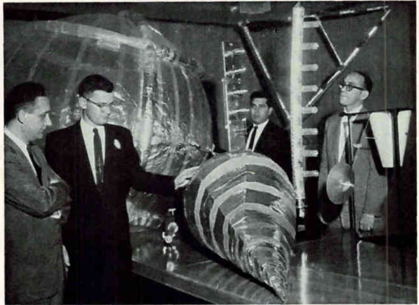
Inflatable antennas of Mylar film and aluminum foil are under study at Lockheed Missiles and Space Div. Sphere is highly directive; conical spire gives wide coverage. Antennas fold into small package, inflate in space
