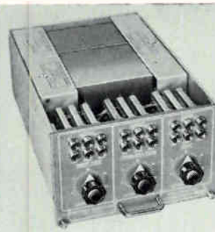
Two Demultiplexers, Type 249 Model 1, are required for full utilization of the capacity of a radio receiver. One is used to receive telegraph, telephone, or facsimile signals for two vf circuits from the radio channel designated as sideband A. The second Demultiplexer performs the same function for sideband B. In this way four vf circuits are derived from the twin-channel radio receiver.
