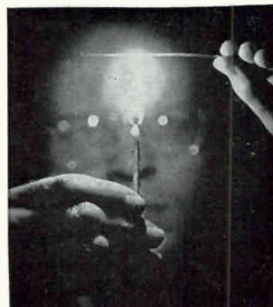
Permanent metallurgical bond is assured between solder and base metal. Even when liquid, continuous conductive coating of tin-gallium clings to base metal in smooth uniform layer. Chief use: for stamping base tabs to support the silicon or germanium wafer in transistors. Developed by Alpha Metals, Jersey City, N. J.
