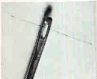
In view magnified 10 times, mineral thread easily slips through eye of needle for size comparison
