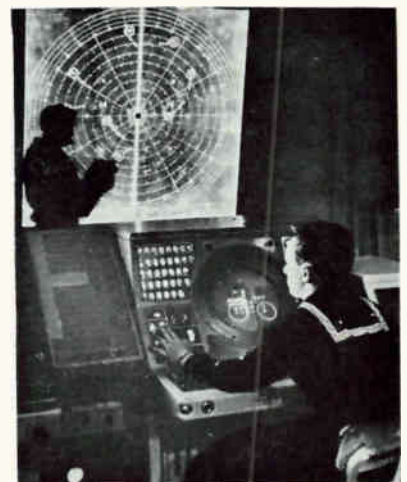
New battle display console (foreground) by Hughes Aircraft shows aspects of air, surface and submarine action for fleets. Rear: the grease-pencil method
