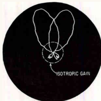
FIG. 4—Antenna pattern of the dual Yagi array mounted on a C-130A aircraft
