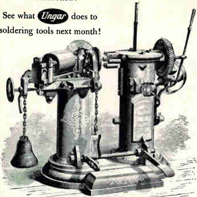
Machine for Rounding Heads of all sizes for Kegs and Barrels • E. & B. Holmes • Circa 1870
