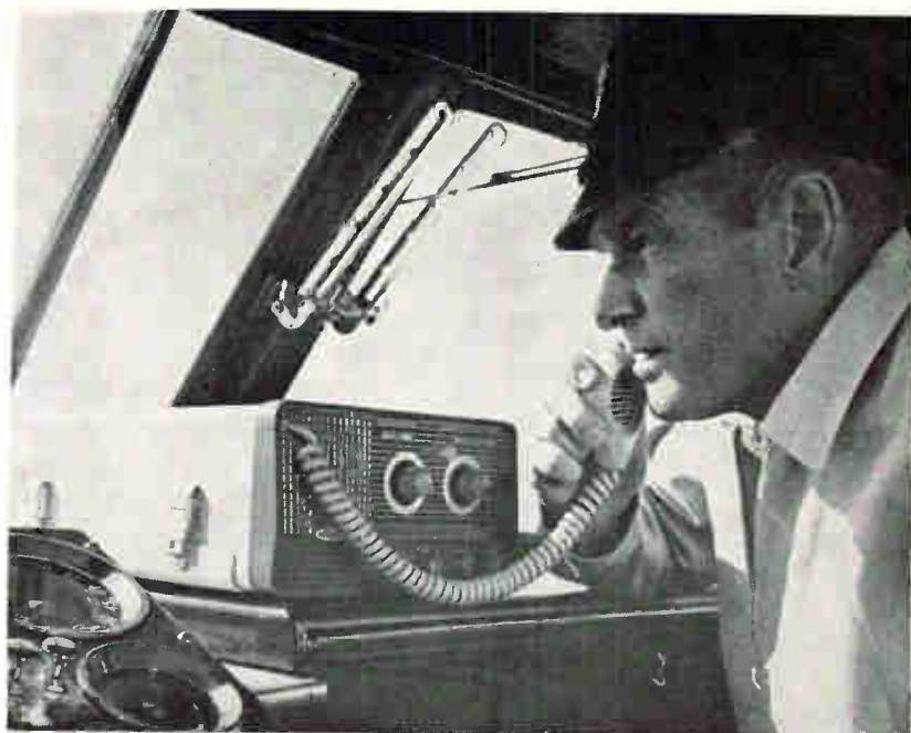
Along with depth finders, radiotelephones dominated the show. This Raytheon unit has eight crystal controlled channels, broadcast band, corrosion proof plastic panel, epoxy painted aluminum cabinet
