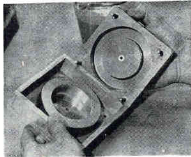
Mold is released from pattern
