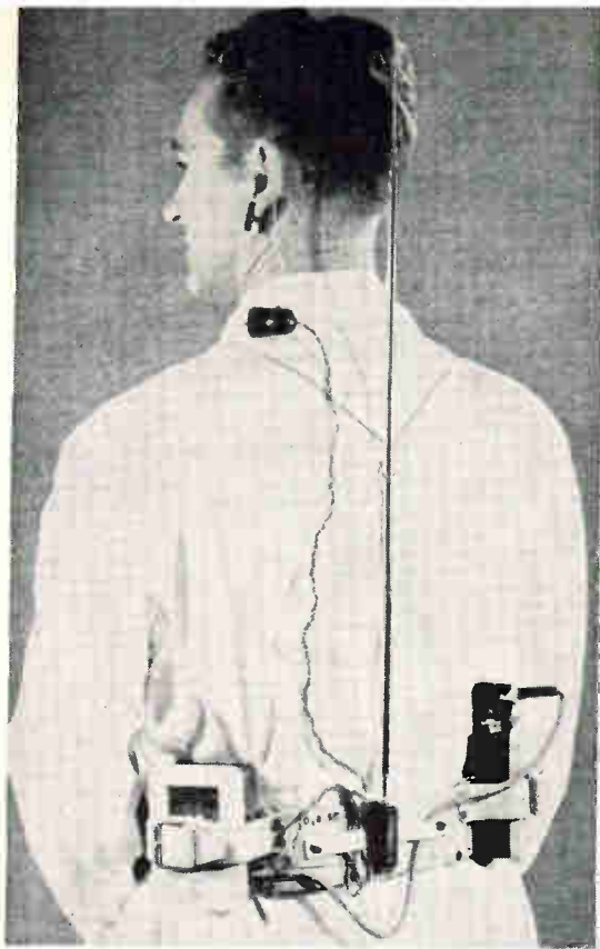
Subject wears clip, transmitter, batteries and antenna. One box contains all electronic components, encapsulated in Plexiglass for strength; the other box contains batteries
