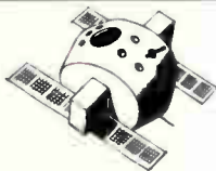
Orbiting Astronomical Observatory —Standardized, 3500 lb. satellite, for several experiments with different scientific sensors and specialized devices.
