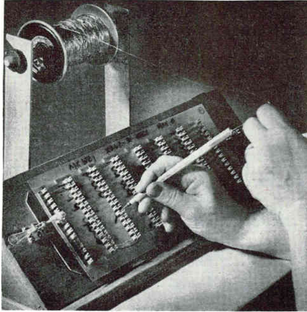
Pencil is used to thread jumper wire along route marked on template
