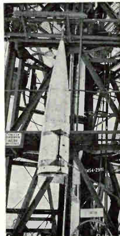
Nose cone being raised up tower for mating with main rocket body
