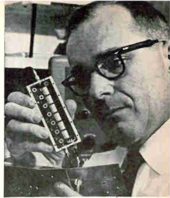
Author examines compact six-stage amplifier. All components are mounted on printed-circuit board. Cover has innerstage shields that mesh with triode connections
