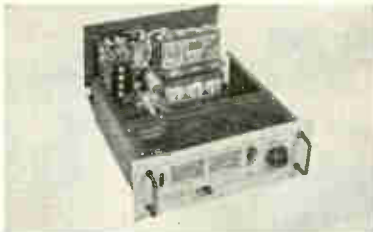
"Flip Top Box" Permits Accessibility For Maintenance
