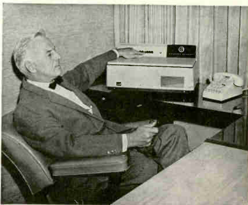
Lawyer plays back telephone messages recorded on his Electronic Secretary answering set during his absence
