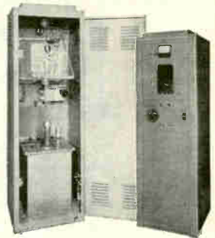
Vacuum system holds paper in place as transistorized weather plotter draws isobar patterns for forecasting use
