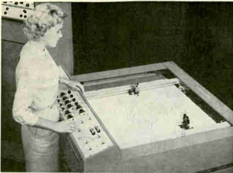
Vacuum system holds paper in place as transistorized weather plotter draws isobar patterns for forecasting use
