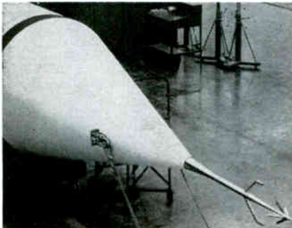
Inconel-sheathed total temperature probe mounted on Redstone missile nose cone — assures high strength at high temperatures and readily withstands oxidation, erosion and thermal shock at extreme velocities. Probe (shown at right) is product of Aero Research Instrument Company, Inc., Chicago, Illinois.
