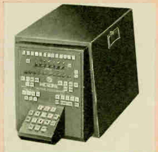
FIG. 2—This MicroPac tactical field computer is one of two equipments being delivered by RCA under the U. S. Army micromodule production program
