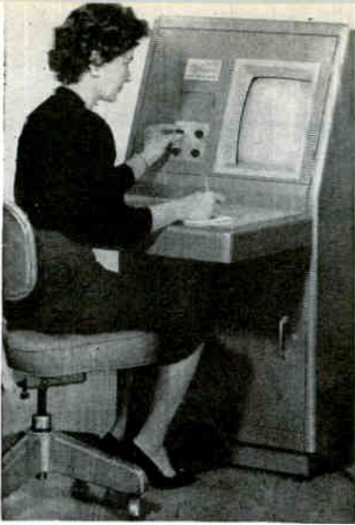
Inquiry station displays information requested from computer. It is part of A. G. Dick Videograph
