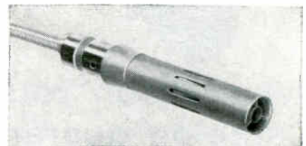
Inconel-sheathed total temperature probe mounted on Redstone missile nose cone — assures high strength at high temperatures and readily withstands oxidation, erosion and thermal shock at extreme velocities. Probe (shown at right) is product of Aero Research Instrument Company, Inc., Chicago, Illinois.
