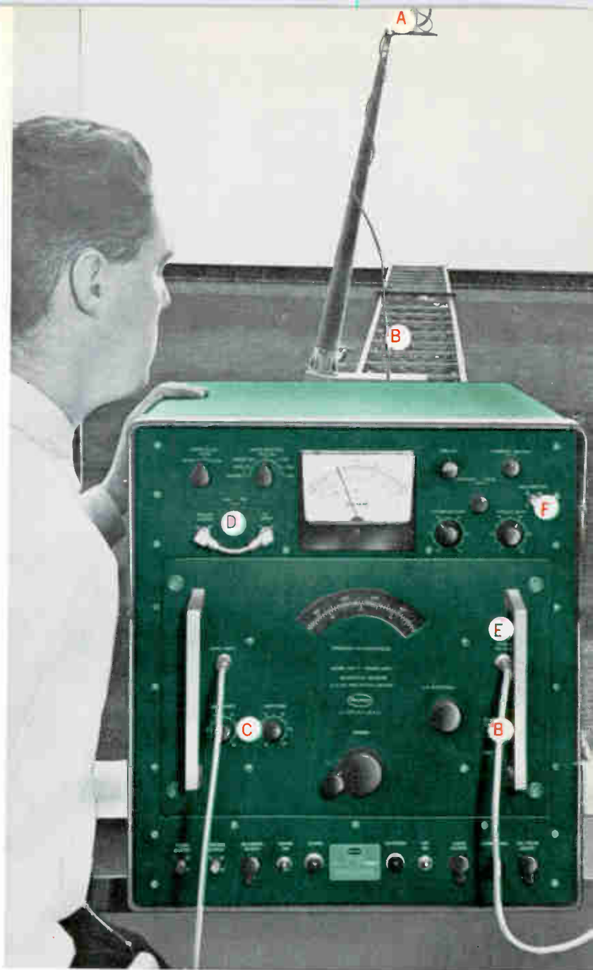
Model RW-T Microwave receiver being used to make antenna pattern measurements on Polarad range.
