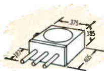
THE MODEL 50 3/8" square, 3/16" high, and weighing 1 gram, the Model 50 is available in standard resistances of 50 ohms to 20K ohms.
