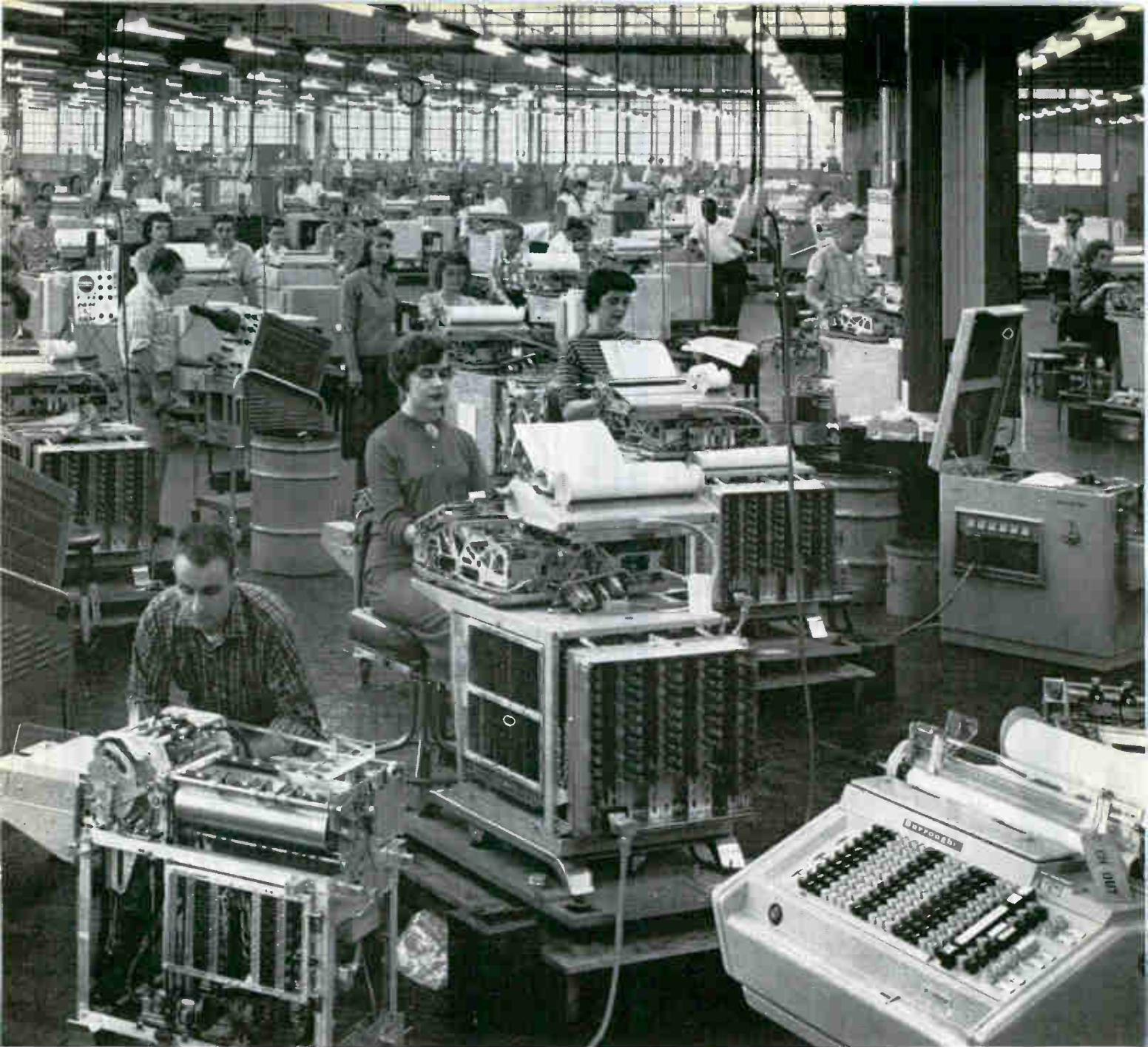
Electronic accounting machines are inspected at Burroughs Corporation's Plymouth Plant, Plymouth, Michigan.
