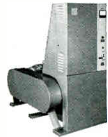
Typical Generator for H-F Industrial Installations
