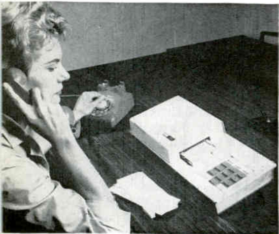
Transmitting punched-card information over telephone lines with IBM's 1001 data-transmission system
