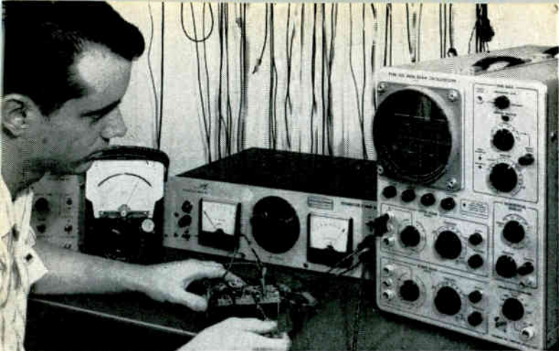
Technician adjusts the circuit for optimum ratio of R_1 and R_2 (see Fig. 2) for best stabilizing performance
