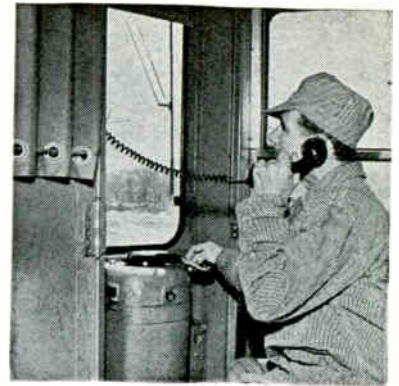
Chicago El line supervisor (foreground, left photo) flips control box switch and gets operating information from motorman aboard train
