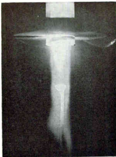
Artificial sapphire is produced by melting end of aluminum oxide rod
