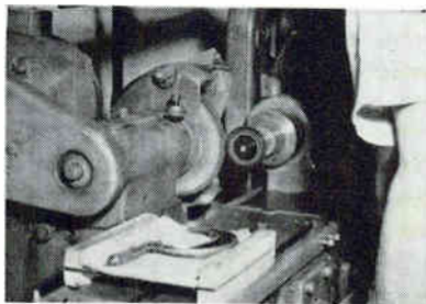
Idler wheels are trued on grinding machine
