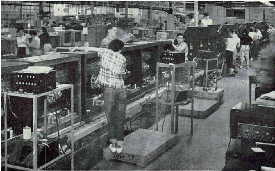
The final assembly line at Thomas Organ. Instruments are tuned with electronic stroboscopes in five minutes by factory workers
