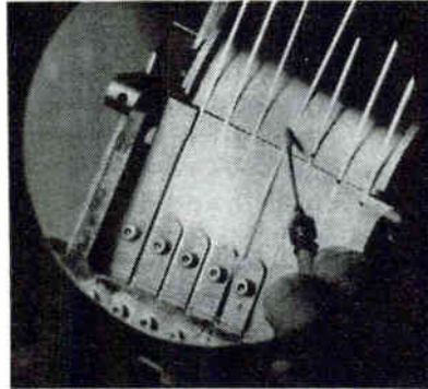
FIG. 2—Rows of dendrites are fed through a scribing machine, (left), each strip being cut into tiny germanium dice approx. 50/1,000-in. long. Each wafer forms a single transistor (right)
