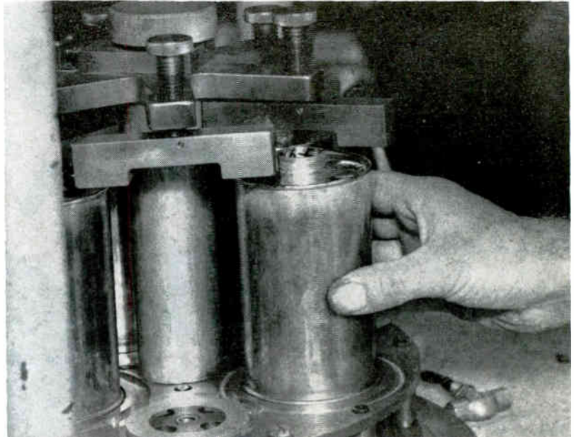
Sealing fixture is loaded with can-type housings before bell jar is lowered. Cans are evacuated and gas filled through hole in bottom
