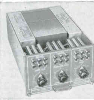
Two Demultiplexers, Type 249 Model 1, are required for full utilization of the capacity of a radio receiver. One is used to receive telegraph, telephone, or facsimile signals for two vf circuits from the radio channel designated as sideband A. The second Demultiplexer performs the same function for sideband B. In this way four vf circuits are derived from the twin-channel radio receiver.
