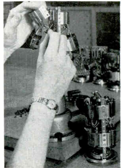
Sealing fixture is loaded with can-type housings before bell jar is lowered. Cans are evacuated and gas filled through hole in bottom
