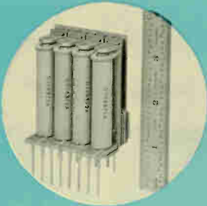
FIG. 1—Automatic Electric's new wire-spring relay (A) transfers up to 51 circuits quickly for 100 million or more operations without readjustment. The company has a space-saving relay with a common heel piece and a common fixed contact assembly (B), which is used in data processing equipment.
