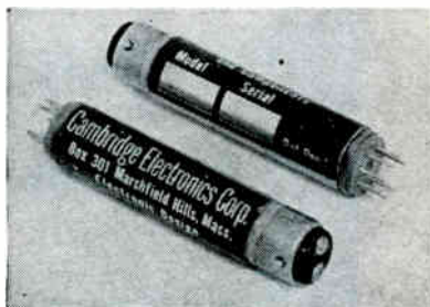
Photomodulator package. Design geometry isolates photosensitive material from modulating voltage
