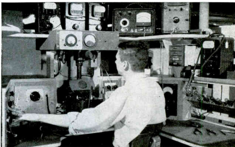
Vtvm calibrator watches scale through projector while shifting test frequencies with pushbuttons at his left hand
