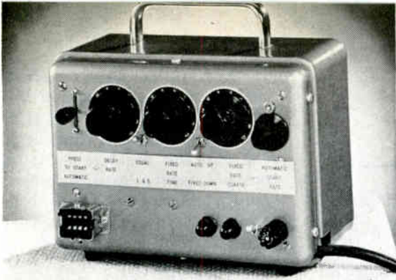
Relay contacts are brought out to plug on front panel
