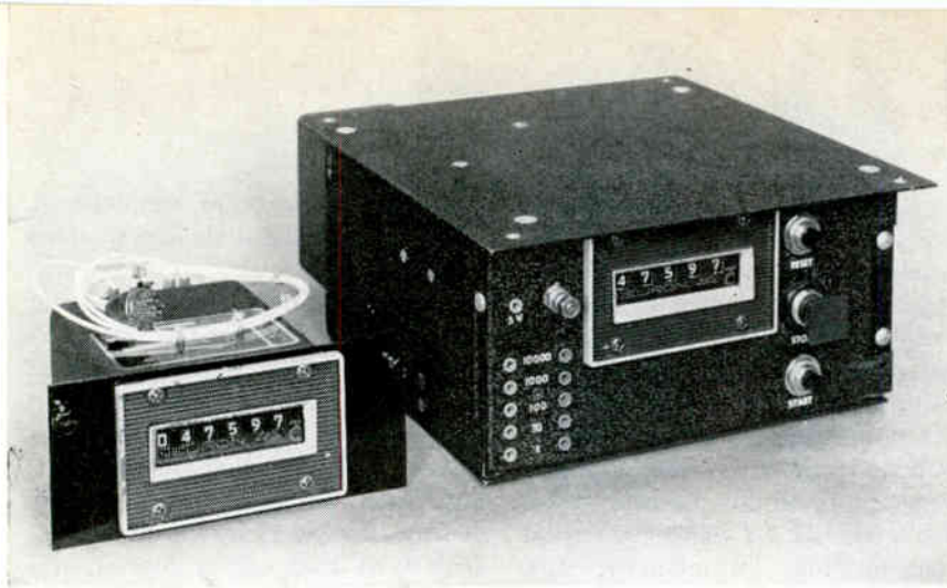
Display equipment of B-66 radar development instrumentation system shows at left the remote repeater for the cockpit
