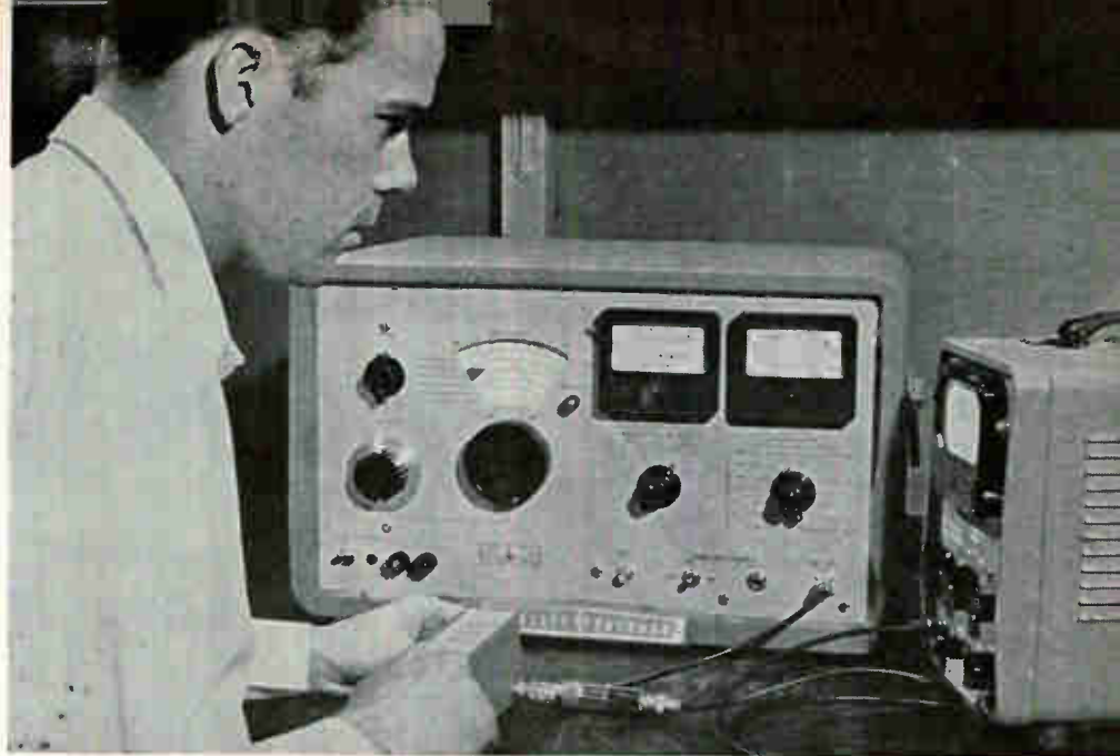
Output of production unit is within \pm 1 db from 50 Kc to 65 Mc
