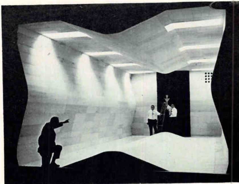
Radio wave absorbing lining in Republic Aviation's 40-ft anechoic chamber minimizes interference in advanced antenna performance tests
