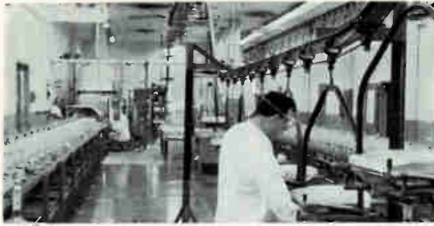
View of line from unloading station. Long length of conveyor permits heated epoxy to set before the tube and shield assembly is transferred
