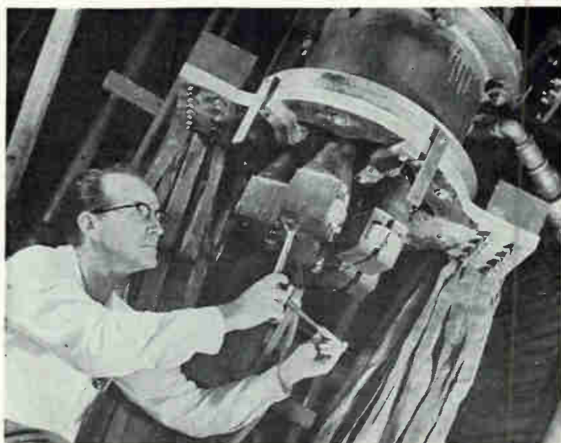
Grain refining unit goes on arc-melting furnace at Westinghouse metals plant. The combination improves properties and yield of metals
