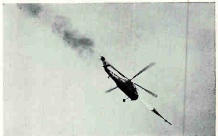
Bullpup, radio-guided air-to-air missile built by Martin, is launched from helicopter in recent tests. Missile is 12½ ft long, weighs 570 lb
