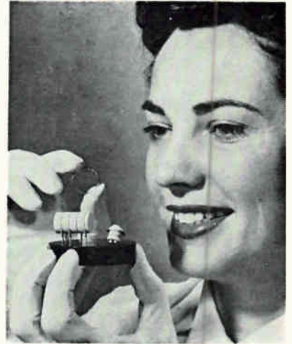
Two gold-plated ceramic receiving tubes made at the General Electric tube plant in Owensboro, Ky., are used in the transmitting equipment of the Pioneer IV, and the Thor-Able Star missile which put the TIROS 1B into orbit
