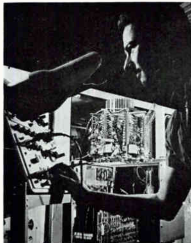
Oscilloscope checks operation of Librascope memory drum used in GPL's air traffic control system
