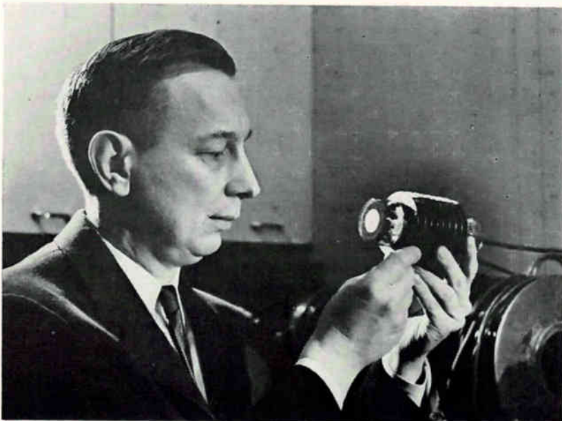
The Astracon, a small tube developed by Westinghouse, now makes it possible to see individual electrons released at the tube's input. In astronomy, the tube will increase the light-gathering ability of the largest telescope. In nuclear physics, the tube will permit the viewing of the tracks of high-energy cosmic rays and other particles
