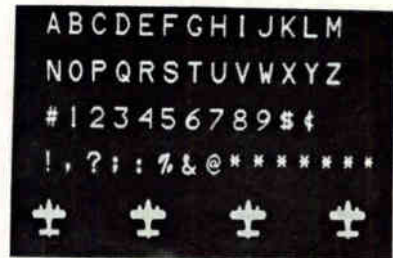
FIG. 1—Generated characters displayed on conventional crt; enlarged view of character shows raster structure
