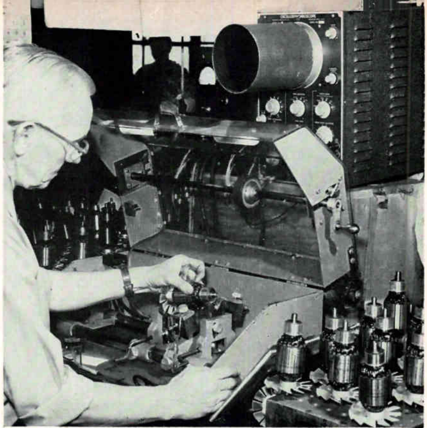
Armatures are rotated during test, so that each coil is examined in turn
