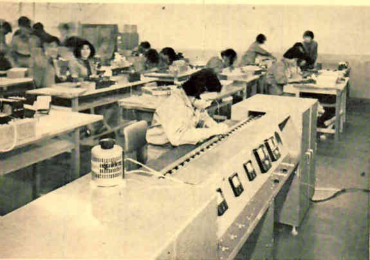
Automatic test equipment for ceramic capacitors at Murata Mfg. Co. measures Q factor, capacitance, resistivity, dielectric strength, at rate of 1,200 units per hour
