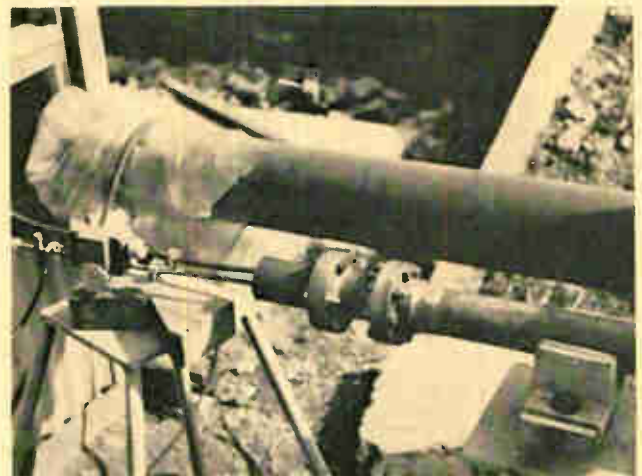
Above: test facility at Sumitomo labs where X- and O-type waveguides are checked out; below: closeup of 35-gigacycle coupling under test
