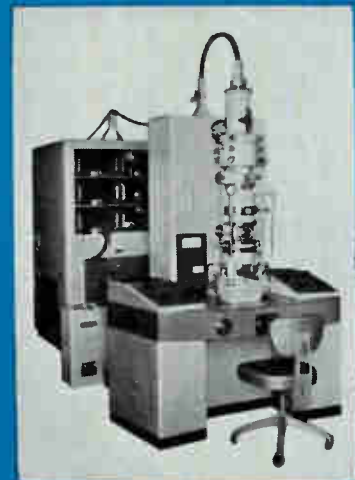
▲ Hitachi Electron Microscope with a Direct Magnification of 250,000 Times
