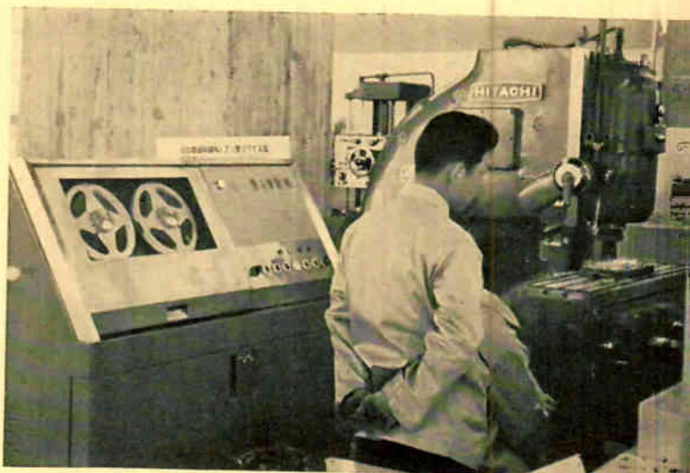
Numerical controls for Hitachi milling machine include transistorized special-purpose computer HIDAM. Machine costs 14 million yen—about $39,200
