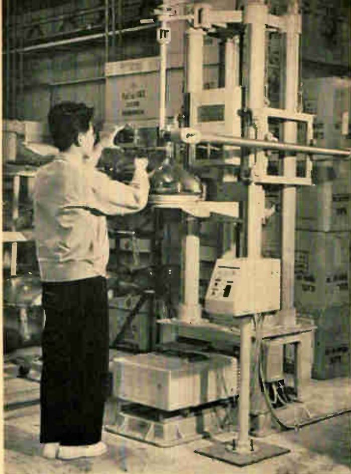
Polarimeter (closeup above) in use on Kobe Kogyo's tv-tube production line to test for strain in glass
