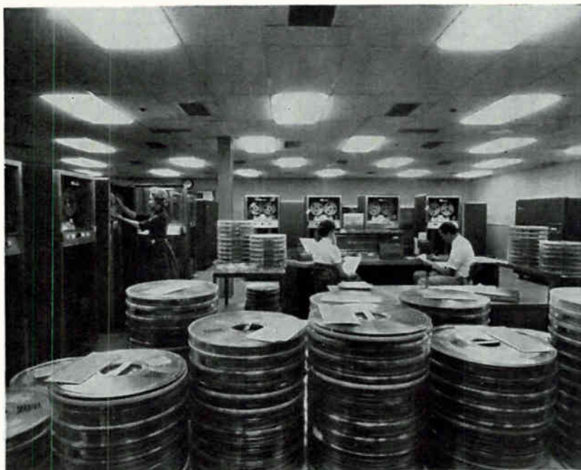
Information received by microwave at North American's Los Angeles computer room is recorded on IBM units for processing, playback
