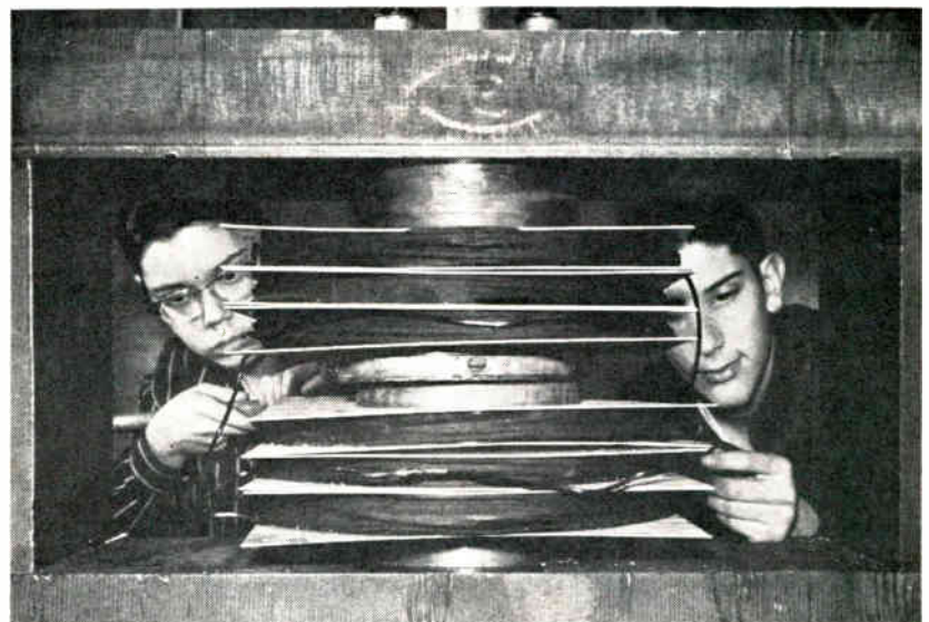
Two-ton magnetic unit is studied by Levittown High, N. Y., student members of JETS (Junior Engineering Tech Society), who will use it in a cyclotron they are building. JETS is a nationwide group sponsored by industry and education.
