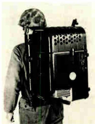
Portable power pack using 30 ion-membrane fuel cells and weighing about 30 lb is reported by GE to be under development for Marines and Army. Cutaway shows cell setup
