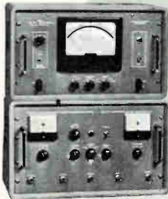
Plotting Phase and Amplitude Characteristics of Crystal Filter.
