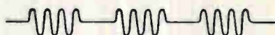
FIG. 7—Because this function can be treated as a product of a pure cosine function and a rectangular waveform, its frequency spectrum can be analyzed by graphical convolution techniques
