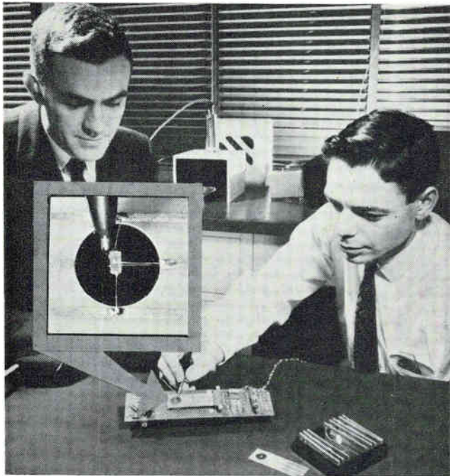
GM Research Labs' cadmium sulfide transistor (insert left) acts as audio amplifier when struck by light beam. Right: Chrysler's telemetry system records results of dynamic tests on new brake design for later evaluation and analysis
