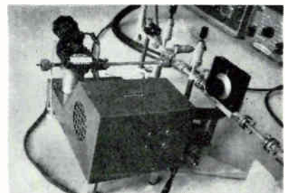
Experimental set-up for millimeter-wave klystron amplifier at left. H-plane tee, E-H tuners, crystal mount and variable attenuator on right
