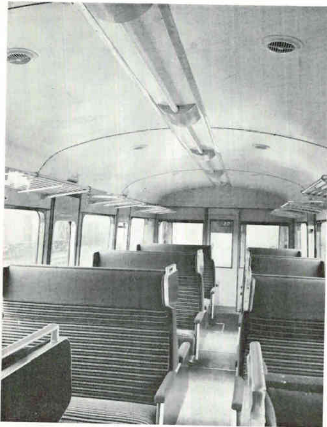
New British railway coach uses fluorescent lighting
