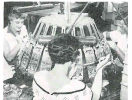
Demodulators are assembled by 3 operators working together on motorized rotary wheel
