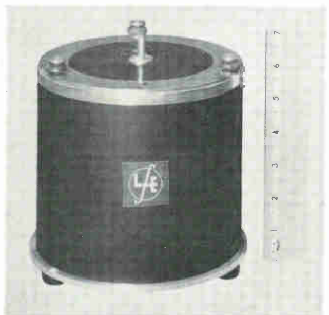
FIG. 8—Magnetic disk memory unit is designed to operate from a solar cell
