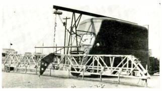
FIG. 6—Transverse profilometer truss can be quickly leveled and probes activated by equipment in truck. Motor-driven carriage (left bottom of truss) records analog of profile
