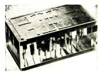
Encapsulated dual flip-flop with plated connections and etched wiring. Unit is 2 inches long
