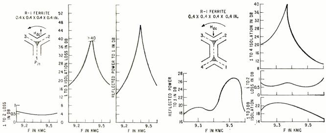
FIG. 6—Data for Y-type circulator. Wave travel is from port 1 to 2 FIG. 7—Data for 4-port circulator. Wave travel is from port 1 to 2
