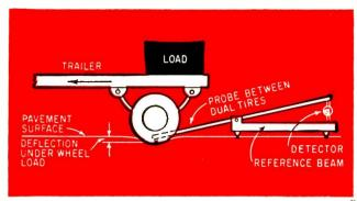
FIG. 3—Benkelman beam used to measure road distortion due to applied load as truck passes probe at creep speed. Road deflection is indicated on detector
