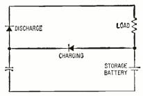
FIG. 3—Increased voltage across capacitor as temperature increases recharges storage battery through discharge diode
