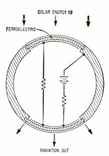
FIG. 5—Solar energy could be converted into a-c voltage with this arrangement
