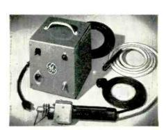
A NEW G-E RESISTANCE SOLDERING TOOL provides void-free solder joints for reliable, high-quality connections required by aircraft and missile applications. The new tool eliminates tip arcing or flashing, preventing pitting; is handoperated, requiring no pedals; and features a zirconium-tungsten electrode that does not require frequent redressing, maintenance or replacement. Write for Bulletin GEA-6588.
