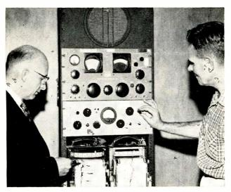
Two of the authors demonstrate continuous fading rate recorder. Chart on left records radio signal fading rate
