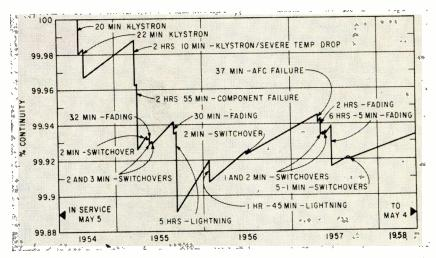
FIG. 1—Typical microwave system (Canton-Philo) provides reliable operation. Records show a continuity about 99.88 percent for the system or 99.97 percent per hop
