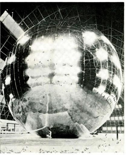
NASA's 100-ft aluminized polyester film sphere will fold inside a 28-in. diameter container at launching of passive balloon satellite
