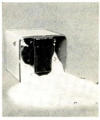
Since the alumina powder maintains its granular characteristic, the component can be filled or emptied at will for repairs or changes
