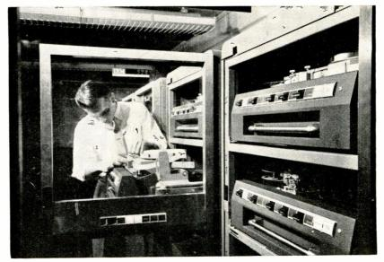
Federal Aviation Agency has tied in an IBM650 at Indianapolis Air Route Traffic Control Center with Univac File-Computers at Washington, Cleveland and Pittsburgh ARTCs. Paper tape equipment (pictured) provides multiple direct connections between wire links and the computer. Incoming message traffic is automatically edited, checked and sent to the computer; outgoing flight plans are devised and routed to proper adjoining centers. Boston and New York computers will join the network shortly
