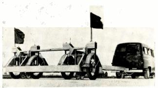
FIG. 4—Longitudinal profile of road is highly correlated with road performance. Slope-detecting wheels are located between the two pairs of large riding wheels
