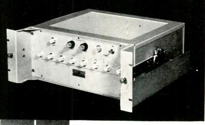
THE PM-406 is a combination instrument comprised of a preamplifier and multicoupler located on a single chassis for rack mounting. This unit permits the coupling of eight receivers to a single antenna and is designed for use where short runs of cable from the antenna are employed. These units are of the "bath tub" chassis design having a 3-inch recessed front panel to permit patching cables to hang without protruding. Modifications of this design are available on special order.
