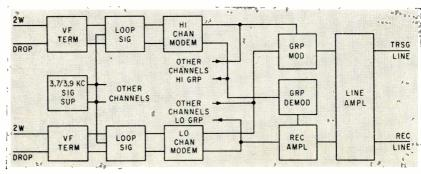
FIG. 6—Terminal of telephone carrier system. Four terminals can be mounted in one 11-ft,
