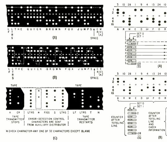
FIG. 4—Horizontal check line (A), spiral check line (B) and errordetection control characters (C) used in odd-even count error detection system
