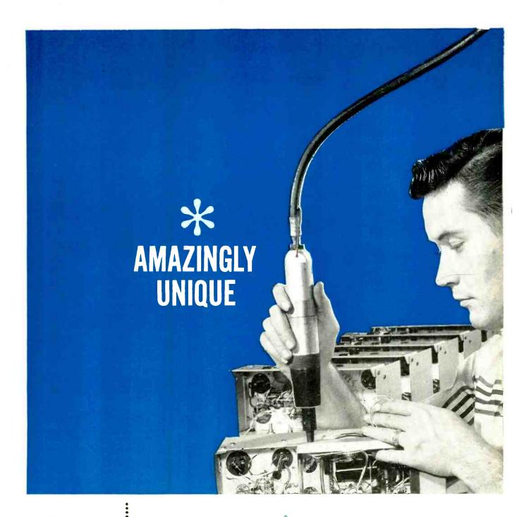
\*Clecomatic stands alone as the only automatic start and stop screwdrivernut runner with positive torque control
