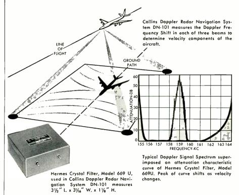
Collins DN-101 Doppler Radar Navigation System is an airborne radar transmitting and receiving system which directs three beams of X-band energy towards the earth and then accurately measures the amount of frequency change between the transmitted and reflected signals to determine the lateral, vertical, and horizontal velocities of the aircraft.
