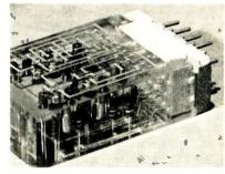
Transistor inverter package with deposited wiring and plated connections
