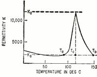
FIG. 2—Permittivity curve of barium titanate as temperature is varied around Curie point, T<sub>c</sub>, applies only with low field strength
