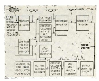
FIG. 1—This recorder diagram shows progressive transformations of i-f signal input
