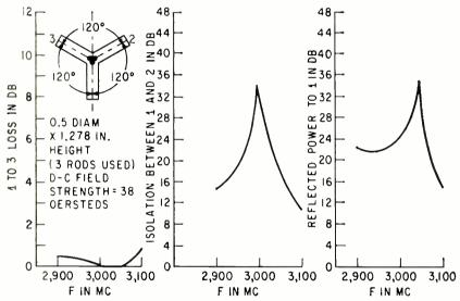
FIG. 8—Test data for S-band circulator whose wave-travel direction is from 1 to 3
