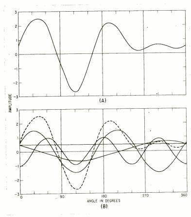
FIG. 1—Complex wave (A) is broken into its harmonics and baseline (B) by using form shown in Fig. 2. Dotted line shows check obtained by adding harmonics and baseline at each point
