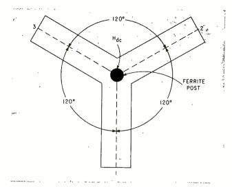
FIG. 1—Circulator's cylindrical ferrite produces transverse d-c field
