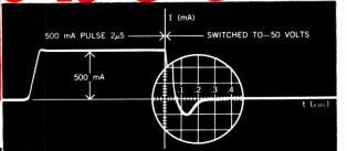
... in a high-current silicon switching diode. The 1N920-1N923 series is the latest result of Sperry Semiconductor's unique developments for the computer field.
