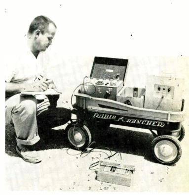
FIG. 8—Crushed stone base material density measured by backscatter from Cs<sup>137</sup> source and indicated on wagon-mounted scaler
