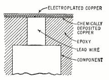
FIG. 1—Detail of plated connection
