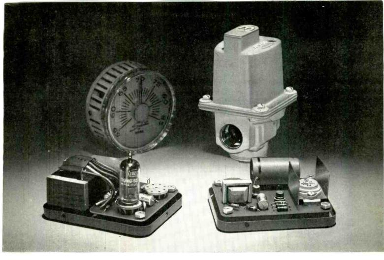
End alternate chills and hot blasts. Shown in front of the thermistor wall unit and the furnace modulator valve are the tube type and transistorized amplifiers for the new Selectra home gas furnace control now in production at Maxitrol Company, Detroit, Michigan.
