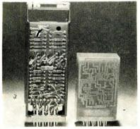
Flip-flop with deposited wiring and plated connections (right) contains components identical to those in the conventional package
