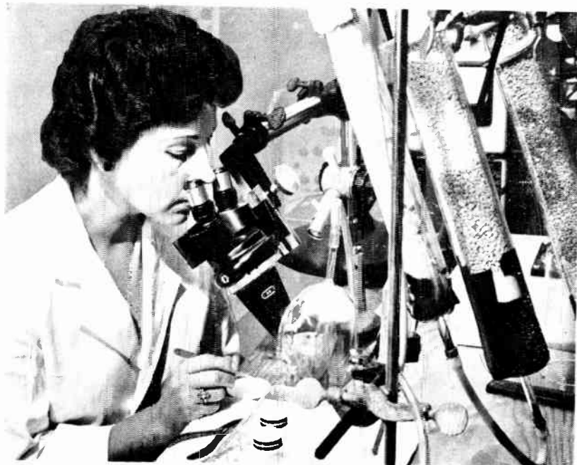
THE FRONT COVER —Technician prepares to attach leads to tunnel diode with aid of micromanipulator. Diode is assembled in bell jar containing inert gas
