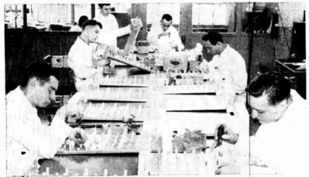
Component test fixtures are prepared on assembly line. Similar line is used to load components. Fixturing techniques save time, permit maximum utilization and versatility of environmental test equipment
