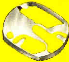
Full stock thickness at top of draw on .018 brass case improved watch quality and saved assembly time.
