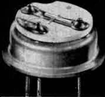
Greatly magnified photo of silicon transistor showing Fixed Bed Construction. All parts are firmly fastened, with no suspended parts except wire lead. Transistor reacts as a solid block in resisting shock and vibration. Power dissipation is inherently higher.
