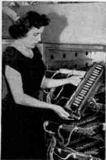
Load life and temperature cycling tests are made in this oven under controlled conditions.
