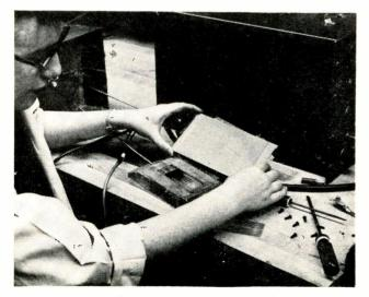
Thin ferromagnetic films—a couple of molecules thick—are future logic elements for microwave computers. IBM researcher here prepares to test field penetration
