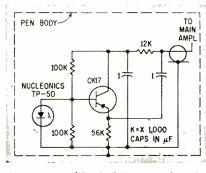
FIG. 3—Preamplifier built into pen-shaped holder
