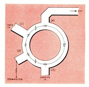
FIG. 1—Hybrid ring NOT circuit. Signals interfere destructively at (4); ring geometry also makes carrier cancel itself at (1) when information signal is not present, thus keeping the carrier out of the information line
