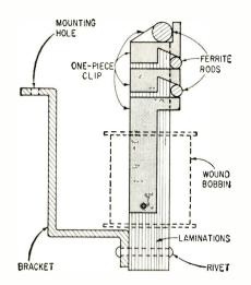
The clips shown in Fig. 1 (looking from inside the laminations) are slipped over the inside edges of the lamination stack. The clips are made of copper spring alloy and hug the stack ends on two sides.
