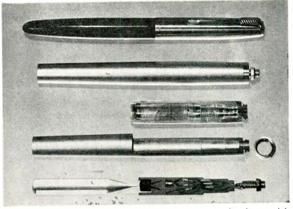
Disassembled pen with light-pipe lens and preamplifier mounting board removed is shown at bottom. Above is assembled light pen, at top fountain pen for size comparison
