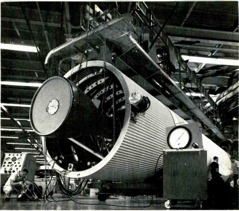
Jupiter IRBM Missile in final test and checkout area where actual flight conditions are simulated, at the Chrysler operated U.S. Army Michigan Ordnance Missile Plant near Detroit.
