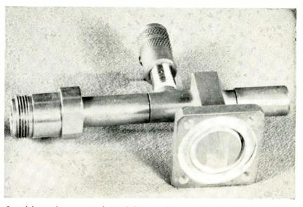
Crystal harmonic generator designed for second harmonic output over 12,500 kc to 14,500 mc
