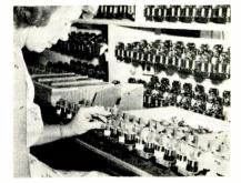
Assembling Increductors, Completed units are in storage racks
