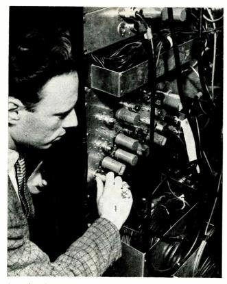
Coaxial cable served as distributed-parameter delay in this experimental 50-mc adder, an early IBM approach to microwaverange computers
