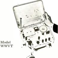
A 6-position dial switches instantly to any Standard Frequency - 2.5, 5, 10, 15, 20 or 25 mc. It is small, light-weight and rugged - sealed metal case and potted components, all transistorized and battery operated, and has better than 2 mv sensitivity. Priced at \$545.00
