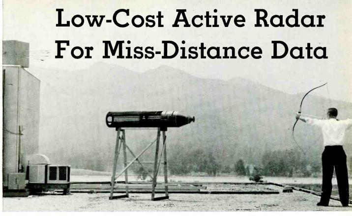
Old-fashioned ballistic missile (arrow) is used to check a new miss-distance indicator. The mdi can detect objects at closing speeds up to Mach 10 and at altitudes to 100,000 feet
