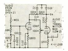
FIG. 1—Electronic impedance matching circuit between receiver and transmitter
