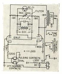
FIG. 6—Dial code sender circuit used in mobile units to unlock repeater station
