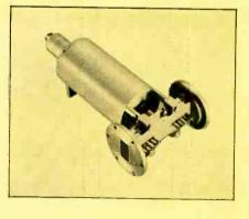
Miniature pulsed magnetrons for missile beacon applications are ruggedly constructed with integral magnets. The RK-7461 is tunable from 9,300 to 9,500 mc and has minimum peak power output of 60 watts. It is 1¼" in diameter and 2½" long, and weighs only 6 ounces.
