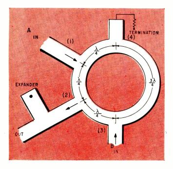
FIG. 2—Logical AND circuit using hybrid ring. Expander (diode in quarter-wave stub) gates output when both input signals are are present. Removal of stub termination at (4) changes circuit to primitive half-adder
