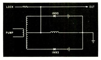
FIG. 5—Phase-locked subharmonic oscillator using lumped parameters. Oscillating parameter is nonlinear capacitance of the two 1N93 diades
