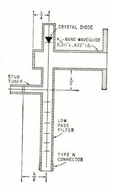
FIG. 1—Multiplier mount dimensions in Ku-band wavelengths
