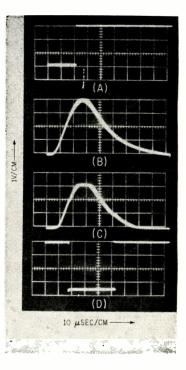
sponse in the blue region to respond to the flash from the crt, yet provide some rejection of white room light. Unfortunately, the only diodes now available are germanium and silicon types, which have peak responses in the infrared region. Early models of the pen used an extremely fast germanium diode.<sup>1</sup> The speed of this diode proved unnecessary for the long (10- to 80- $\mu$ sec) flashes used, so a commercial germanium diode of moderate speed was utilized in later models.
