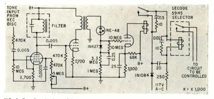
FIG. 5-Decoder circuit used in repeater station with dial lock out
