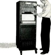
Additional features of the 950-1500 include: common power supply, built-in MOPA, front and rear inputs, easily serviced plug-in circuit cards, adaptability for use with other readout devices. When many channels are constantly in use for floating or grounded high gain inputs the simplified 950-1500 design assures dependable operation, yet at much lower "per channel" cost.
