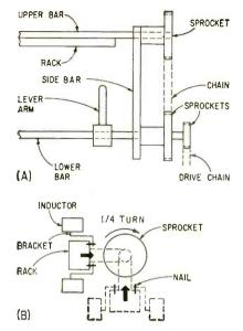
FIG. 3—Rack dips 9 assemblies into encapsulant with 1 motion
