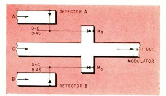
FIG. 4—Diode-waveguide circuit capable of serving as logical AND or OR circuit. Modulator operates as a bridge, reacting to detector outputs. Diode bias is from constant-current source
