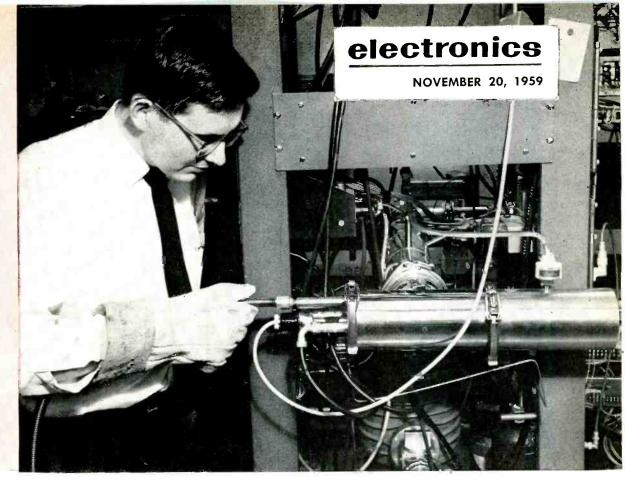
Ammonia maser (being filled with liquid nitrogen) operates in microwave range, uses waveguide as both transmission line and input gate
