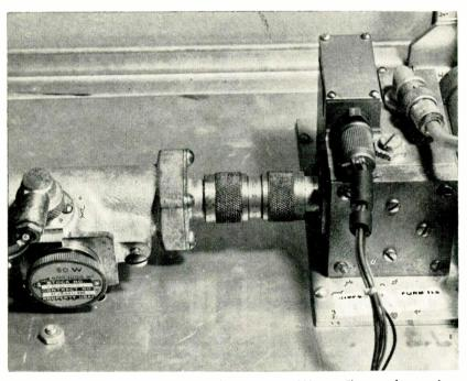
The f-m/c-w radar transmitter operates from 800 to 1,000 mc. The actual transmitter is at the right side of photo
