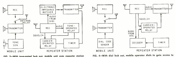
FIG. 3—With tone-gated lock out, mobile unit uses repeater station by transmitting a tone burst which actuates the tone-operated relay allowing carrier control of repeater transmitter
