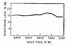
FIG. 2—Second harmonic conversion loss using a 1N78 diode in the mount. Fundamental peak power is equal to 19  $\pm$  3db above one milliwatt
