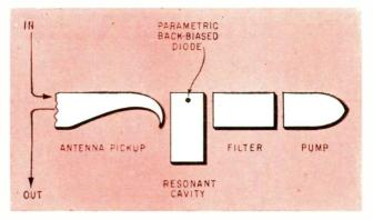
FIG. 6—Microwave version of phase-locked oscillator. Microwave point-contact diode provides oscillating parameter. Filter isolates pump frequency from incoming or outgoing signals
