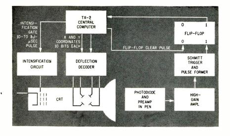
FIG. 1—Simplified block diagram of lightpen system
