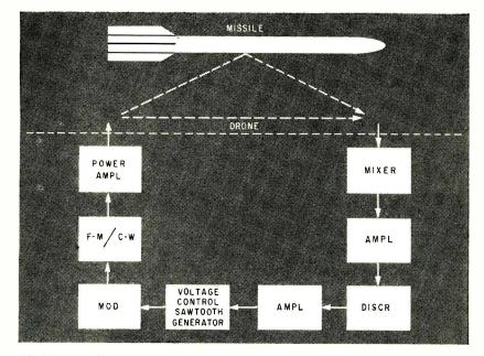
FIG. 1—Sawtooth generator is controlled by error signal developed in the discriminator. Transmitter sweep rate becomes a measure of distance between target and missile
