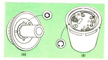
FIG. 1—Knob assembly (A) uses circular self-locking ring to position and lock dial skirt on plastic knob shaft. Push-on type ring is installed without groove, accommodates tolerances of plastic parts to eliminate end play. Portable industrial X-ray unit (B) uses beveled external ring to lock end plate of transformer tube housing
