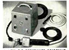
**A NEW G-E RESISTANCE SOLDERING TOOL** provides void-free solder joints for reliable, high-quality connections required by aircraft and missile applications. The new tool eliminates tip arcing or flashing, preventing pitting; is handoperated, requiring no pedals; and features a zirconium-tungsten electrode that does not require frequent redressing, maintenance or replacement. Write for Bulletin GEA-6588.
