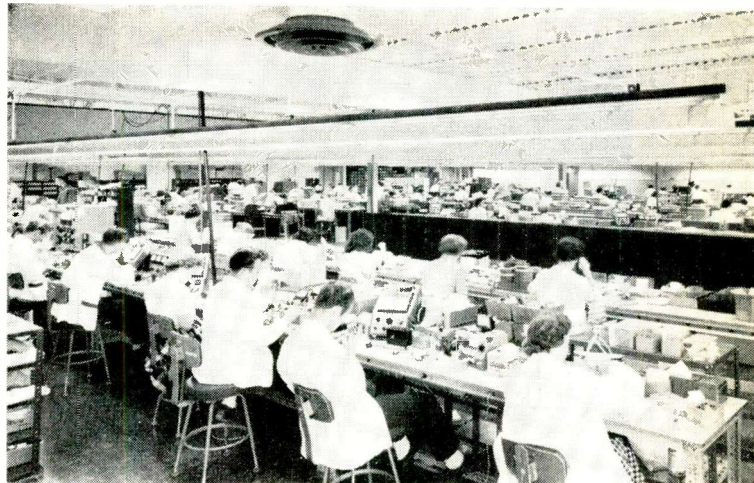
New instrument production area at Assembly Products is pressurized to keep out dust. Area covers 9,600 square feet in plant addition
