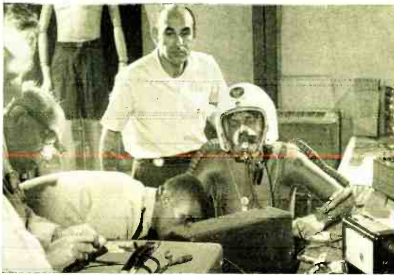
Laboratory testing of sensing devices. Blood pressure sensor is affixed to right index finger of test subject
