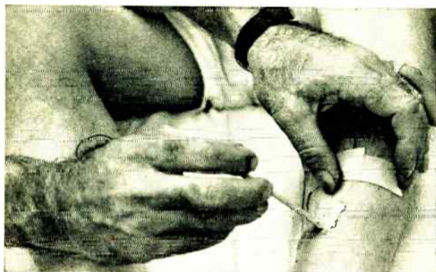
Suspension of silver in collodion forms a light, sturdy, high conductance electrode that can be worn for days without irritation
