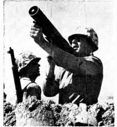
Redeye guided missile is designed to protect ground troops from strafing and bombing
