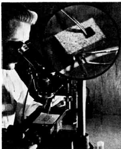
Seen through microscope, tiny Biax has spaced orthogonal holes
