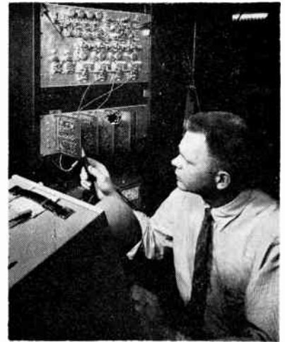
Clock pulse generator is being used to evaluate performance of small subassembly but could be used with synchronized high-speed computing system
