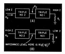
FIG. 4—Cascaded triples with high-impedance output (A); and low-impedance output (B)
