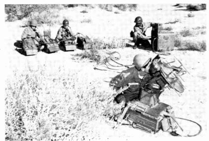
An angular tracker (foreground) is adjusted to pick up signals from Army's Lacrosse surface-to-surface missile as it streaks toward a target 15 miles away. Other equipment shown above in the radio command guidance system includes a power supply unit (right), a computer and a range and direction indicator. Martin is prime contractor
