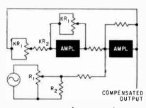
FIG. 5—The general compensation case using operational amplifiers
