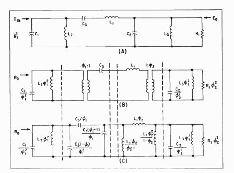
FIG. 1—Triple bandpass filter and equivalent circuits
