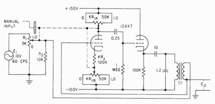
FIG. 2—Practical circuit for error computer reduces loading error 97 percent
