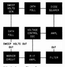
FIG. 2—Output filter of sweep generator sharply attenuates frequencies above and below sweep frequency band
