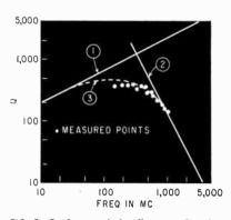
FIG. 5-Q of transmission line as a function of frequency for ideal and actual lines
