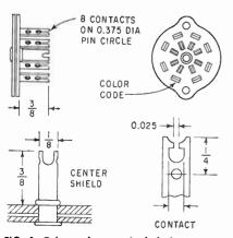
FIG. 1—Tube socket terminal design
