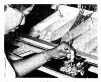
Assembler uses hollow tube tool to weave wire through slots in tube socket terminals
