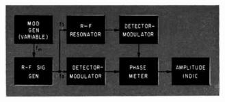
FIG. 1—Test set-up for measurement of resonator Q by observing envelope phase shift
