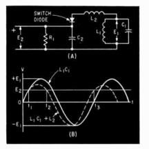
FIG. 1—Fundomentol reoctance-switch modulotor (A) and cycle of operation (B)
