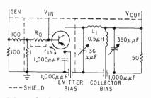
FIG. 2—Sketch shows arrangement of coaxial elements used for measuring  $f_{max}$
