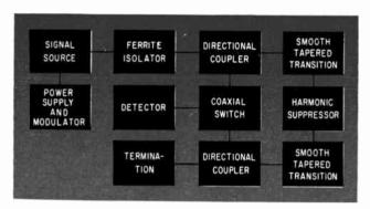
FIG. 3—Low power test setup for measuring effectiveness of spurious frequency suppression
