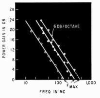
FIG. 7—Power gain characteristics of three graded base transistors in the cutoff region
