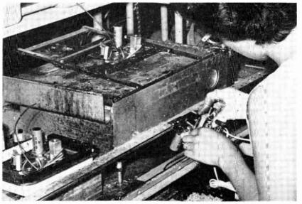
Chassis at lower left is in flux bath. The other chassis is on the cam-eperated jig which lowers terminal tips and wire connections into solder bath
