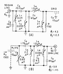
FIG. 3—Transmission from a 90-ohm line to  $10-\mu\mu$ f grid (A); from a  $10-\mu\mu$ f plate to a 90-ohm line (B)
