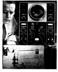
Strain in vibrating beam is plotted against time in upper waveform at same time as beam strain is plotted against acceleration of beam by DuMont dual-beam oscilloscope
