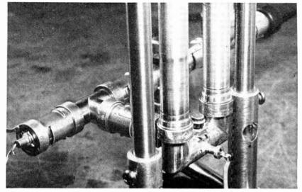
Close-up of coaxial setup shows transistor mount, feedthrough capacitors for emitter and collector bias connections, and detector coupling
