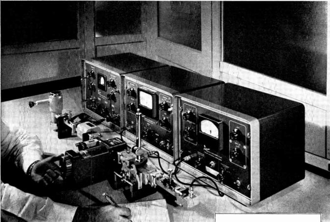
This microwave bench set-up is for the measurement of power by the Self-Balancing Bolometer Bridge method. Other systems, including PRD's more accurate Calorimetric Instrumentation could have been shown, but the Bridge represents the most universally used technique.
