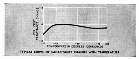
Cera-Mite Capacitors are now available in Formulation 40 from .001 to .02  $\mu$ F, 250, 500 and 1000 volts d-c. Engineering Data Sheets 6106 and 6125 list complete ratings and specifications.
