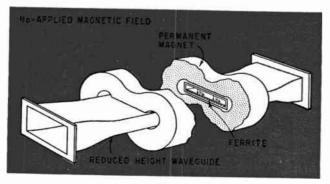
FIG. 2—Method of suppressing unwanted signals in waveguide by use af ferrite slabs magnetized ta resanance
