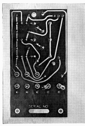
High strength-to-weight ratio. This printed wiring board for a phase failure relay (manufactured by Phase-Guard Co., Carnegie, Pa., and distributed by Stradley Engineering Co., Pittsburgh) was designed with CDF Di-Clad 28E (epoxy resin laminated with medium weave glass cloth) for high mechanical strength, very low moisture-absorption, and good insulation resistance. Details upon request.
