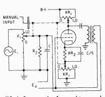
FIG. 4—Compensating for a resistance and capacitance load
