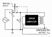
FIG. 1—Loading error is computed and used for compensation
