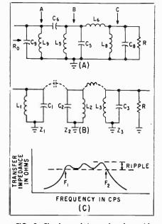
FIG. 2—Circuit used in conjunction with design box (A), triple-tuned bandpass transformer circuit (B) and frequency response of filters (C)
