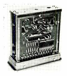
One of the most significant single component developments in building of the computer for the Titan was the use of a sealed chassis. A glass-epoxy copper-clad laminate was chosen for the circuit board material
