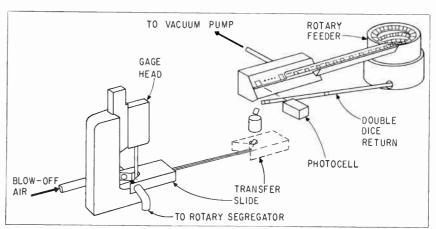
FIG. 1—Basic parts of gaging and sorting mechanism. Vibratory feeder, gravity, camoperated slide and air blew are used to move dice
