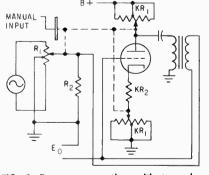
FIG. 3—Error compensation with tapped potentiometers
