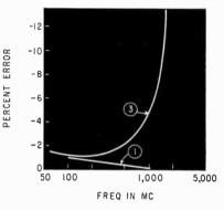
FIG. 6—Error in  $f_{max}$  measurements caused by Q factor in ideal and actual line
