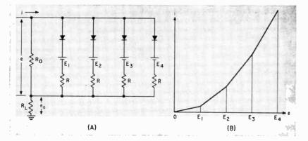
FIG. 4-Fundamental squaring circuit (A) and its operation (B) to produce  $e_0 = ki = k'e^{k}$
