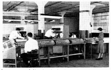
Transacter system gets final inspection at Stromberg Time Corp. factory prior to installation at U.S. Naval Gun Factory, Washington, D.C. Units in foreground gather and instantly transmit information to Compiler (two in background), where it is recorded on punched tape for use of other data-processing equipment
