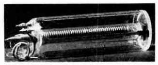
Miniature cryostat, the size of a cigarette, turns nitrogen gas into liquid nitrogen by regenerative cooling
