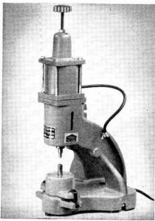
**SHORT RUNS: Electropunch** — sets hand fed terminals twice as fast as conventional methods. All electric. Foct switch operated.
