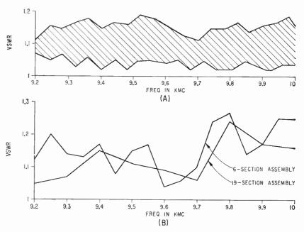
FIG. 2—Frequency in kmc plotted against vswr. Maximum and minimum deviation is given for 40 individual coiled waveguide sections, (A), and for coiled waveguide assemblies, (B)
