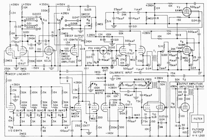
FIG. 3—Oscillator circuit (V<sub>5</sub>) shows how reverse-biased p-n junction voltage-variable capacitor is used to generate a variable-frequency output. Plate voltage of squarer V<sub>3</sub> must be regulated
