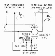
FIG. 2—Hold-off voltage permits warmup to continue until second cam switch closes
