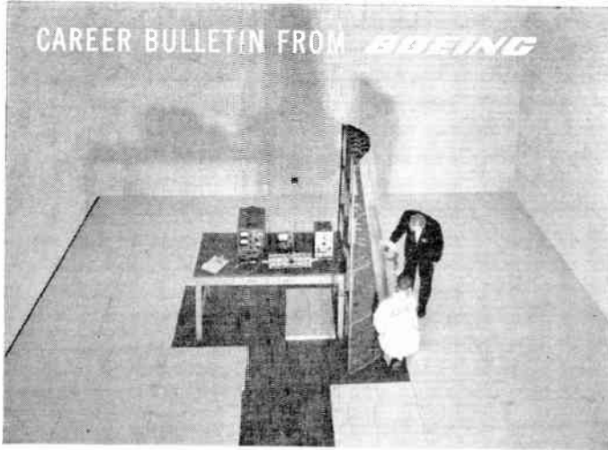
FREE-SPACE ROOM in Boeing antenna and radar laboratory, built for advanced antenna and radome development and testing. Expanding missile and advanced jet aircraft projects at Boeing provide outstanding career opportunities for engineers in virtually every area of electronics.
