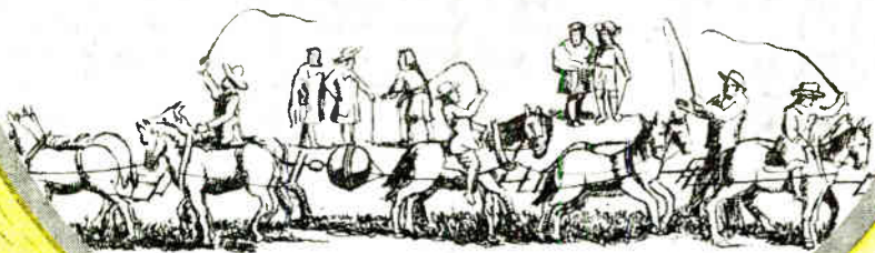
Otto von Guericke's famous experiment with his vacuum or "Magdeburg Hemispheres" which required 16 horses to pull apart during such tests in 1650.
