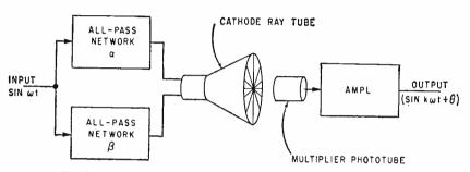
FIG. 5—Cycle-splitter arrangement provides frequency multiplication and digital conversion
