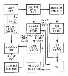
FIG. 1—Two tubes can be added to double integrator to get velocity and distance information for recording
