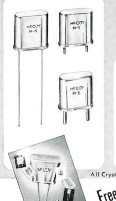
Regardless of size, weight, or shape, a McCoy crystal will deliver the utmost in stability under extreme conditions of shock and vibration. Frequency range of M-1, M-4 and M-5; 200 kc. to 200 mc: M-20, M-21 and M-23; 3.0 mc. to 200 mc.
