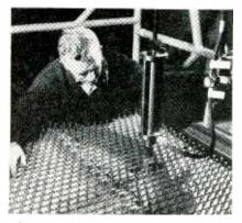
Plastic silver-coated lens developed by Sperry Gyroscope Co. for the Talos missile guidance radar is composed of 4100 cells. The lens is molded of plastic-impregnated fiber glass and coated with silver to make it electrically conductive. Aluminum cores forming the grid structure are molded into lens and then removed with a pneumatic ram
