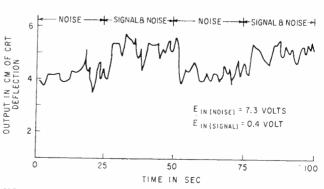
FIG. 4—Experimental waveforms showing actual improvement in signal detectability obtained with crosscorrelator
