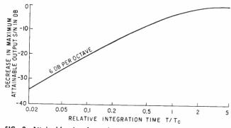
FIG. 3—Attainable signal-to-noise improvement is function of the ratio  $T/T_{\bullet}$
