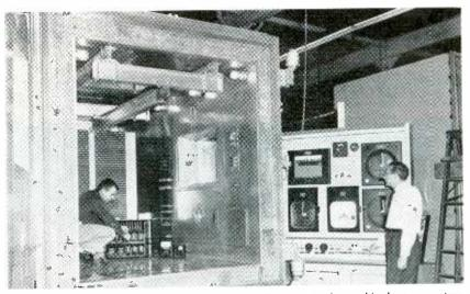
Environmental test chamber used by Army Chemical Corps simulates altitude, temperature and humidity conditions. Chamber was built by Tenney Engineering, control console (right) was manufactured by Bristol
