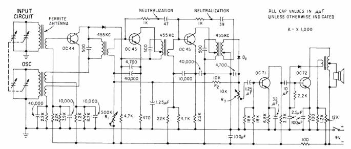
FIG. 4—Typical European broadcast-band receiver, the Peggie portable of Akkord AG
