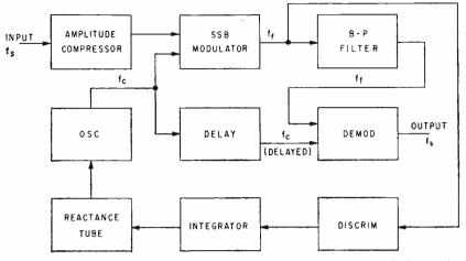
FIG. 3-Automatic tracking filter accommodates wide range of Doppler shift frequencies
