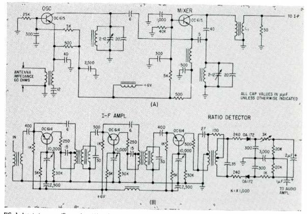
FIG. 1—Input stages, oscillator-mixer (A) and corresponding i-f amplifier (B) of vhf receiver developed by Telefunken, GmbH
