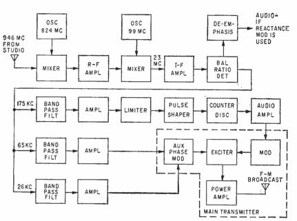
FIG. 2—Mountain-top receiver and main, or broadcast, transmitter. Receiver picks up three programs sent from studio and main transmitter broadcasts them
