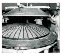
Adhesive on ribs and perimeter readies unit for final assembly
