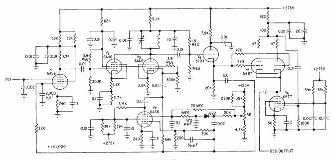
FIG. 4—Schematic of the amplitude-regulated wide-range controlled oscillator
