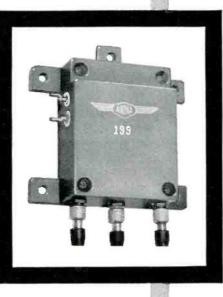
Designed for use in the 100 to 400 megacycle range, the chopper samples two incoming signal sources for a single load or distributes a low level signal to two loads in a periodic manner. Switching frequency is 100 cycles per second.
