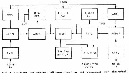
FIG. 5—Simulated two-receiver radiometer used to predictions
