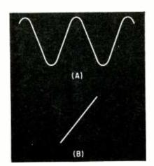
FIG. 6—Compensated amplifier output (A) and transfer characteristic (B)
