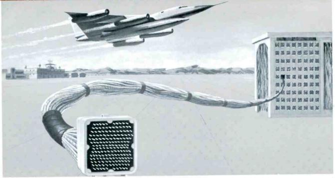
WIRE HARNESS for the navigation system of Convair's B-58 bomber is insulated with Du Pont TFE-fluorocarbon resins for maximum reliability in a high ambient temperature environment. Engineers of the Sperry Gyroscope Company, which developed and is producing the B-58 bomb-navigation system, have also found that
