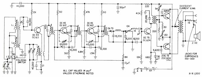
FIG. 5-Combined broadcast and long-wave receiver, developed by Braun GmbH. Sliding contacts are used for switching bands
