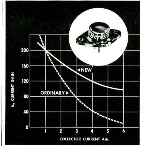
Solid line indicates the low beta fall-off of one of the new Bendix transistors os compared to that of an ordinary transistor.
