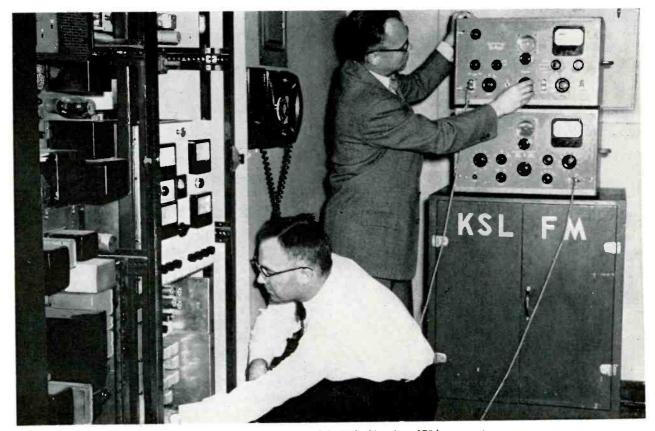
Testing the 175-kc generator of stl transmitter. Engineer at left is looking into 175-kc generator
