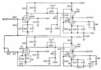
FIG. 7—Wideband driver has low output impedance with balanced output
