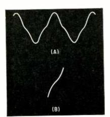
FIG. 5—Uncompensated amplifier output (A) and transfer characteristic (B)
