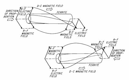
FIG. 1—Direction of rotation for an advancing portion of the wave is clockwise, viewed in the direction of the d-c field irrespective of the direction of wave propagation
