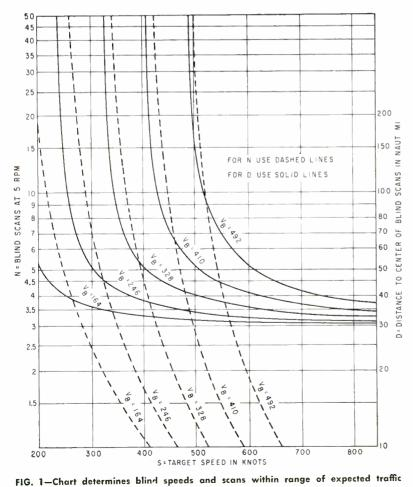
solution of passing course problems. The charts are most useful when it is desired to site radars, analyze evaluation test flights and prescribe aircraft in-flight control criteria.
