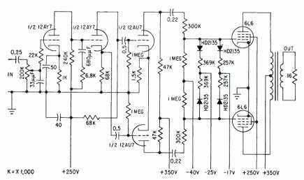
FIG. 4—Compensated amplifier delivers 16 w with 2.6 percent total distortion at 47.6-percent efficiency
