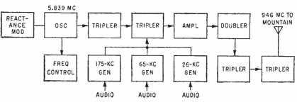
FIG. 1—Studio transmitter. Reactance-tube modulator, formerly used to modulate stl transmitter, now controls oscillator frequency
