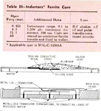
FIG. 1—Preliminary diode and transistor designs
