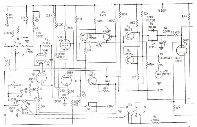
FIG. 1-Log amplifier and period amplifier are completely transistorized. Log diodes, electrometers and catching diode are vacuum tubes. Func-
