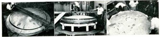
Paraboloid face mold with plastic-topped female templates
