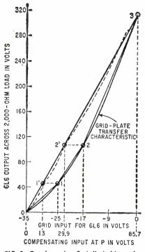
FIG. 2—Graph used to find diode bias voltage and resistors in compensator
