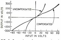
FIG. 3—Comparison of compensated and uncompensated push-pull 6L6 transfer characteristics
