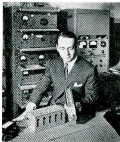
Prime ignition batteries for jet airliners were developed by Sonotone. Firm's president, I. I. Schachtel, inspects unit which weighs only 10 lb, is 2½ in. wide, 4½ in. deep, 14 in. long. Other battery weighs 12 lb, is 4½ in. wide, 4½ in. deep and 10 in. long
