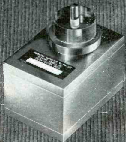
Infrared detection equipment shown here can spot and record concentrations of harmful fumes as low as one part per million
