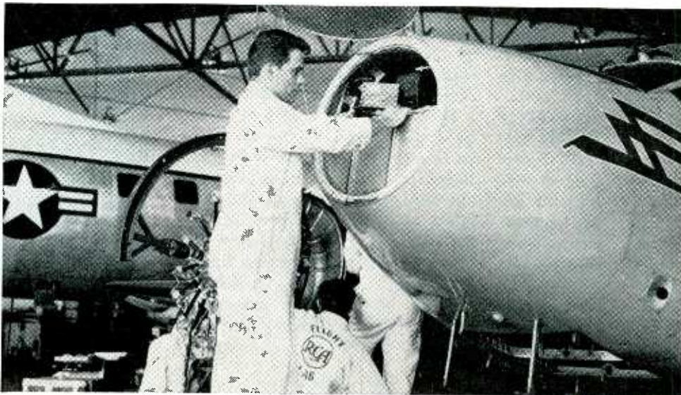
Three-indicator-light adapter is mounted on one-indicator-light receiver to form small, light package
