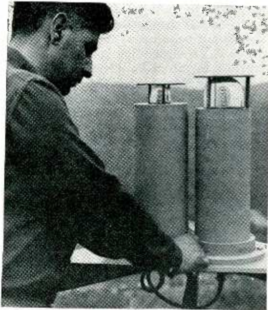
FIG. 1—Output of test unit simulates initial fast rise and subsequent sustained pulse of light flash from nuclear bomb
