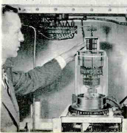
Engineer points out Tung-Sol/Chatham VC1257 installed in Bendix AN/FPS-20 radar equipment.
