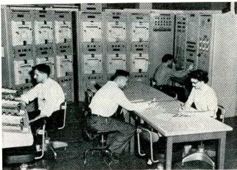
Transonic wind tunnel at Boeing Airplane Co. uses variety of electronic gear to control tests and gather data. At left is analog computer; at center are Leeds & Northrup recorders for recording transducer signals; and at right is automatic programmer to control data gathering, tunnel operation and model position
