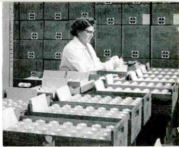
Ready for shipment, these Eimac ceramic tetrodes are just one of more than a hundred different tube types manufactured by Eitel-McCullough, Inc., including negative grid tubes, power amplifier klystrons, reflex klystrons and traveling wave tubes.
