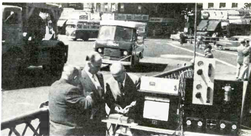
Infrared detection equipment shown here can spot and record concentrations of harmful fumes as low as one part per million
