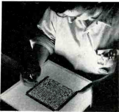
Epoxy board strips around 3 edges of pattern form frame for board blank. Pattern is being checked on light table
