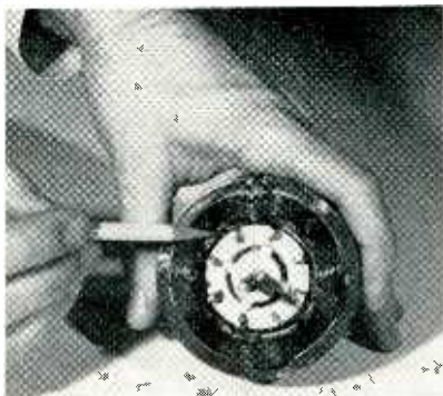
Desired air gap (pencil) is predetermined and motor is built around this dimension
