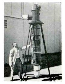
Varian Associates' VA-842 klystron is said to be the world's largest. It's 12-ft high; weighs 900 lb
