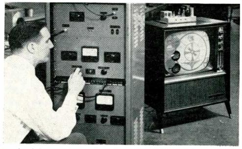
Motorola multiplex transmitter used in closed-circuit test of stereophonic system for television sound
