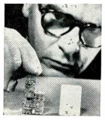
All the electranic parts of this military radia are no bigger than a sugar lump. Receiver is made of micromodules, circuit building blocks developed by Army Signal Research & Development Laboratory and RCA
