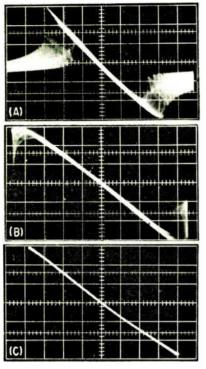
FIG. δ—Performance oscillograms (top to bottom)—signal level to driver, 1.5 mv, 10 mv and 30 mv; f-m, 25 kc at 50 cps, 50 kc at 50 cps and 50 kc at 50 cps; a-m, 30 percent at 400 cps for all three
