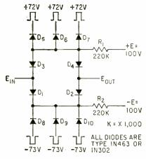
FIG. 2—Schematic of one channel of coincidence circuit using diodes
