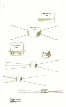
Sprague miniature pulse transformers are ideally suited for application in low-power, high-speed computer circuitry where pulse signals may range up from 20 millimicroseconds and wider in duration, at repetition rates as high as 10 megacycles, with pulse levels ranging from fractions of a volt to several hundred volts.
