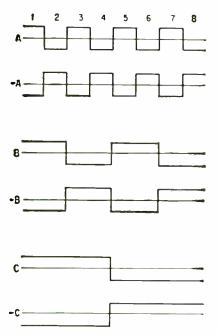
FIG. 1—Waveforms of the three binary switching voltages required to switch 8 channels are periodic with frequencies 4f, 2f and f, respectively
