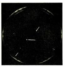
Appearance of markers on ppi scope. Markers along edge indicate direction. Markers with dot and tail represent direction and position of aircraft
