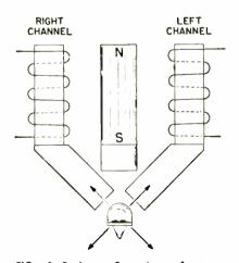
FIG. 1—Basic configuration of stereo pickup design. Magnet is lacated behind plane af the drawing
