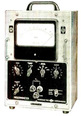
USEFUL RANGE: 1 MEGOHM TO 100 MILLION MEGOHMS 5 TEST VOLTAGES: 50, 100, 200, 500, AND 1000 VOLTS d.c. Meter scale calibrated from 1 to 100 Megohms with 7 range multipliers: x1, x10, ...., x10<sup>6</sup>.
