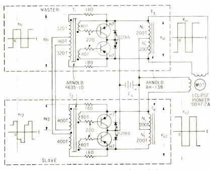
FIG. 1—Two-phase square-wave inverter drives two-phase induction motor
