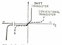
FIG. 2—Zero-bias characteristics for a drift and conventional pnp transistor
