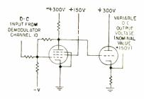
FIG. 4—Compensator for variation of parameters in the transmitting equipment
