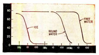
FIG. 3—Dielectric dispersion in ice and water. Curve for bound water explains dispersion of effective dielectric constant of hemoglobin molecules
