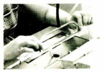
Assembler uses hand vacuum pickup to hold electrodes
