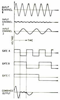
FIG. 3—Waveforms show how binary voltages gate switch for three input signals. When gates A, B and C are positive, channel 1 is closed. Channel 2 conducts when A reverses polarity. All possible logical combinations result in eight channels
