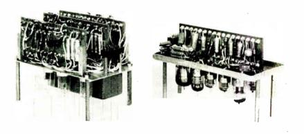
Pulse-position demodulator (left) ond decommutator (right) are packaged in modulor form to facilitate plug-in use
