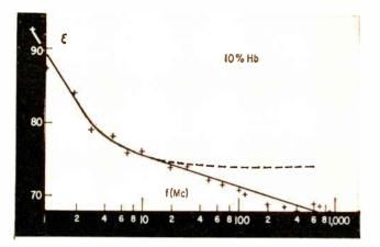
FIG. 2—Dielectric dispersion of 10-percent hemoglobin solution in water. Dashed curve indicates theoretically predicted behavior; points are empirically derived
