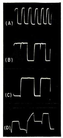
FIG. 6—Oscillograms of gating voltages for six channel switch are shown in (A), (B) and (C) while (D) shows switch output with input from marker generator
