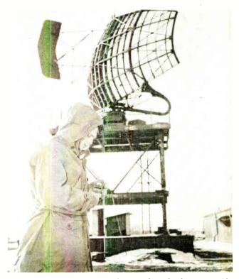
Richardson dosimeter measures heat analog of r-f energy, with blob of gelotin as transducer
