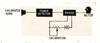
FIG. 4—Black diagram of Sperry Gyroscope microwave power-density meter. Meter reads directly in  $mw/cm^2$  and in db relative to 0.01  $w/cm^2$
