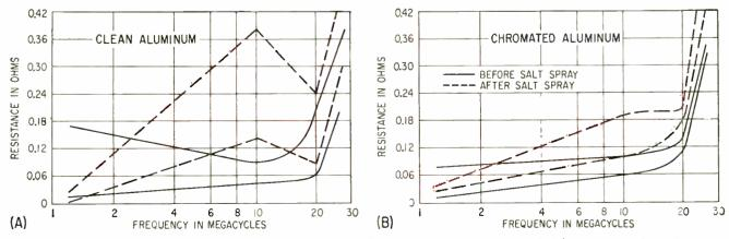
FIG. 1—R-f resistance of aluminum. Maximums and minimums before salt spray exposure are shown by black lines. Ranges after 64-hour salt spray are shown by red shading
