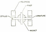
FIG. 3-Simplified bottom view of pickup
