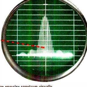
Dissect complex pulse spectrum visually by means of Polarad Model SD-1
