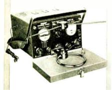
This improved instrument is a compact, rugged and highly sensitive interference locatorwith the widest frequency range of any standard available unit.
