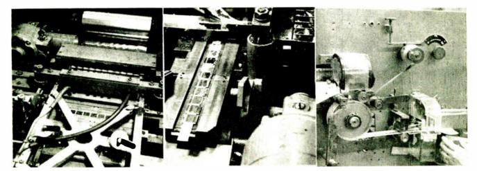
Electrode pickup and foil slitting roller die
