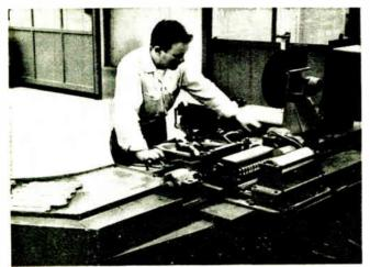
Ribbons of glass and foil electrodes are interleaved automatically an compact machine
