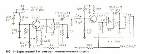
**D**<sup>ESIGN</sup> of a transistorized tv receiver requires an efficient, low-cost sound strip. The circuitry described uses an efficient, highly sensitive oscillating linearslope detector, injection locked by a one-stage sound driver. The combination of sound driver and detector is capable of overdriving the output audio amplifier when driven from the first video amplifier,
