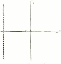
FIG. 2—Pole-zero diagram of one-stage amplifier using 2N384 transistor
