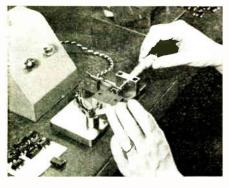
Every Milli-Switch is checked for pre-travel and over-travel. Maximum allowable pre-travel is onethird of that in most other switches.
