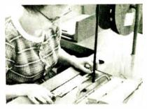
Stacking capacitor strip by hand
