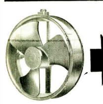
The Saucer Fan represents an entirely new design concept whereby the driving motor is built within the propeller hub limiting its axial length to the minimum measurement required by a highly efficient motor. Ideally suited for tightly packed electronic packages, where space is critical, the Saucer Fan will provide cooling air to the amount of 280 cfm. Power requirement is 115 vac. 50-60 cps, 1 Ø.
