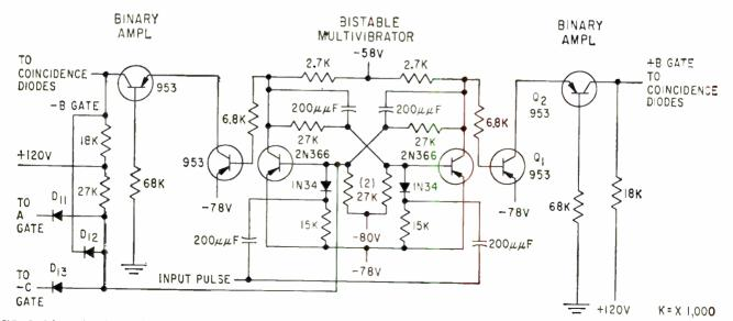
FIG. 5—Schematic of one channel of the six-channel switch. Forced recycling of the switch through diodes D<sub>11</sub>, D<sub>12</sub> and D<sub>13</sub> triggers switch back to channel 1 after channel 6 is reached
