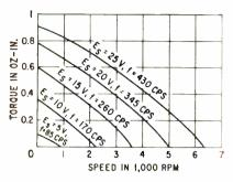
FIG. 2-Measured torque as a function of speed for driven inverter servo motor. Supply voltage Es sets inverter frequency and determines motor speed and torque
