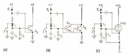
FIG. 5—Emitter follower used for bootstrap sweep circuit (A); composite emitter follower for high input impedance (3); and electron-tube version which covers larger temperature range
