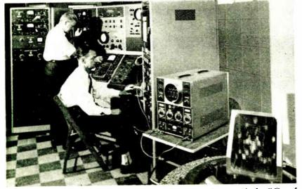
U. S. Army Signal Research and Development Laboratory engineers study feasibility of random vibration test system for evaluating components for future space vehicles. Du Mont dual-beam oscilloscope provides visual indication to pinpoint instant random noise frequencies begin to affect component's structure. Shaker at right is operated from taperecorded random noise
