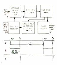
FIG. 2—Simplified black diagram of telemetry transmitting system
