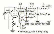
FIG. 4—Lumped-constant technique was used in designing vhf oscillator that deliveres about 10 mw into 50 ohms
