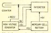
FIG. 1—Counter produces pulses whose rate of occurrence is proportional to radiation intensity of contaminated area
