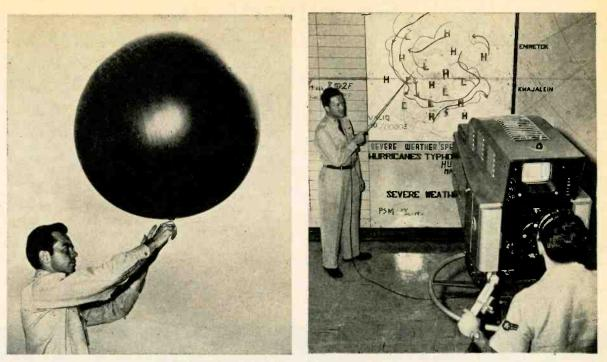
Radiosondes (left) gather weather data at some 8,500 stations. Color tv camera in SAC's global weather central gives world-wide weather picture to rest of underground control center
