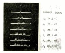
FIG. 8—Deviation of 110-kc sine-wave modulating signal is shown as a function of amplitude with 46-mc carrier and 50volt bias
