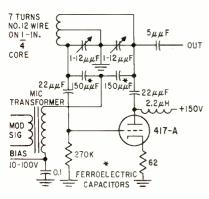
FIG. 5—F-m oscillator uses ferroelectric capacitors for tuning as well as for modulating
