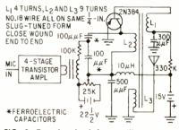
FIG. 9—Transistorized f-m oscillator operates in 50-mc range
