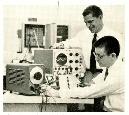
Engineers demonstrate the low-drift d-c differential amplifier. Output of amplifier is visable on the oscilloscope screen
