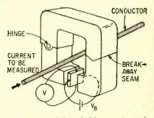
Some type of box holds sample and magnet pieces together. Device becomes wattmeter if voltage across conductors is used in place of  $V_{IP}$
