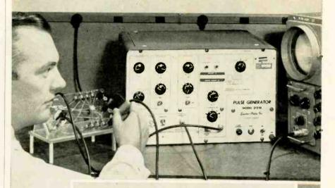
Evaluating a Magnetic Core at Hughes Aircraft Co. — with the Electro-Pulse, Inc. Model 21258 PHOTOGRAPH COURTESY HUGHES AIRCRAFT CO.
