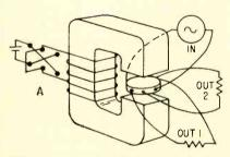
Position of switch A determines whether input is transmitted to output No. 1 or 2
