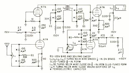
FIG. 10—Tuned stages of panoramic receiver are packaged plug-in units covering 35 to 70, 70 to 130 and 130 to 200 mc
