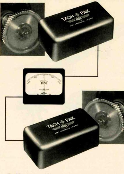
The difference in speed between two rotating shafts is accurately sensed and indicated on a center-zero meter. Even slight variations are instantly transmitted to the indicator. The proximity magnetic pickups used with the system do not impede shaft rotation. Shaft speeds may be adjusted manually or, if a closed servo loop is used, a predetermined rotational speed difference may be maintained automatically.
