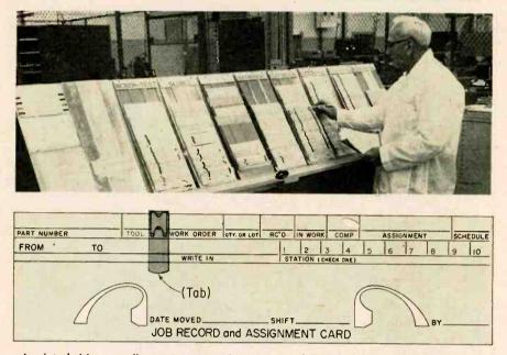
Lead technician coordinates test operations at control board, keeping job records and assignments listed on cards like the copy shown
