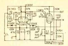
FIG. 2—When switch S<sub>1</sub> is closed, gate is opened. Negative-going trailing edge of pulse closes gate again
