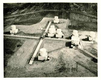
Azusa, developed by Convair, is a highly accurate c-w phase-comparison system. Antenna array measures angle cosines
