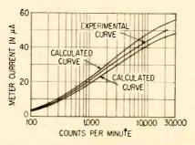
FIG. 4—Metering circuit calibration curves. Two calculated curves apply to extreme limits of the adjustment for R<sub>7</sub>
