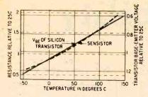
FIG. 3—Temperature charactivistics of silicon resistor element, used to compensate for thermal variation due to  $V_{he}$
