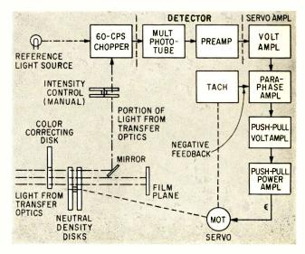
FIG. 2-ROTI automatic exposure control
