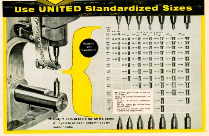
Only SEVEN sets of tools needed for all 65 sizes! This means that tooling is reduced as much as 90%. With United's closely co-ordinated system of Standardized Eyelets and Eyeleting machines, eyelet grip can be increased as much as 1000% (for instance, from .093" to .437") without a single change in drill, punch, or setting tool. Result: greatly reduced installed costs and true fastener economy.
