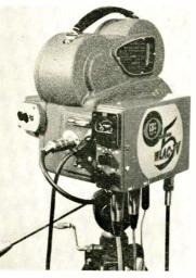
Transistor amplifier is mounted on camera
