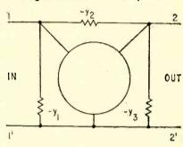
For amplifier to isolate,  $y_1$ ,  $y_2$  and  $y_3$ must have precise values
