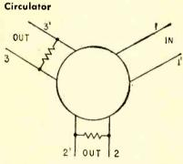
Load resistances must be of proper valnes for device to circulate. May be used with parallel resistances
