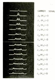
FIG. 7—Bessel function plot shows 40-kc sine-wave modulating frequency with amplitude varied to obtain indicated roots. Carrier is 46 mc and bias is 50 volts
