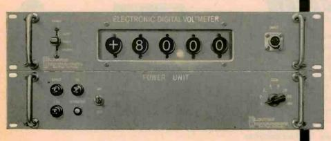
Both the 7000 and 8000 Series develop voltage state BCD outputs for data recorder entry. Standard code is 2, 4, 2, 1; other codes available on special order.
