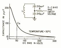
FIG. 1—Ferroelectric capacitors are connected in parallel with bias and sweep voltages but in series with r-f voltage to keep low r-f field across each capacitor. Plot shows capacitance against bias voltage with C<sub>0</sub> the operating point
