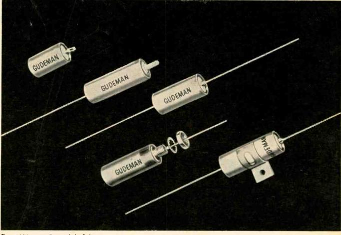
These miniature capacitors made by Gudeman Company for filter, by-pass and blocking service, are impregnated with silicone fluids to decrease electrical losses and increase permissible operating temperatures. Designed to meet all specifications of characteristic "K" MIL-C-25A, they have an operating temperature range of --55 to 125 C.
