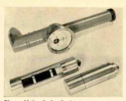
Disassembled probe handle showing case and meter (top), high-voltage generator and ratemeter circuit board (bottom, left) and battery housing (right)
