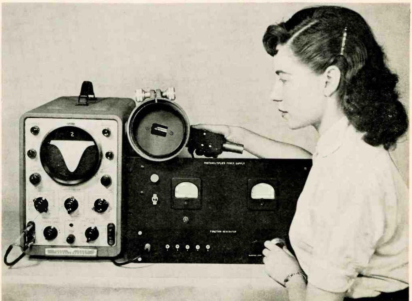
Bench setup illustrates use of component parts that make up photoelectric function generator
