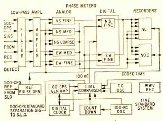
FIG. 4—Entire equipment at each receiving station
