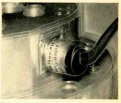
Typical M Series Gyro undergoes 20 G Linear Vibration Test with no deterioration of performance.
