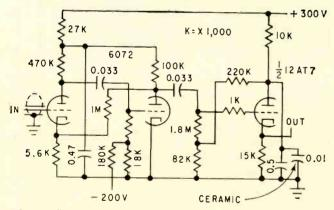
FIG. 6-Buffer circuit of the tracking system
