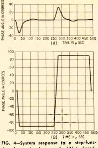
tion change in phase angle; (A) is closedloop, (B) open-loop response
