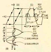
FIG. 3—Graphical analysis shows that only *I* component can be produced because reference signal saturates core except during time  $\triangle T$
