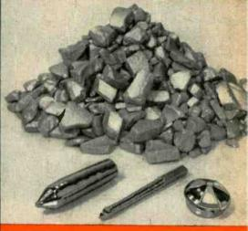
Three characterization crystals are grown from each lot — one for resistivity, type and lifetime determination; another for cleanliness; a third for boron content.
