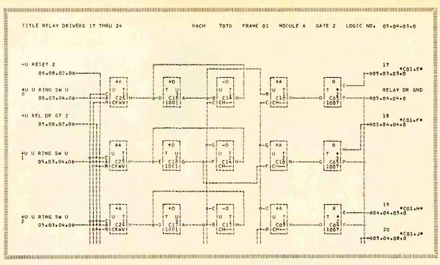
From an engineer's rough logic sketch, IBM computer produces a finished drawing. Diamonds are connection points
