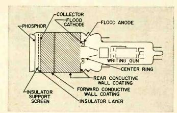
FIG. 1-Schematic diagram of 2.5-in. latron with symmetrical guns
