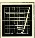
PIGH COLLECTOR CU2RENT PNP transistor, collector current vs collector valtage with constant-current base steps. Collector sweep is 0 to 5 v with a 0 25-ohm load, base current is 50 ma/step. Vertical deflection is 100 ma/div, horizontal 0.5 v/div.
