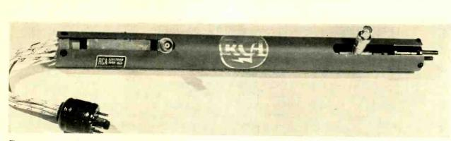
Closeup view of packaged traveling-wave device
