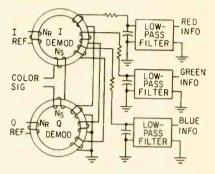
FIG. 4—Complete system shows core outputs integrated and filtered to produce red, green and blue information
