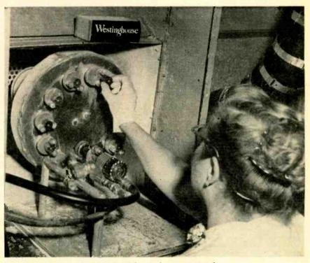
Magnetic chucks speed loading of nickel cathodes on rotating fixture
