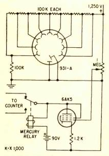
FIG. 3—Multiplier-phototube control circuit. The mercury relay controls the electronic counter
