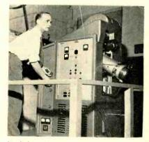
Single-barrel projector displays pictures in Swiss-made system
