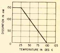
FIG. 1—Typical derating curve for TI 2N559 transistor
