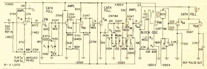
FIG. 7—Reference-pulse generator supplies a 500-cps reference pulse to the analog and digital phase meters
