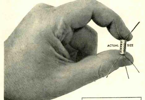
The Airpax Type 6000 Transistor Chopper performs a switching operation over a frequency range of 0 (DC) to 100 KC with signal levels from a fraction of a millivolt to 5 volts.
