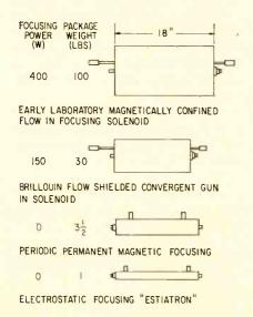
FIG. 1—Size and weight comparison for 10-w S-band traveling-wave amplifiers **B**ECAUSE of its large bandwidth and gain, the traveling-wave tube is useful in radio-relay systems requiring frequency diversification.
