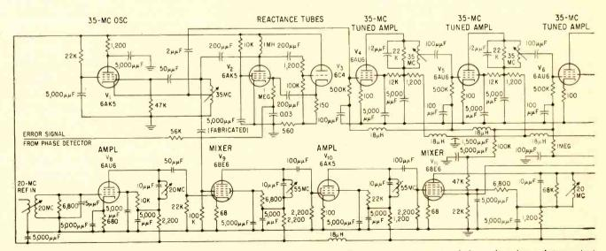
FIG. 3—Schematic diagram of the phase-shifting circuit used in the phase-stabilized system. Error signal from the phase detector (not through reactance tubes V₂ and V₃. Output of fixed-tuned stages V₄ through V7 is shifted as a function of the d-c error signal
