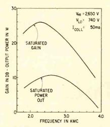
FIG. 5—Saturated gain and power output as a function of frequency. Voltages held fixed at optimum values for 3 kmc
