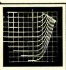
HIGH INPUT CURRENT PNP transistar, collector current vs collector voltage with base graunded and constant-current emitter steps. Collector sweep is 0 to 1.5 v, emitter current 200 ma/step. Vertical deflection is 200 ma/div, horizantal 0.1 v/div. Zera voltage is a center scale.
