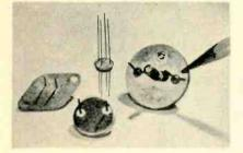
Power transistor bases show how leads are sealed directly to copper base without need for metal eyelets
