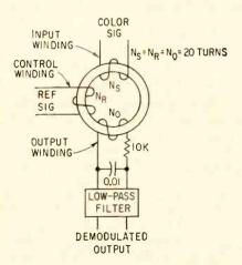
FIG. 1—Basic magnetic demodulator has input winding with color information, reference winding and output winding that supplies demodulated 1 or Q information Fig. 1. Mixing takes place in the ferromagnetic toroid, whose actual and idealized hysteresis loops are shown in Fig. 2. A graphical analysis of the basic operation is shown in Fig. 3. The idealized hysteresis loop of Fig. 2 is used in Fig. 3A.
