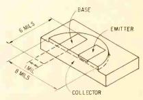
FIG. 3—Closeup of diffused-base germanium wafer
