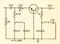
FIG. 2—Capacitor C of transistor circuit to be measured must be increased in valve for frequencies below 1 mc
