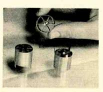
Type of cathode sprayed on inside surfaces
