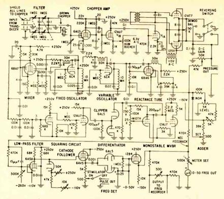
FIG. 5—Complete circuit diagrom of blood pressure regulator. Power supplies are conventional, hence not shown
