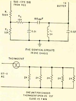
FIG. 5—Schematic of narrow-passband filter
