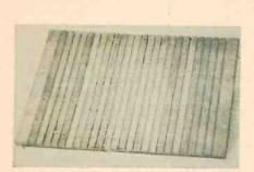
Board holder is pine strips nailed on plywood
