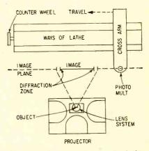
FIG. 2—Mechanical arrangement of the precision measuring machine. Image of object to be measured is scanned by phototube as arm travels down lathe
