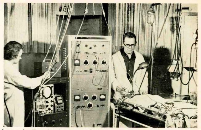
Prototype regulator, filling standard rack at center, successfully held blood pressure and pulse rate of dog on table at desired levels set on dials. Clamps on table hold pressure transducer that goes in artery and electrodes that make contact with nerves
