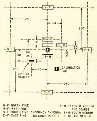
FIG. 1—Antenna field layout at each of eleven ground receiving stations located at widely scattered points on earth. Signal-phase comparisons are made from antenna pairs that lie in north-south and east-west directions
