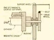
FIG. 1—Cutaway view of chuck and drive wheel assembly
