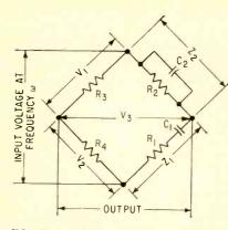
FIG. 1—Basic Wien bridge is balanced when  $V_3 \equiv 0$
