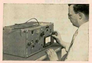
The RX Meter measures the characteristic impedance, attenuation and propagation velocity of RG-58/U Cable.
