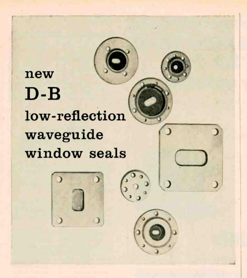
These rugged hermetic seals pass microwave energy with minimum reflection loss. Soldered directly to the waveguide flange, they seal out moisture, dust, oil, and salt spray—or maintain constant pressure or constant dielectric inside.
