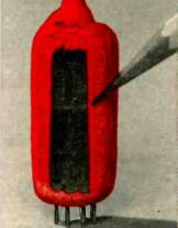
Electronic tube encapsulated with Silastic.
