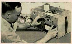
Dynamic measurement of a junction transistor under conditions of variable bias and applied RF. Similar procedures can be used with vacuum tubes.
