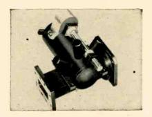
ance equalling that of a two-section filter. Tuning range covered is 8,500 to 9,600 mc, with an insertion loss of less than 1.0 db and a vswr of less than 1.20. Bandwidth to the 3db points is approximately 20 mc at midband. Rejection obtained at  $F_o \pm 60$  mc is greater than 27 db. Circle 300 on Reader Service Card.
