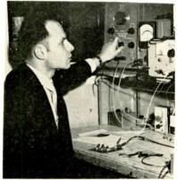
Checking the gain of amplifier-limiter
