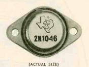
NEW TI 2N1046 combines high power, high frequency and high voltage performance in a single transistor package! This P-N-P diffused base germanium transistor has guaranteed dissipation to 15 watts and collector breakdown voltage to 80 volts with 12 mc typical alpha cutoff. Extremely low collector reverse current averaging 0.2 ma at 40 volts and a low 0.75 ohm saturation resistance assure reliable operating characteristics.
