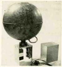
Complete ion chamber assembly. Copper-plated steel sphere is filled with pure argon at 100 psi
