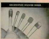
Ratings: 20 to 160 volts . 100ma to 11 ma. Ideal components for bias supplies, sensitive relays, computers etc. High resistance, (10 megohms and higher at -10 volts). Excellent linear forward characteristics. Extremely small, low in cost. Encapsulated to resist adverse environmental extremes. Specify Bullatin 5D-18.
