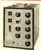
VR-607 Precision Voltage Reference Source. Certified standard cells, oil.immersed ultrastable resistors and high-gain chopper-stabilized amplifiers ensure 0.01% absolute occuracy. ±111.112 volts d.c range . . . 0.1 millivolts resolution down to zero volts . . . 0.05% stability. Bulletin 95806
