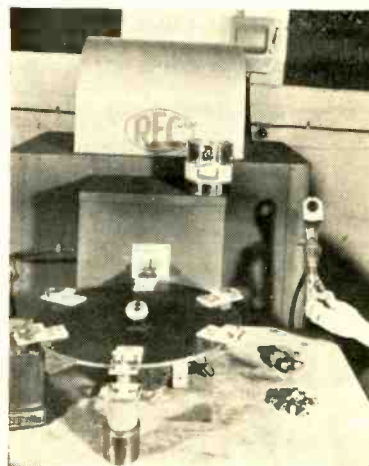
Meter magnet assembly setup. Turntable moves counter-clockwise
