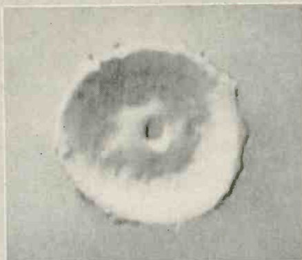
Electron micrograph of impact produced on aluminum coated glass by a 1 micron diameter particle traveling at 7,000 feet per second.
