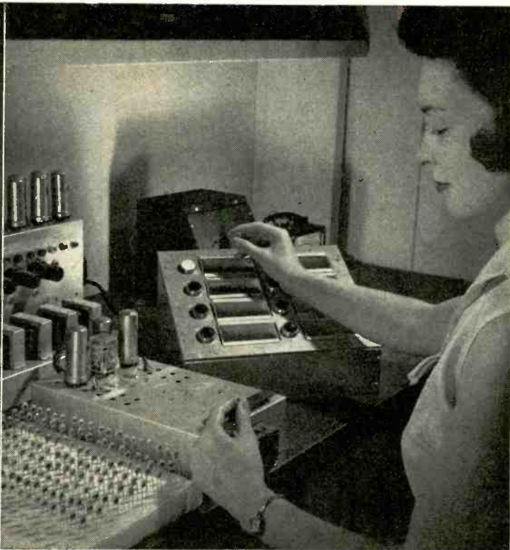
Mallory-designed and built automatic classification equipment is used for 100% testing of silicon rectifier production—insuring high quality and reliability at low cost.
