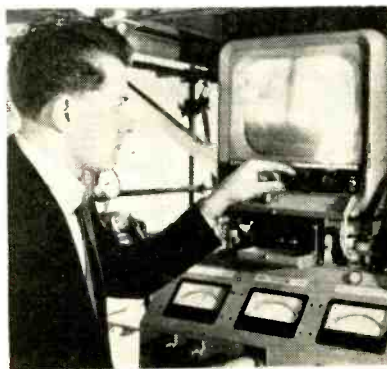
Derrick heads controls show how tv (left) guides mechanical hand in grabbing radioactive cartridges as . . .
