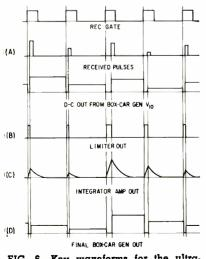
FIG. 6-Key waveforms for the ultrasonic equipment
