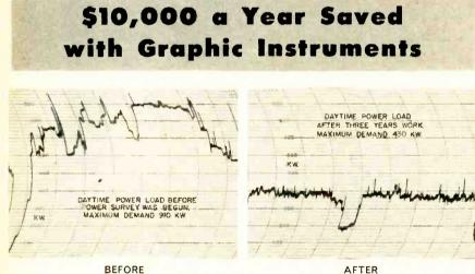
Power Savings of \$10,000 a year were made, as the result of a power survey, at the same time that output increased 25%. You too can make similar savings in your plant.
