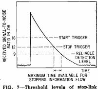
trigger are based on known maximum fade rate of meteor burst
