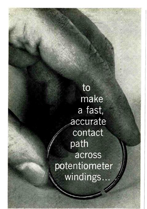
Cut potentiometer contact paths 6 to 10 times FASTER with the S.S.WHITE Airbrasive Unit. It gas-propels a fine stream of abrasives to give fast, uniform, perfectly controlled cutting action. The cutting action will not affect even the finest wires...or create heat to damage wires or surrounding varnish. Cuts lines as fine as .008"! For more information about this amazing new industrial tool, ask for Bulletin 5705A.
