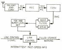
FIG. 1—Overall block diagram of meteor-burst communications system shows signal path for the detection and control of transmission, as radio waves bounce from ionized meteor trail. Information is transmitted only during meteor-burst
