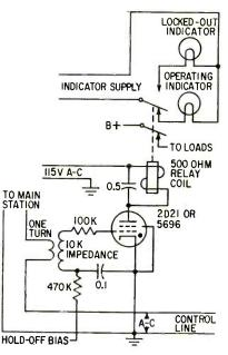
FIG. 3—Current transformer in control line locks out overridden station in system with any number of stations
