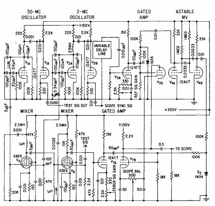
FIG. 4—Free-running multivibrator output is R-C coupled to grids of gated amplifiers  $V_{\rm 3B}$  and  $V_{\rm 7B}$ . Output of  $V_{\rm 7B}$  is a composite signal
