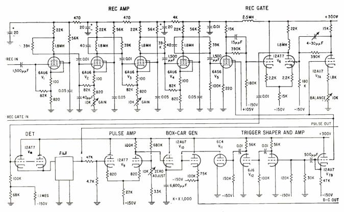
FIG. 5—Complete circuits for one of the receivers. The second receiver is similar in design
