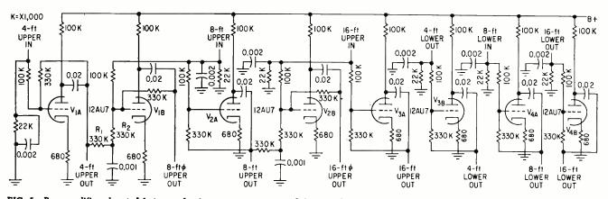
FIG. 5—Bus amplifiers located between keying-system outputs and formant filters provide outphased signals  $\phi$  that lack even-harmonic content. Combinations of these produce the tone colors called for by the voicing panel
