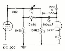
FIG. 7—Swell shoe operates capacitive volume control  $C_1$  that replaces expensive industrial-type potentiometer
