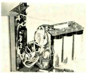
FIG. 1—Power unit by American Speedlight Ascorlight uses symmetrical inverter circuit. Thyratron trigger tube limits shutter con-
