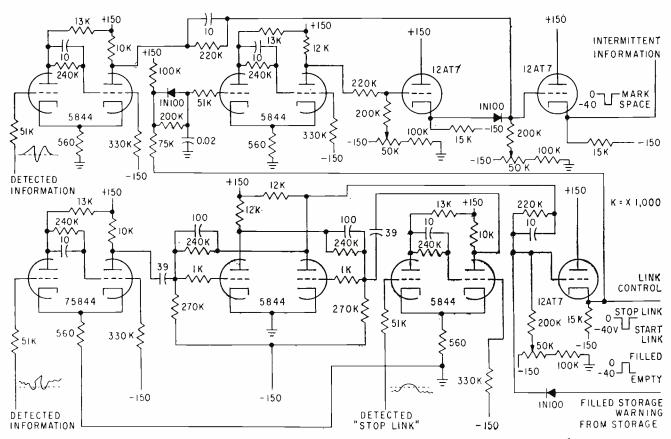
FIG. 6-Link-control schematic. Triggers are set well above ambient noise to preclude false triggering by noise spikes
