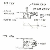
FIG. 4-Electromagnetic fields for tube
