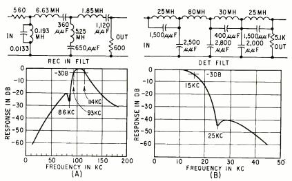
FIG. 4—Receiver input filter design and response (A) and detector filter design and response (B)
