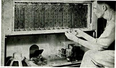
THE FRONT COVER—Engineer installs removable printed-circut modules in electronic organ. Modules include tone generators, voicing panel and amplifier
