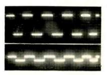
FIG. 2—Collector-to-collector (top) and base-to-base (bottom) voltage waveforms for circuit of Fig. 1
