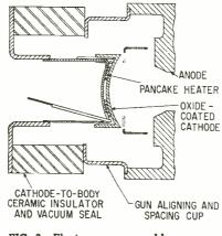
FIG. 2-Electron-gun assembly
