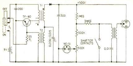
FIG. 4—Single power transistor is used in Burleich Brooks Mecablitz 100 modified blocking-oscillator circuit. Half-wave rectifier requires higher voltage step-up by  $T_1$
