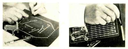
Coating is stripped from plastic film to produce photo-etch negative
