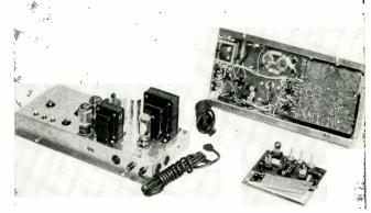
Voicing panel contains all filter components plus stop switches operated by plastic stop tablets shown at left
