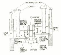
FIG. 1-Sectional view of klystron
