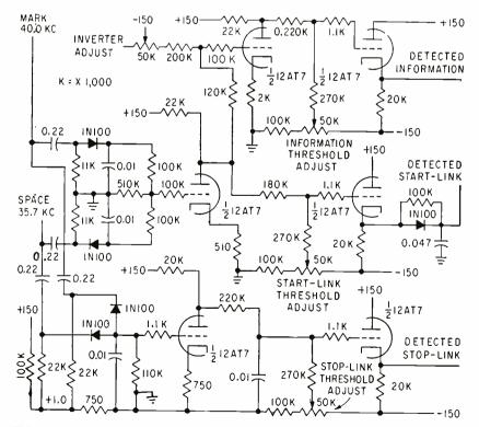
FIG. 4—Detector circuitry. Rapid response start-stop signals use minimum burst time
