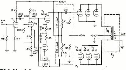
FIG. 3—Schematic diagram of the transmitter
