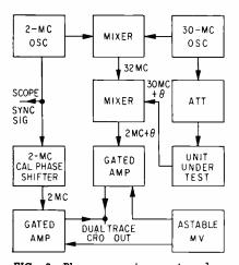
FIG. 2—Phase-measuring system has two mixers that brings 30-mc input down to 2 mc
