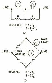
FIG. 4—Lamp failure in circuits at A and B does not stop current flow, and circuit at B also indicates lamp failure
