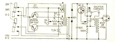
FIG. 3—Inverter transistors are used as rectifiers when charging integral nickelcadmium cells in Romal Electric's Vanguard supply
