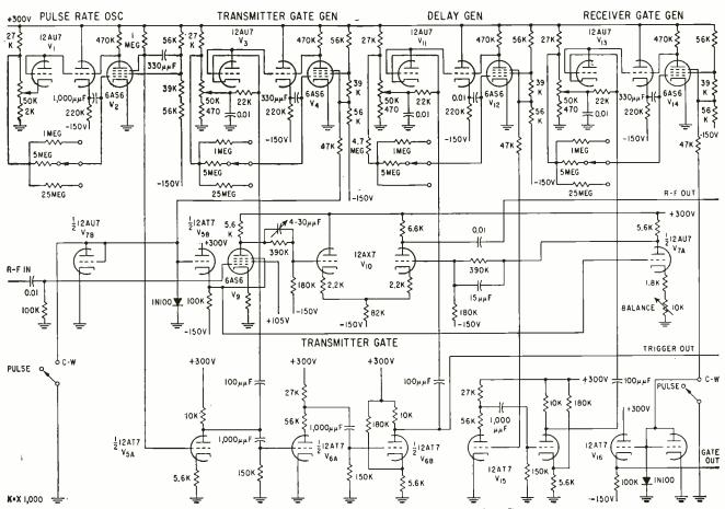
FIG. 2—Trigger and gate generator circuits used in equipment measuring propagation under the sea
