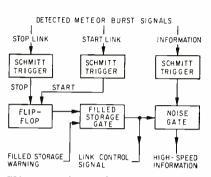
FIG. 5—Link-control block diagram. Start and stop links are regenerated by Schmitt trigger circuits
