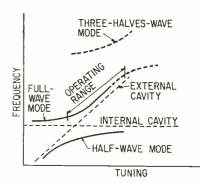
FIG. 3—Tuning curves for tightly coupled double-tuned cavity
