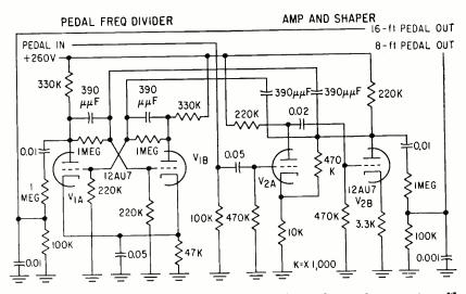
FIG. 4—Pedal generator produces notes an octave lower than main generator with the use of bistable multivibrator  $m{V}_1$
