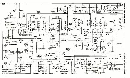
FIG. 6—Voicing panel contains formant filters which transform sawtooth-generator signals into waveforms of various instruments
