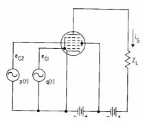
FIG. 1—Output of pentagrid mixer is a nonlinear function of its two inputs
