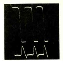
FIG. 5—Collector (top) and emitter (bottom) voltages for circuit of Fig. 4
