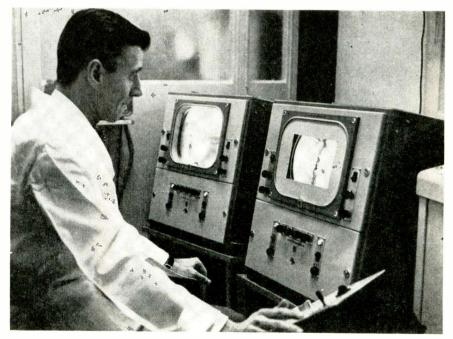
Peristaltic movement of a patient's intestine is viewed by doctors eight miles away in a Montreal hospital. Closed-circuit or transmitted tv pictures of x-ray images used with a Philips intensifier permit consultants to diagnose human ills without being on the spot
