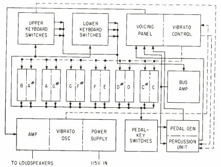
FIG. 1—Each main block in organ block diagram is a removable module with two tone generators on each of six tone modules
