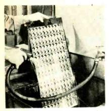
Sheet of name plates is rinsed after unexposed areas are etched off
