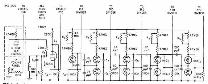
FIG. 3—Complete tone generator for one series of octavely related tones has master oscillator that provides initial sync for neon-lamp divider chain. Resistor  $R_1$  varies from unit to unit and maintains oscillator Q within common range
