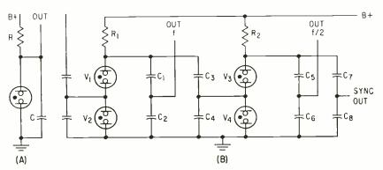
FIG. 2—Standard neon relaxation oscillator (A) is modified (B) so that series lamps have high-impedance point between lamps for sync injection
