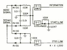
FIG. 3—Simplified schematic of burst detector. The start-link channel indicates when the incoming signal exceeds a usable threshold
