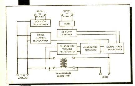
The Ratiometer consists of two precision variable transformers, a calibrated quadrature injector, a filter, and a pre-amplifier. Block diagram indicates connections of the various components ACCURACY ± (0.0005% + 0.0001%/ratio FREQUENCY RANGE 25 cps to 2,500 cps MAXIMUM VOLTAGE Twice the frequency in cps, or 250V, whichever is lower. PRICE Model 214 Rotiometer, complete with 400 cps plug-in filter ond quodrature units
