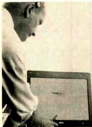
Control tower operator (left)—his vision blocked by hangar—uses remote camera to check runway activity
