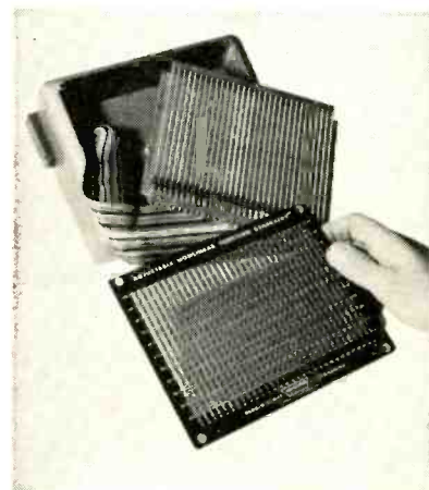
Panel contains 31 sliders each of which may be adjusted to 101 positions
