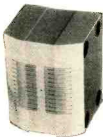
REDUNDANT —Close-spaced record-reproduce head speeds data processing by reading and checking tape immediately after recording. Reduces necessary equipment and power for checking register.
