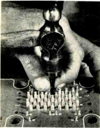
When hydraulic press is used (left) anvil is fixed on moving ram and die is on press base. Positions are reversed in hand method as hammer is used to strike die
