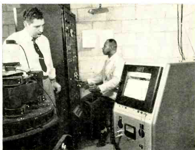
In this Barry Controls setup, ratio of signals from two a-c transducers at left is plotted on recorder at right for a permanent record of vibration transmissibility
