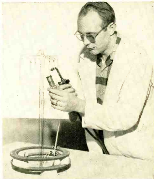
Technician seals off an InSb detector from the vacuum pumping equipment prior to testing characteristics
