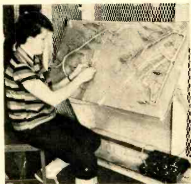
Step-by-step instructions from sender (lower right) go to hearing-aid receiver to teach worker complicated tasks
