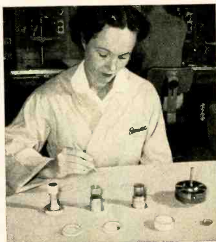
Assembling parts of Eimac, high-gain, amplifier tube. Nickel provides rugged structural support, helps assure electrical stability.
