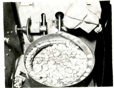
Photocell triggers feed system on disk tester
