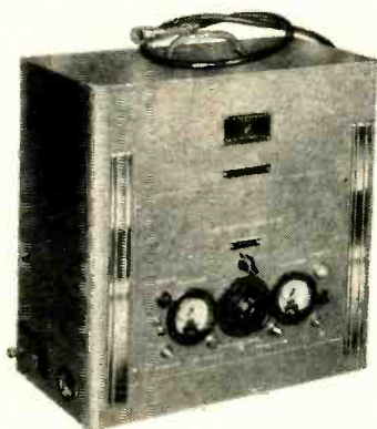
200 Series, Portable Light-weight, easily carried, air-insulated. Output from 0 to 30 KV continuously variable, 2 to 5 ma, with reversible polarity. Ripple, 1% per ma at 30 KV.
