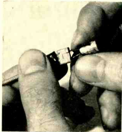
Closeup of cadmium-sulphide photocell mounted in transistor socket. This detector features compactness, low cost and reliability. Several types are available
