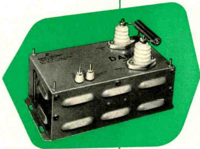
9000 Series, "HI-SEL" DC Power Packs Five models, from 0-5 KV and 5 ma up to 0-30 KV and 5 ma. Low ripple at all ratings. Selenium rectifiers and air-insulated design. Can be mounted in any position.
