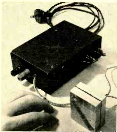
Complete photoelectric system. Bistable transistor amplifier is contained in chassis at top of photo. Slotted block holds radioisotope and shutter
