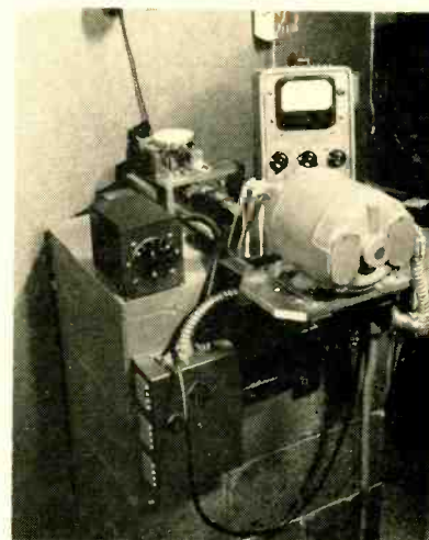
One form of microwave thickness gage uses a motor and reduction-gear train to achieve mechanical motion of horn
