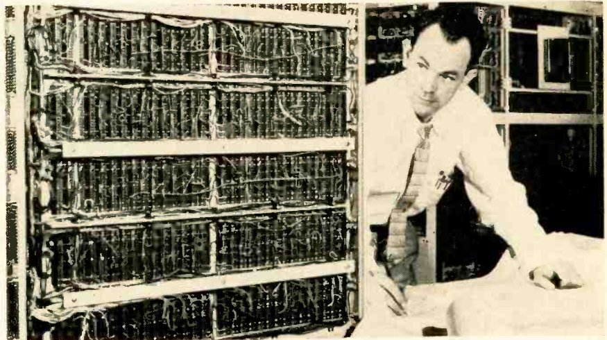
Engineer adds error-correction system to data-processing machine as . . .
