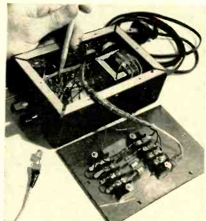
Internal construction of transistor amplifier. Pencil is pointing to 2N138A transistor. In left foreground are cadmium-sulphide photocell and cable
