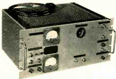
1000 Series, Rack-Mounted DC Supplies 0-1 to 0-60 KV, 2-500 ma. Rugged construction, conservative design, with full self-protection. Selenium rectifiers in models below 10 ma rating. Ripple; below 2.5% rms for max. current at max. voltage. Polarity reversible, with center-tap provision if desired.
