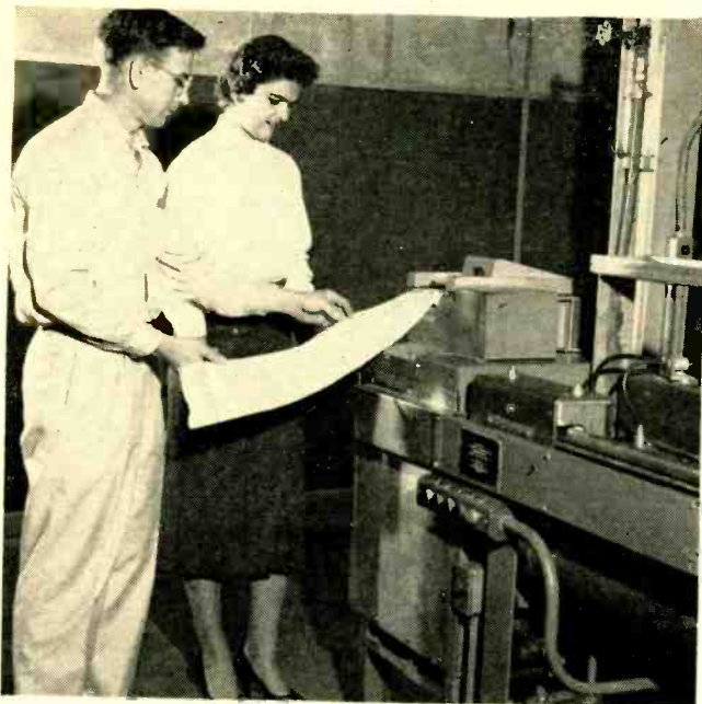
Flaws show up as irregularities in the plot of transmitted signal. Extent and location of defect is determined by attenuation
