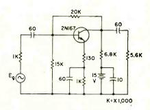
FIG. 4—Practical transistor a-c amplifier with selected component values. Use of 20.000-ohm shunt feedback resistor provides d-c and a-c voltage feedback and eliminates two components
