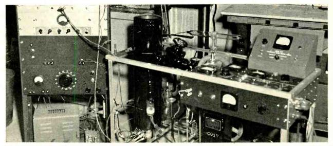
First experimental model of the Peritron. Vacuum tank is a 6-in. diam 30-in. long, seamless brass tube mounted in an angle iron table. Screen is viewed through a convex Pyrex window sealed to a shoulder turned in the upper end of the tank. Relay rack contains control circuits
