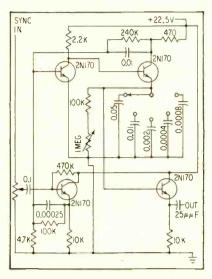
FIG. 1—Transistorized crt beam-direction marker has direct-coupled emitter follower to isolate oscillator from load
