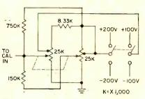
FIG. 4—Precision potentiometer circuit provides various input voltages into photoformer for calibration purposes
