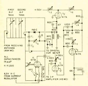
FIG. 4—Double-tuned coaxial tanks provide selectivity for receiver tuner. Unit provides 40 db rejection of image frequency
