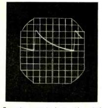
Generator output is shown with vertical scale of 5 volts per cm and horizontal scale of 2 microseconds per cm
