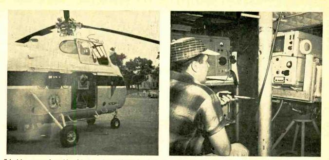
Television camera is positioned in open door of helicopter (left). Quarter-wave stub transmitting antenna extends below body when airborne. Internal view of helicopter (right) shows arrangement of camera chain and adjunct equipment
