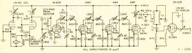
FIG. 3-Transmitter exciter consists of local oscillator, mixer, three amplifier stages and driver that provides 3-w to tripler stage
