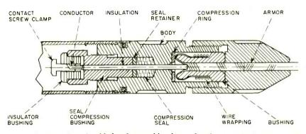
FIG. 2-Cross-section of cable-head assembly shows details of method used to seal probe against pressures which may rise as high as 2,000 psig
