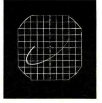
Lissajou display of 70-kc signal shows vertical voltage leading horizontal by an angle of 38 degrees
