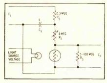
FIG. 1-Photoconductive chopper offers low noise level and resistance to vibration
