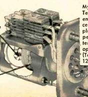
Mycalex stack, Tefton wire and end washers and ceramic pushers, plus sealed coll, permit high temperature operations. (Tested up to 125° C.) Hermetically sealing the coil of the MH "Seal-Temp" substantially increases the reliability and life of this popular telephone-type relay. Considered a major reason for relay failure, contact contamination due to outgassing of the coil has been eliminated by this sealing process.
