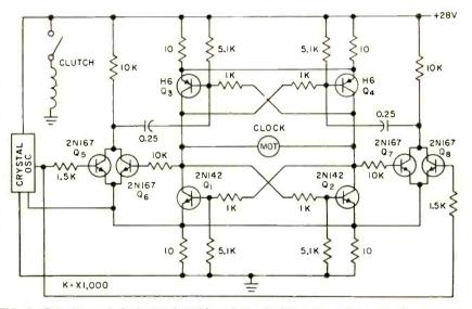
FIG. 1—Time-interval clock uses bistable voltage doubling chopper to provide a-c power necessary to drive synchronous clock motor with 0.02-percent accuracy
