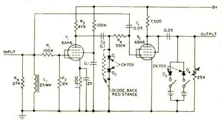
FIG. 1—Circuit of automatic amplitude control for audio section of radio transmitter
