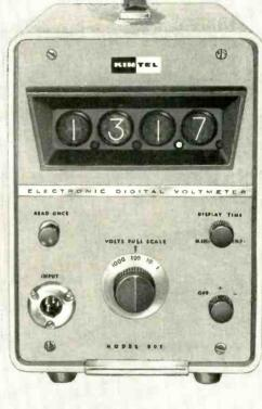
only in the delicate, complex and expensive instruments. Extremely stable operation – continuous calibration against an internal reference.
