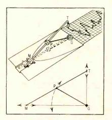
FIG. 1—Jeweled pivots convert curvilinear motion of the galvanometer movement to rectilinear motion. Rectilinear pen recordings have the same shape as a plotted graph and can be measured with a straight edge ruler.
