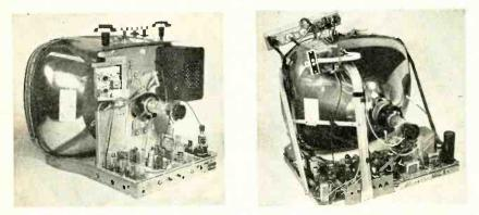
Relatively massive tv chassis (left) has been replaced by a lighter, less costly triangular chassis (right) which frames the picture tube and printed circuit board
