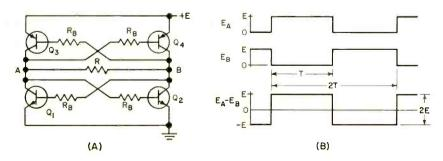
FIG. 2—Voltage-doubling chopper utilizes complementary symmetry feature of transistors (A) to double input voltage to that appearing across the load in (B)
