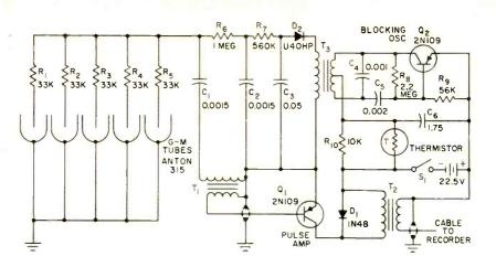
FIG. 1—Schematic of gamma-ray probe. High voltage for G-M tubes is provided by blocking oscillator  $Q_2$  and selenium rectifier  $D_2$ . Simple but effective temperature compensation is achieved through the use of a thermistor
