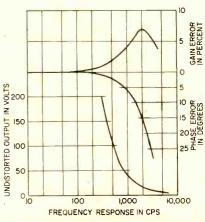
FIG. 2—Frequency response, phase error and gain error curves of photoformer. Response is flat to about 300 cps
