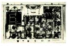
Cabling is used for power leads while signal wiring connects point-to-point
