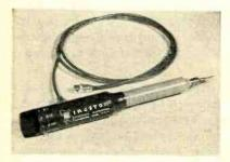
A direct prope can be used to convert to a highly sensitive direct-contact scope
