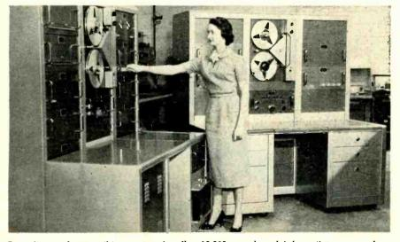
Recording and transcribing system handles 10,000 samples of information a second on its 100 channels. It was originally conceived by North American Aviation and developed by Minneapolis-Honeywell. The system incorporates multiplexing feature and provides analog to digital conversion
