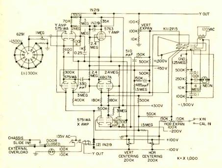
FIG. 3—Schematic of photoformer crt deflection system. Input to Y amplifier is cathode follower with cathode shield provided to minimize phototube output capacitance, achieving crt low spot intensity. Effective Y amplifier gain is about 1250
