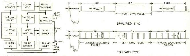
FIG. 5-Simplified-sync generator used in airborne system and its output compared to commercially used sync signals
