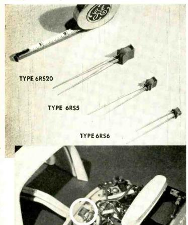
Three new clip assembly selenium rectifiers are now being produced in quantity by General Electric using the Vac-u-Sel process.
