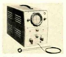
Waveform is displayed on the scope by picking up the electrostatic field around a component
