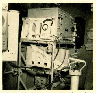
Transmitter (top) and sync generator (center) and mounted over 400-cps rotary inverter. Tube at right supports stub antenna
