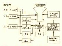
FIG. 1—Logic employed for generating three-dimensional patterns on display tube described in text
