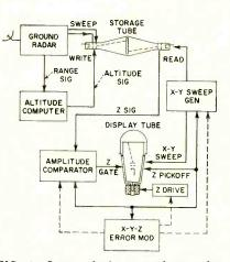
FIG. 4—One method of translating altitude and position data from the airport radar into a three-dimensional display. Error signals are shown in dashed line
