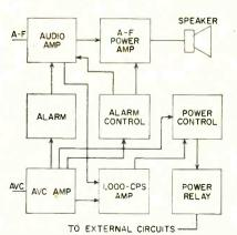
FIG. 3—Functional diagram of complete alarm system and control circuits pears at the grid of phase inverter  $V_{\text{gal}}$ . No volume control is provided for the alarm signals, which should be audible as far from the speaker as possible under all conditions. Tested range of audibility is about 1,000 feet under business-district conditions of ambient noise and more than 250 feet under airport conditions.
