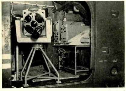
Closeup view of camera installation in helicopter shows camera control unit and power supply at upper right; 60-cps inverter is at lower right
