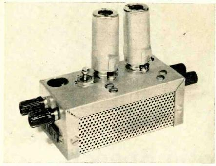
Miniaturized automatic amplitude control unit, designed for insertion in speech frequency line, consumes 11 watts. Plate power input at normal levels is about 3 w
