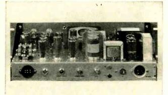
Standard relay-rack construction is used, with 3½-in. front panel
