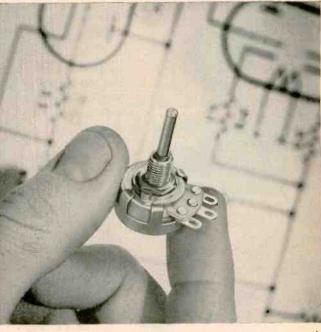
New high temperature miniature wirewound control ... only %" in diameter, is designed for ambient temperatures of 200°C and up. It has exceptionally high power dissipation for its sizerated 5 watts at 145°C. Control is gold plated to assure maximum shelf life, resistance to corrosion and high heat transfer. Easily adaptable to hermetically sealed mounting.
