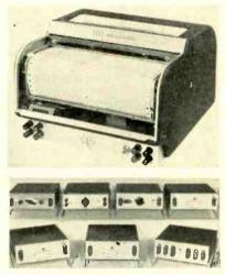
Accessory transducers enable the writing mechanism of one pen recorder to be used for many different types of measurements Unnecessary duplication of the high cost writing mechanism is eliminated.
