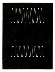
FIG. 3—Waveforms showing degree of clipping required for pure 1,000-cps sine wave (above) to limit output variations to approximately 1 db. Wave below is clipped 5.8 db
