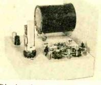
Side view of time-interval clock system shows mounting of circuit components
