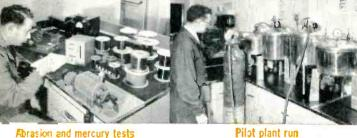
Abrasion and mercury tests on magnet wire
