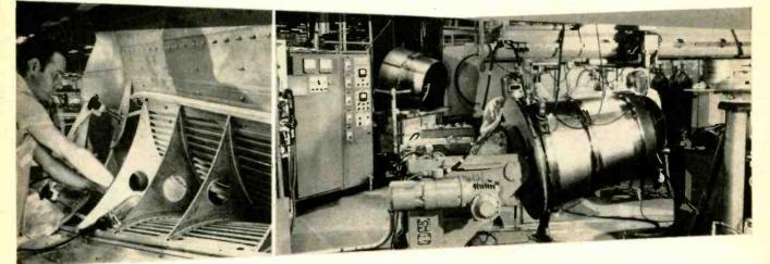
At Temco titanium is keeping its promises to the aircraft industry. No longer the intransigent metal, titanium in precision assemblies has become routine here. Through the development of Temco's Ti-Brite process, the tough titanium scale which once limited the material's usefulness is electrolytically removed without etching or disturbing the most precise dimensions.
