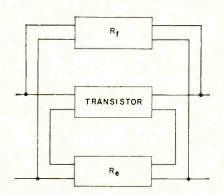
FIG. 3—Circuit shown can be used for matrix analysis technique. Matrix is derived by using equivalent a-c circuit shown in Fig. 2 and reducing transistor and feedback loops to 4-terminal networks Eq. 3, quantity  $A_v$  is equal to -12.9. This is slightly less than the desired 15. Selecting a smaller series feedback resistor,  $R_v$ , will tend to increase the voltage amplification. Therefore, if  $R_v$  is selected to be 130 ohms, Eq. 9 becomes
