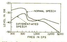
FIG. 2—Energy distribution curves for normal and differentiated speech
