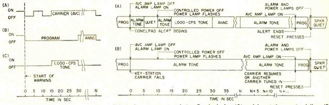
FIG. 1—Typical sequence of carrier (A), program (B) and warning-tone (C)
