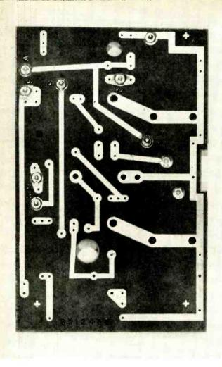
**Di-Clad 2350.** An economy paper-base phenolic grade having good tensile, flexural, compressive, and impact strength. Adequate for most non-critical printed-circuit applications. Can be cold punched and sheared up to 5/64 of an inch in thickness.
