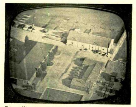
Picture on 17-in. monitor was transmitted from airborne camera chain by uhf f-m
