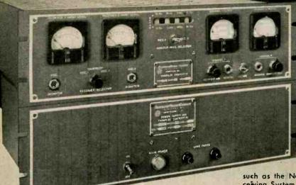
provide 2 channels of FS communication with existing single channel transmitter and receiving facilitieswith performance comparable to the existing single channel system
