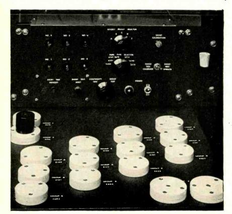
Three groups of four long-life tube sockets are used for most-required types. Octal adapter is used for subminiature types. Cork hammer aggravates tap shorts
