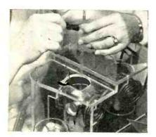
Glass seal is applied while tube is between heating coils. Tube at right is being brought to sealing temperature
