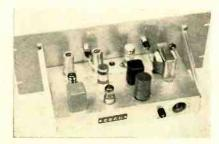
In-line mounting of plug-in components improves appearance, simplifies service
