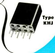
Allied's type KHJ and KHY subminiature relays were developed to meet the present "Automation" need for relays with incremental grid spaced terminals and with improved performance. These relays have a higher contact rating and are designed to meet the increased vibration and shock requirements of the latest MIL specs. They are available with mounting brackets that are interchangeable with Allied's present type KH subminiature relay.
