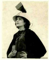
Unusual headgear is actually a horn antenna mounted on a helmet for picking up signals from aircraft navigation or bombing radars. It enables Ground Observer Corps personnel to detect aircraft more than 100 miles away. Output of eight-transistor amplifier is supplied to earplug
