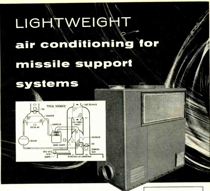
The mobility problem in cooling electronic equipment in vans and for missile pre-launching has been answered by new AiResearch Freon air conditioning units. One-fourth the weight and one-third the size of conventional equipment, these lightweight, airtransportable units utilize highly efficient AiResearch Freon components (see diagram) originally developed for commercial aircraft applications.
