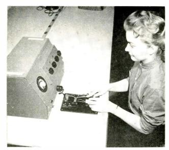
Resistance is quickly checked with a Wheatstone Bridge circuit adapted for go, no-go operation
