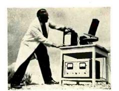
Mobile atmosphere radiation monitor finds radioactivity released from reactor stacks
