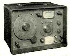
The 1064/2 provides highgrade fm outputs in the ranges 30 to 50, 118 to 185, and 450 to 470 mc; crystalcontrolled i-f outputs at five spot frequencies; and a 1 kc af output.
