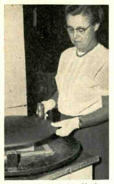
Tapping shadow mask with rubber hammer to remove dents, while shaped mandrel underneath provides support
