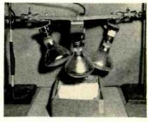
Heat of infra red lamps pre-expands polystyrene beads
