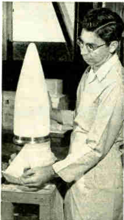
After compacting in press, protective bag is removed and radome is taken off mandrel for firing and finish-machining
