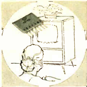
TV SETS—17 PEC's replaced over 100 parts, simplifying assembly and improving performance.
