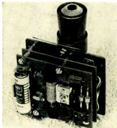
Interior view of transistorized microphone transmitter. Unit is compact and can be easily disassembled for repair through use of tier construction technique
