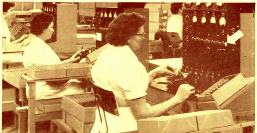
G-E 5-Star workers are shown checking tubes for intermittent short-circuits, employing General Electric's positive method of DC testing whereby a warning light at the right of the panel (arrow) continues to glow until the operator removes the faulty tube.
