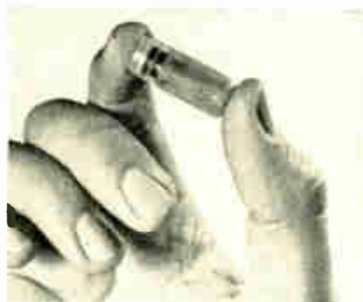
Endoradiosonde, the transmitter-modulator-transducer that is swallowed, is a capsule 2.8 cm long and 0.9 cm in diameter
