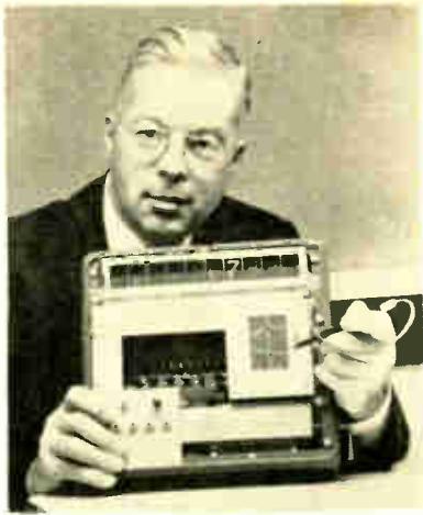
Handwriting reader. Operator writes numerals with stylus on special surface at right
