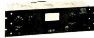
Model 60 Logarithmic Converter 60 db dynamic range; AC or DC; 20-20,000 cps; with AUTOGRAF and appropriate signal generator automatically plots gain-frequency characteristics.
