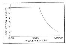
FIG. 2—Maximum vertical deflection as a function of frequency
