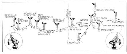
FIG. 1—Map of entire radar data collection system planned by CAA and designed for expansion to include selection of data from Bellefontaine. Columbus and Cincinnati
