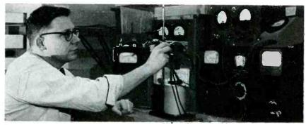
Laboratory setup used to measure gain-temperature characteristics of silicon transistors in 1-mc grounded-emitter i-f amplifiers with feedback and thermistor compensation
