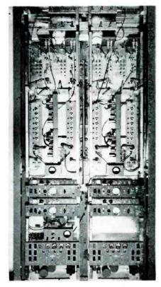
**VIEWS** of the outside and inside of the quadruple-diversity receiver used in commercial broad-band microwave tropospheric scatter system reveals that . . .
