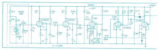
FIG. 2—Circuit of noise generator and transistor-ferrite-core binary. Series of pulses from noise generator causes negative of the two transistors. The resistor between base and emitter provides rapid transistor cutoff. The blanking pulses switch off the
