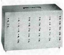
mensions of 101 in. long by 4 in. wide and 63 in. high. Twenty-five tap terminals are brought out on each of the length and height sides, for a total of 50 taps.
