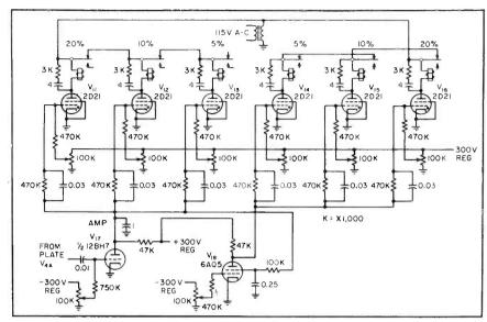
power supply potential. Plate voltage for the thyratrons is interconnected through the relay contacts; thus, only one relay can be energized at any one time.
