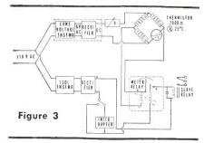
Because the thermistor has a large negative temperature coefficient of resistance, even minute changes unbalance the bridge to let the current actuate the relay.
