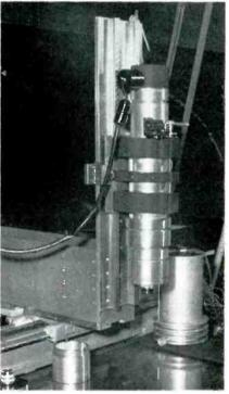
Arrangement of vertical tracks on cross slide for raising and lowering projector assembly
