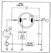
FIG. 2—Regulation system for stabilized electrostatic generator
