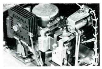
Small relay for control of auxiliary coil is bolted to same bracket that supports the selenium rectifier. Relay frame is insulated from bracket by insulating washers around the mounting screws
