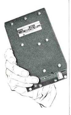
New, improved model designed for extreme environmental conditions (100g shock, 2000 cps vibration, —55 to +75°C). Subminiaturized and crystal-stabilized with telemetry band spurious output better than 60db below carrier.
