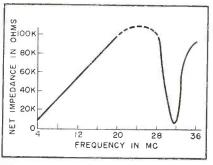
FIG. 3—Net impedance of six parallel r-f chokes as compared to frequency
