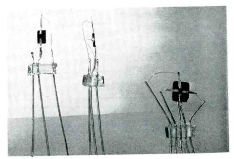
Front and side views of developmental single-direction photocell with multi-contact two-direction cell at right
