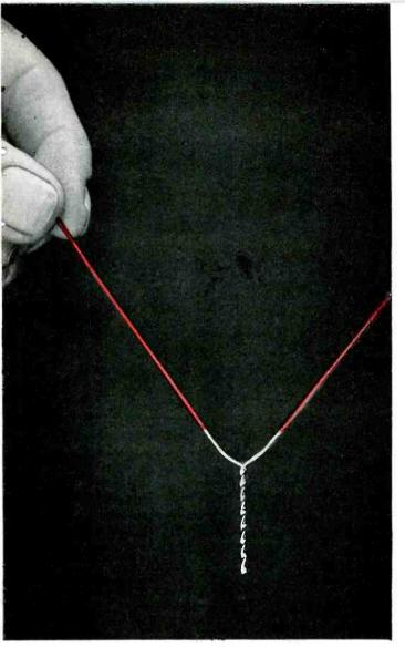
JOINT IS COMPLETED WITHOUT STRIPPING WIRE with Analac wire dipped in a 50-50 tin-lead solder at 360°C (680°F). The insulation is removed at the temperature of molten solder.
