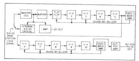
FIG. 1—Block of system shows feedback technique that produces count down from  $31.5~\mathrm{kc}$ , or twice the line frequency, to a field frequency of  $60~\mathrm{cps}$
