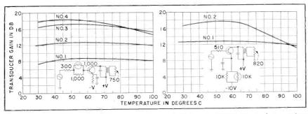
FIG. 3—Compensation resulting from thermistor in input circuit (A) and in emitter circuit (B) for silicon units of same type shows stability throughout temperature range
