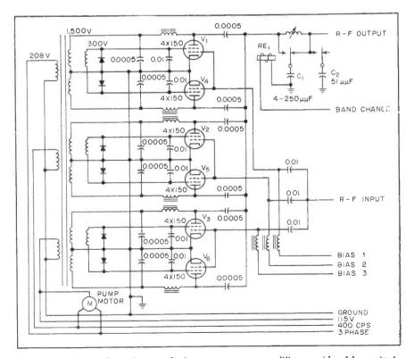
FIG. 2—Six-phase self-rectifying radio-frequency power amplifier provides 1-kw output using six 4X50 tubes immersed in silicone cooling liquid
