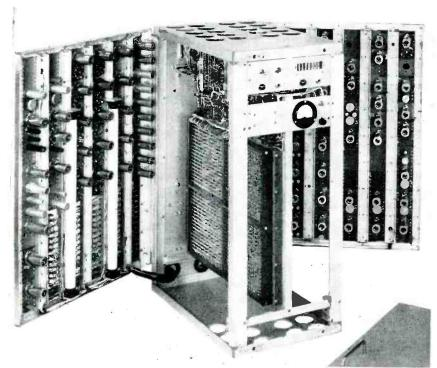
When converter unit is pulled out from rack on roller suspension, hinged side chassis units swing out to give access to tubes and to neon-tube matrix on center section. Fluorescent lamps mounted between vertical rows of tubes on left chassis insure consistent operation of neon tubes in matrix
