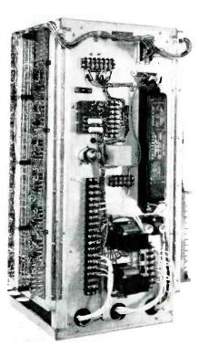
Rear view of converter unit, showing fluorescent lamp ballast mounted on panel and starters directly below. Side panels are supported by piano hinges
