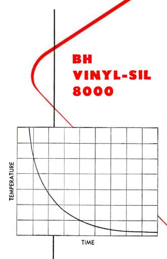
BH Vinyl-Sil 8000 Fiberglass Sleeving offers outstanding resistance to heat-aging, a major factor in insulation breakdown. It retains flexibility and its minimum guaranteed dielectric strength of 8,000 volts even after these exposures:
