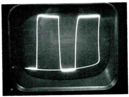
Appearance of 2,000-cps square wave signal on 21-inch screen. Display is approximately 12 inches high. Pattern is essentially identical to input signal
