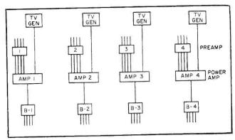
FIG. 8—Method of injecting locally generated signal by using separate generator for each amplifier branch
