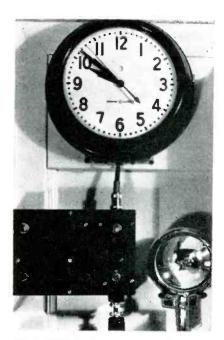
When clock is off-time, lower right switch on panel is turned on. Ready button, left of switch, stops second hand at zero. Clock is set to time announcement and switch is turned off
