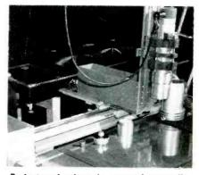
Projector of printer is mounted vertically on ways of lathe which moves over heavy surface plate on which is placed negative to be exposed. Counter wheel housing is at left end of lathe
