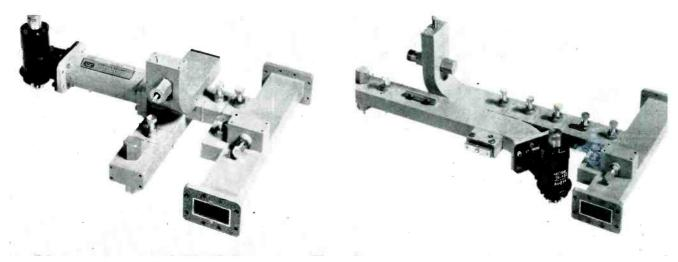
Microwave transmitting plumbing (left) and receiving plumbing (right) showing band-pass and band-reject filters used as part of multiplexing technique. Klystron used for both transmitter and local oscillator is a 100-mw tube modulated  $\pm$  3 mc
