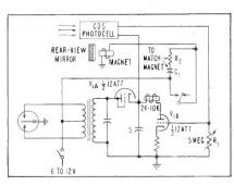
Single 12AT7 serves as rectifier and relay control tube in mirror system
