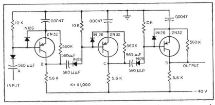
FIG. 1—Transistor delay line for airborne digital computer has delays of 40 microseconds per section for total delay of 120 microseconds
