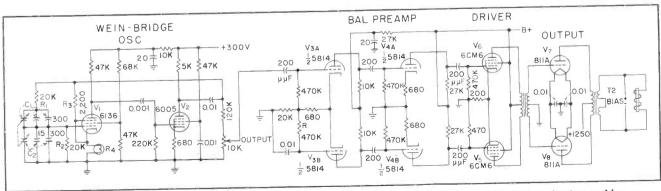
FIG. 2—Complete schematic shows how relatively standard circuits can be adapted to solve an industrial packaging problem
