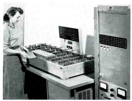
Inserting punched card which controls programming for measuring d-c resistance values of windings in up to 24 transformers. Hooks on ends of test leads speed connecting
