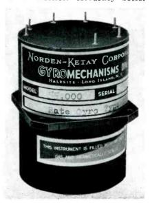
than  $\pm \frac{1}{2}$  percent full scale can be obtained. The gyro can be supplied in a variety of maximum rate ranges from 1 deg per sec to 1,000 deg per sec. It incorporates an inductive signal pickoff, which provides a higher power signal output than has previously been available in this size rate gyro. The power signal output enables the use of minimum gimbal displacement, consequently yielding high natural frequency.
