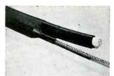
Method of molding strain relief breakout around stainless steel wire rope used to support long cable during firing of large missile
