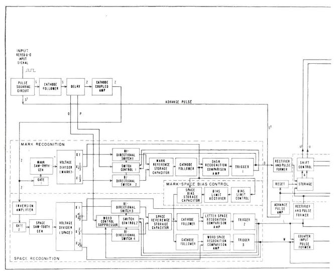
FIG. 2—Automatic Morse-to-teleprinter converter arrangement. Input Morse signal may be keyed audio tone from radio receiver or
