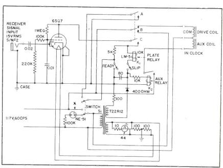
FIG. 1—Electronic time-setter is turned on at  $S_1$ . Relay  $K_2$  energizes the auxiliary coil in clock. Ready button activates relay  $K_1$ , which shorts the switch and stops the clock. After clock is set manually to time of next verbal announcement,  $S_1$  is turned off and relay  $K_2$  is held only by plate current of the tube. Tone signal from WWV releases relay, starts the clock at the exact time and de-energizes the auxiliary coil
