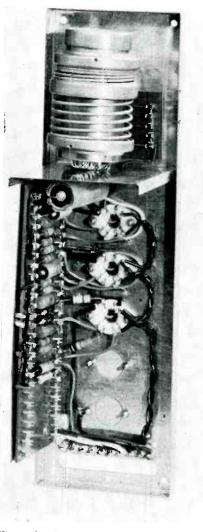
View of noise generator chassis shows suspension system provided for neon tube to minimize injection of external noise frequencies resulting from vibration
