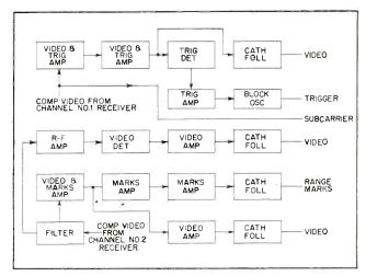
FIG. 3—Decoding at receiving stations is done as indicated in block diagram. The 400-cps demodulators are not shown
