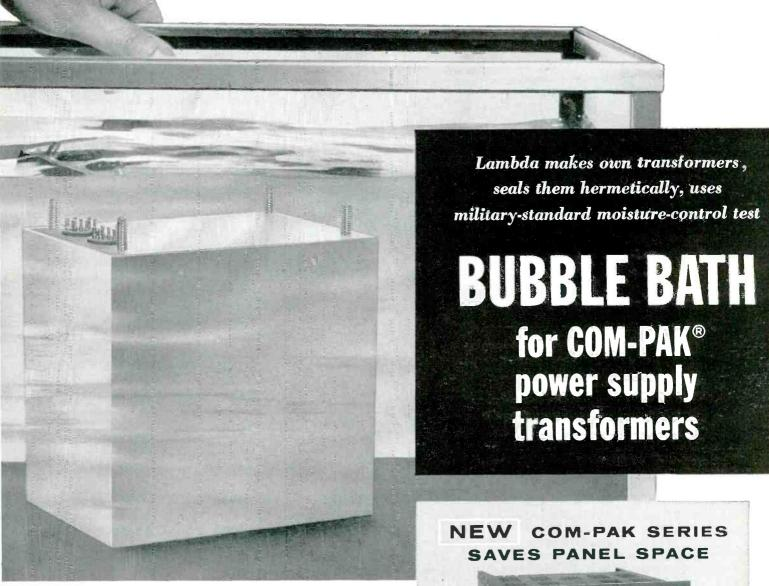
Evary Lambda Com-Pak power supply transformer gets a pre-installation soaking in hot water. A single bubble and the transformer is rejected. The unit installed in your Lambda Com-Pak power supply has passed this military test... assurance of long, trouble-free service.
