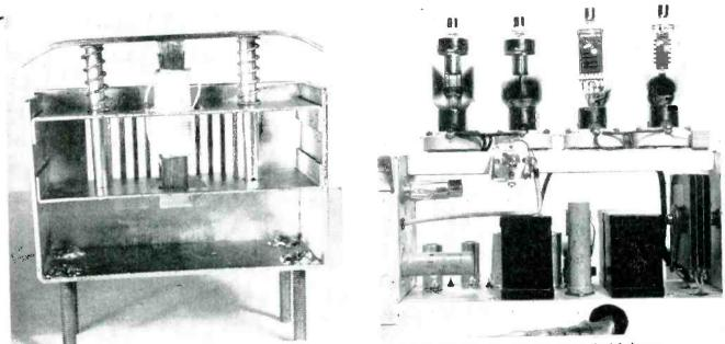
Magnetostriction transducer (left), driven by output of ultrasonic generator (right), has a laminated oxidized nickel core
