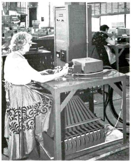
At sorting position, operator now merely inserts mica sheets one by one between gaging contacts. Electronic gage measures thickness to thousandth of inch and drops sheet into proper receptaçle below. Control equipment is in relay rack at rear
