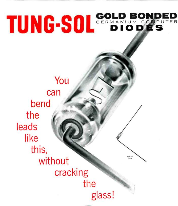
Here's the answer to the problem of how to make computer diodes so the lead wires can be sharply bent close to the glass body without cracking the end seal. It's the "ring seal" design, an exclusive Tung-Sol construction feature embodying a metal collar fused into the end-seal. The collar absorbs the strain of lead wire bends, thereby preventing damage to the diode enclosure.
