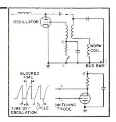
FIG. 1-Manual system of controlling oscillator output (A) compared with automatic system that replaces switch with triode (B) in oscillator grid circuit
