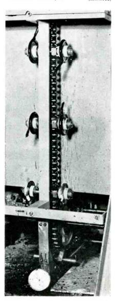
Endless chain conveyor arrangement used for applying protective hot-melt coating to flyback transformer coils. Operator unloads coated coils here as they move down, and puts on new coils for trip across top of pot
