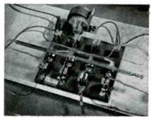
Experimental torsional wave delay line using disk and rod construction
