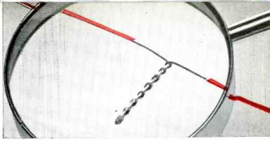
**STRCNG JOINTS**—as strong as the same joints made in bare copper wire—are produced. Here in laboratory test, joint holds under high stress.
