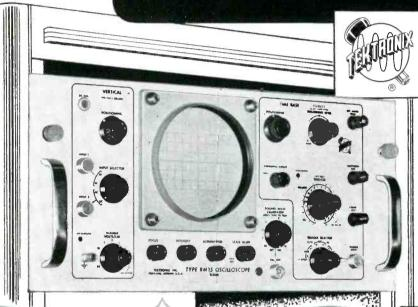
The Tektronix Type RM15 is a high - performance 5 - inch oscilloscope, electrically identical to the Type 515. It mounts in 83/4 vertical inches of the standard instrument rack, is supported on a slide-out mounting, and can be tilted and locked in any of seven positions for servicing convenience.
