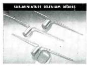
Developed for use in limited space at ambient temperatures ranging from -50°C to +100°C. Encapsulated to resist adverse environmental conditions. Output voltages from 20 to 160 volts; output currents of 100 microamperes to 11 MA. Bulletin SD-1B
