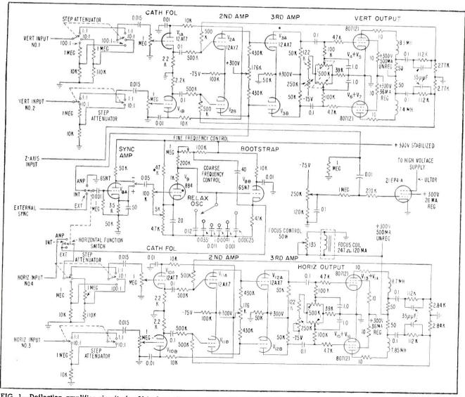
FIG. 1—Deflection amplifier circuits for 21-inch oscilloscope using television receiver picture tube. Power supply circuits (not shown) are conventional
