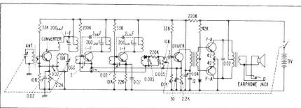
Latest in a line of compact Japanese broadcast receivers is the Sony TR-63 that employs six transistors and a varistor to avoid damage in case the battery is reversed. The varistor also compensates for temperature effects. Sensitivity of the receiver is a millivolt and it has a maximum undistorted output of 20 mw. Selectivity is approximately 15 db 10 kc off. Set is made by Tokyo Tsushin Kogyo, Ltd., Western Electric Transistor licensees
