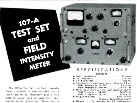
The 107-A Test Set and Field Intensity Meter combines in one portable unit a radio receiver of laboratory quality with metered output and an accurately calibrated signal generator. These instruments, which can be used separately for a variety of test purposes, cover a frequency range of 54 to 240 megacycles without band changing.
