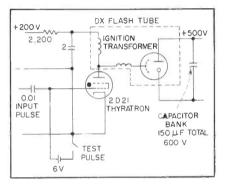
Triggered electronic flash circuit
