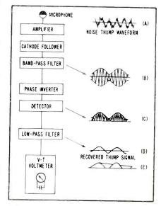
FIG. 3—Block diagram of thump detector
