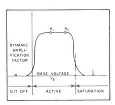
FIG. 3—Typical dynamic characteristic curve for junction transistor switching circuit showing possible operating prints
