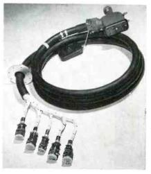
Example of special missile-launcher cable harness having neoprene jacket which remains flexible down to —65 F. Five connector fittings at lower left are anchored in waterproof junction box. Flange on cable provides seal to box
