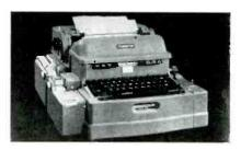
Flexowriter equipment for typewriting of data and simultaneous paper tape punching may be used with NLS digital voltmeters and ohmmeters. NLS Flexowriter converters are provided for this purpose.
