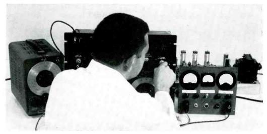
Differential voltmeter unit (foreground) with relay control unit at rear are used with Schering bridge to sort capacitors with a high degree of accuracy in developmental setup
