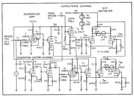
FIG. 2—Capacitance and dissipation factor channels for automatic capacitor sorting system use similar circuits for differential voltmeter
