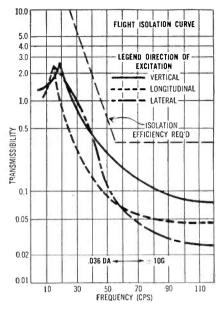
Figure 2. Graph showing in-flight performance characteristics of the distributedelement mounting system.
