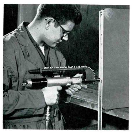
A COMPLETELY AUTOMATIC power screwdriver, developed for mass assembly operations by the Shake-proof Division of Illinois Tool Works, drives screws automatically at any angle as fast as the operator can pull the trigger. Weight is only  $6\frac{1}{2}$  lb.
