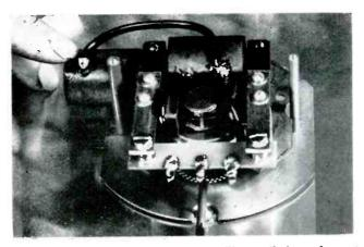
Clock modification incorporates an auxiliary coil shown here at left of main coil. This auxiliary is connected across the a-c line and disables the clock current failure indicator
