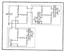
FIG. 6—Experimental distribution network giving four outputs
