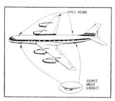
FIG. 1—Typical placement of infrared detectors on plane. Size of irdomes relative to plane is exaggerated
