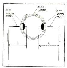
FIG. 1—Basic operation of electrostatic high-voltage generator
