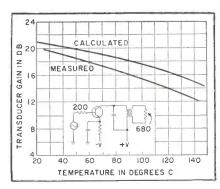
FIG. 1—Curves give calculated gain and measured gain for configuration shown
