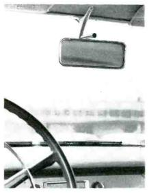
Small tube over rear-view mirror houses cadmium-sulfide photocell that controls mirror position with glare
