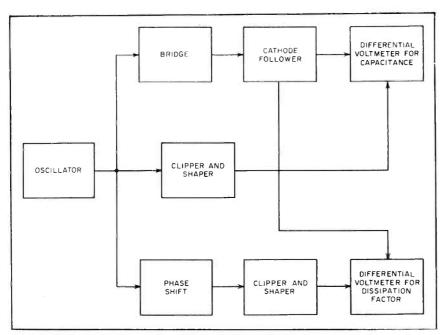
FIG. 1—Two-channel system for sorting capacitors for dissipation factor and capacitance value uses Schering type bridge to obtain in-phase and quadrature signals
