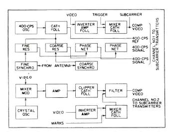
FIG. 2—Block diagram shows method used in encoding video, marks and antenna position information at transmitting site
