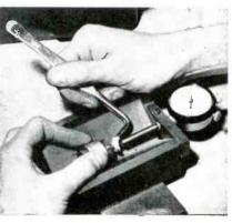
Method of using fixture for checking end play of precision servo motor
