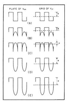
FIG. 5—Plate and grid waveforms for balanced bridge (A), small positive capacitance unbalance (B), large positive capacitance unbalance (C), small negative capacitance unbalance (D) and large negative capacitance unbalance
