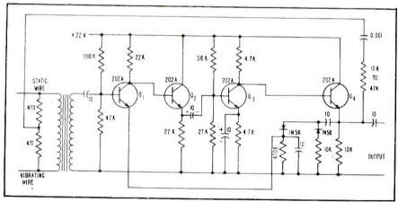
Circuit of improved version of amplifier used in bathythermometer
