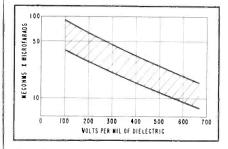
Megohms times microfarads vs voltage stress for mineral-oil impregnated capacitors at 125 C
