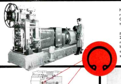
New Model TA-625 2-high/4-high combination rolling mill designed by Stanat Manufacturing Co., Long Island City, N. Y., reduces  $2\frac{1}{2}$ " ingot to precision-rolled strip as thin as .001".
