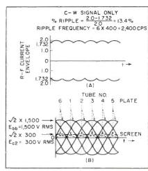
FIG. 1—Ripple frequency (A) and plate and screen voltages (B) for six-tube radiofrequency power amplifier for aircraft
