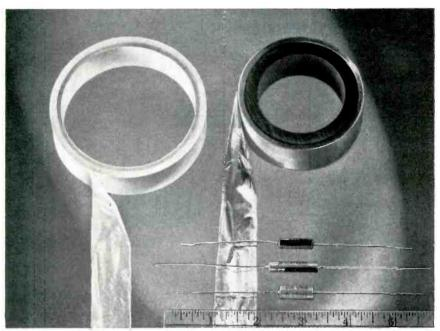
High-temperature capacitors using thin dielectric films of TEFLON are rated for a temperature range of -70°C. to +200°C. Shown are films of metallized TEFLON 1/4 mil thick,
