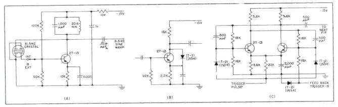
FIG. 2—Basic circuits. Output of crystal-controlled master oscillator (A) is clipped at (B) and triggers flip-flop counters as in (C)
