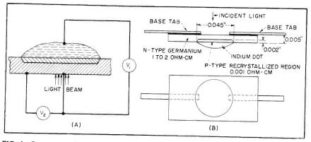
FIG. 1—Basic operation of lateral-effect photocell (A) and its construction (B)
