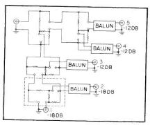
FIG. 7—Method of adding basic network to give five outputs
