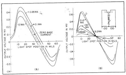
FIG. 4—Axis shift with bias current provides a scanning action (A) and electronic chopping is obtained by applying various values of forward current through dot (B)
