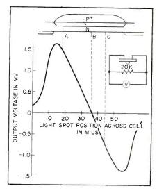
filtering out from the applied sweeping current. But this returns to the speed limitations of mechanical devices. However, it is possible to make an electronic equivalent of light chopping.
