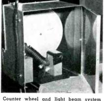
using photocell and transducer
