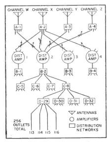
FIG. 1—Example of 256-outlet antennamultiplex system providing choice of four ty channels
