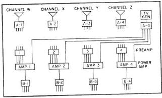
FIG. 9—Use of one generator for injecting locally generated signal for test purposes or for laboratory experiments
