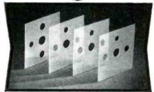
Low thermal expansion, high dielectric strength of these .002" thick mica sheets help maintain top performance in heavy duty power transister application.
