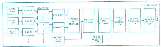
FIG. 1—Block diagram of ERNIE. Ten noise generators are used rather than nine to ensure that the machine operates when one generator fails.
