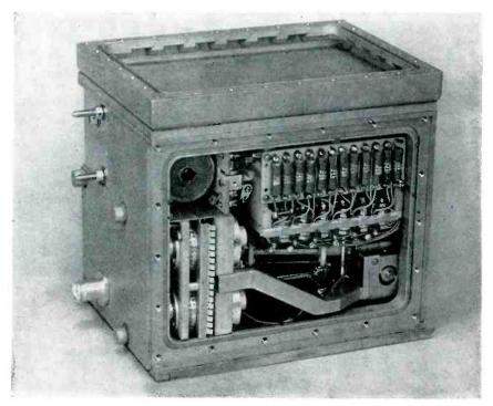
Complete amplifier in housing. Fluid expansion chamber is at top, output tubes at lower left with fluid circulating pump and ducting across bottom
