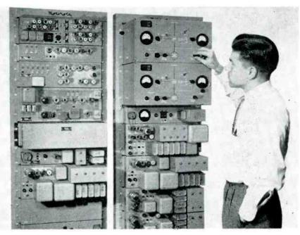
Rack-mounted r-f and auxiliary equipments provide microwave carriers in the 7-125 to 8.000-mc range (left). Engineer (right) adjusts klystron tuning of receiver, part of two-channel radar relay terminal. Auxiliary equipment provides rapid maintenance facilities
