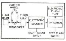
Block diagram of electronic system feeding flash tube
