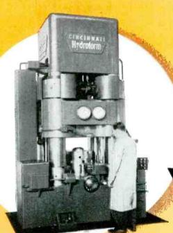
Kaupp hydroformed prototypes and pre-production parts are accurately formed and drawn in less time, at lower cost. Hydroforming produces short run, and in some cases production pieces, quicker and more economically than tool and die methods. New equipment installed by Kaupp assures faster service. For complete information on Kaupp metal forming facilities, call or write today!
