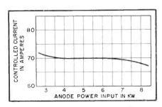
FIG. 3—Curve shows regulating characteristics under varying oscillator load
