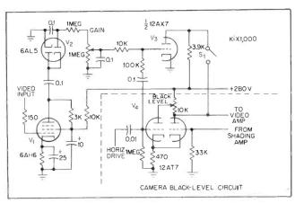
FIG. 3—Control circuit for use with RCA TK20-D iconoscope chain
