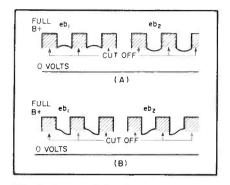
FIG. 3—Differential voltmeter waveforms with in-phase (A) and out-of-phase conditions (B)
