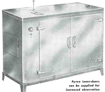
Aminco forced-convection ovens employ a motor-driven blower which produces movement of a large volume of heated air, horizontally across the work chamber. This, together with the circular arrangement of the heaters, results in uniform distribution throughout the entire work chamber. Air velocity is adjusted by means of a damper. Ovens are equipped with positive locking latches, adjustable perforated shelves, and a removable control panel.
