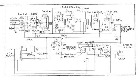
FIG. 1—Respiration monitor in iron-lung control system switches operation to automatic if patient does not start inspiration cycle after set time
