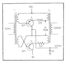
Half-wave demodulator for 2-kc carrier using two transistors. Full-wave version would use two-circuits of this type and additional transformer windings
