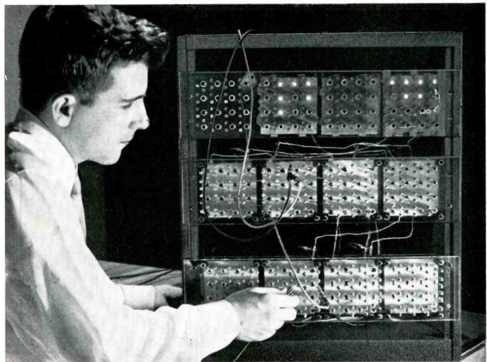
AN ELECTRONIC PHYSICIST in an NCR Research Laboratory evaluates new circuitry that utilizes electroluminescent optical switching devices as part of a basic study program.
