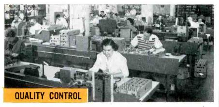
Scientific quality control practices and 100% testing to critical Military Specification requirements, including a hermetic seal test by mass spectrometer, assure standard quality in every relay.
