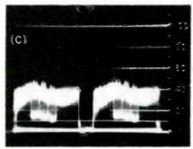
FIG. 1—Output waveform from manually controlled iconoscope chain for average (A), large white area (B) and low-contrast (C slides with no adjustment made for slide content or density
