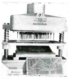
Multiple-spindle drill uses an easilychanged basic drill head, for short-run production of a variety of printed circuit boards. In foreground is example of drilled board. Drill heads are made by Zagar Tool, Inc., Cleveland, Ohio
