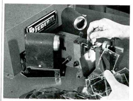
Insertion of sheet of mica between gaging contacts breaks light beam to photocell, causing contacts to move together, grip mica and measure it for thickness. Contacts then open and sheet drops through opened trap door for that thickness
