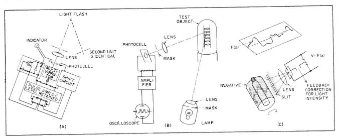
FIG. 5—Typical applications for lateral-effect photocell include light flash locator for determining source of gunfire (A), vibration detector for testing for microphonic electron tubes (B) and computer function generator (C)
