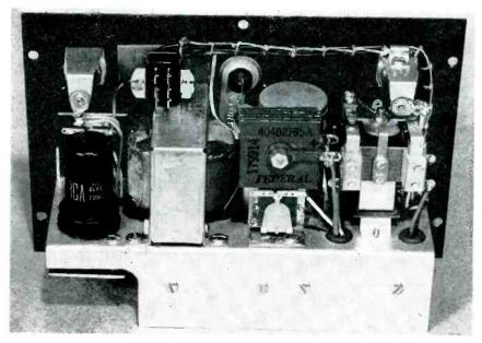
Rear chassis of clock-setter shows six-terminal plug above transformer which engages the mating socket, bolted to the top of the case
