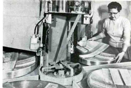
Loading tray of subminiature guided-missile and radar tubes on turntable of new automatic x-ray machine. X-ray tube is in heavy metal shield box at rear over turntable
