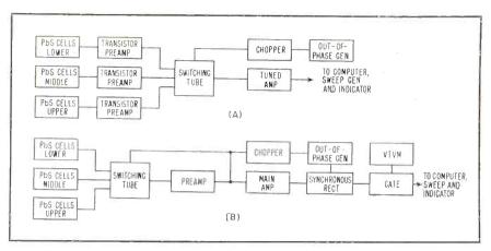
FIG. 2—Two infrared aircraft proximity warning systems in block form
