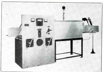
At left—front view of C. M. Manufacturing & Machine Co.'s high temperature hydrogen atmosphere furnace for metallizing ceramics, containing two NOTHELFER TRANSFORMERS.
