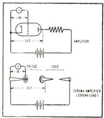
FIG. 2—Comparison of conventional triode and corona triode amplifier circuits
