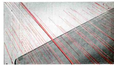
2 EXCELLENT ABRASION RESISTANCE of Analac is shown in this test. It has the same high windability normally associated with Formvar, Plain Enamel.
