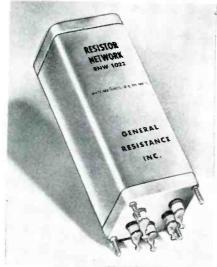
newly designed precision resistance network splits 600 volts into two parts within 0.01 percent over the temperature range of 0 deg to 100 C and under adverse environmental conditions. The network is completely encapsulated and hermetically sealed. It is capable of taking surges of double rated voltage.
