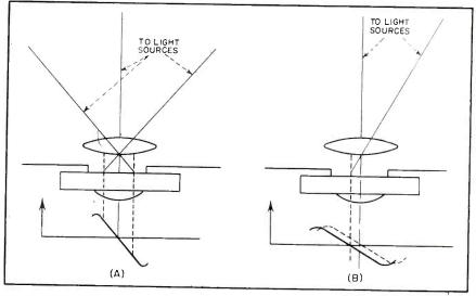
FIG. 3—Light source can be indicated by variation of cell output (A) or by electronically shifting axis of characteristic to obtain null (B)
