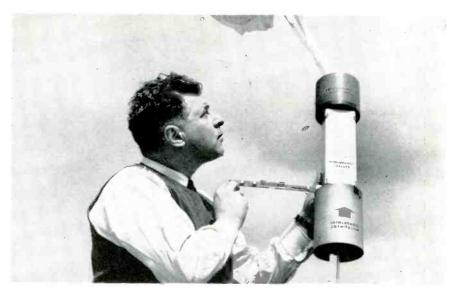
**ELECTRONIC** weather paratrooper, new type of high-altitude sonde, is checked in flight position by General Instrument engineer. The equipment is a . . .
