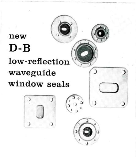
These rugged hermetic seals pass microwave energy with minimum reflection loss. Soldered directly to the waveguide flange, they seal out moisture, dust, oil, and salt spray—or maintain constant pressure or constant dielectric inside.
