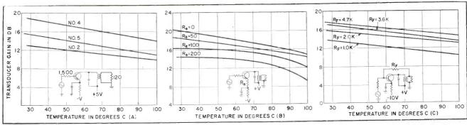
FIG. 2—Effects of compensating grounded-emitter narrow-band amplifier by mismatched impedance (A), emitter feedback (B) and negative feedback (C). Numbers identify transistors tested in circuit configuration associated with curves
