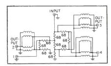
FIG. 2-Four-output distribution network
