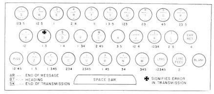
FIG. 1—Teleprinter keyboard, with equivalent Morse code signals on keys. Numbers below keys give positions of marking pulses in corresponding 5-digit teleprinter code; thus, letter F has pulses in 1st, 3rd and 4th spaces
