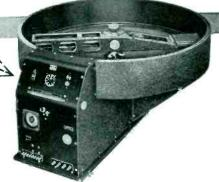
MODEL 878 Used primarily for testing relays, switches, tubes, motors, valves, and other small components, and to calibrate and evaluate accelerometers. Accommodates objects weighing up to 25 lbs.; has G-range of 0.017 G to 120 G's. Maximum centrifugal capacity is 1200 G-pounds. Nominal radius of gyration 24"
