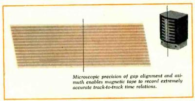
For time correlation the head stacks on an Ampex Tape Recorder are like an "electronic tee-square." All of the gaps are in line within 1/10,000th inch. And gap azimuth is accurate to a minute of arc. Tape moves past the head at speeds up to 60 inches per second and multiplies the track-to-track timing accuracy accordingly. (But consult us at Ampex before you rely on simple arithmetical conclusions).
