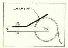
Method of mounting aluminum strip on frame of spool rack
