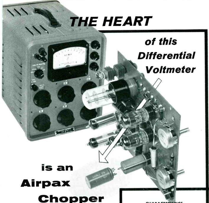
A chopper amplifier extends the range of this null-reading VTVM down to  $0\pm0.01$  DC volt. An Airpax Type 175 chopper modulates the input signal at 60 CPS so that it can readily be amplified and then the chopper synchronously rectifies the signal and returns it to the DC portion of the meter.
