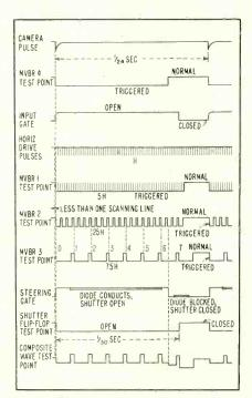
FIG. 3—Waveforms covering time of one horizontal line, one horizontal blanking period and start of next line. Circuit test points are shown in Fig. 2
