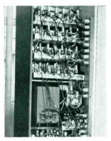
Extensive use of plug-in subassemblies is evident in this view of the counter. Duct at right distributes power to assemblies
