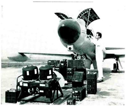
**COMPLEX** radar control, the brain of F-94 interceptor planes guarding the North American continent, is checked and installed by Hughes technician while . . .
