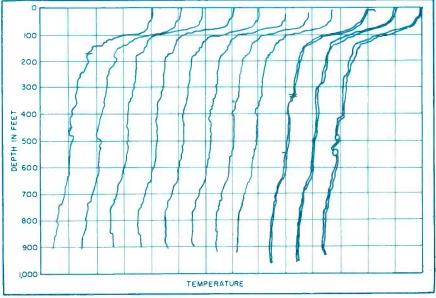
FIG. 7—Typical family of temperature-depth curves obtained with bathythermometer off the coast of San Diego, California
