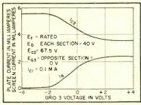
FIG. 10—Average transfer characteristics for one section of 6BU8 tube
