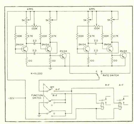
FIG. 3—Transistor multivibrators pulse r-f or a-f modulation at either 4 or 6 pps rate through relays installed in signal generator
