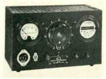
components. The unit operates on 115-v 400-cycle single-phase power and provides a continuously adjustable output from zero to 115 v under a maximum load current of 15 amperes. Standard instrumentation includes a  $3\frac{1}{2}$ -in. 21-reed  $\frac{1}{2}$ -percent accuracy frequency meter and a 2-percent accurate a-c voltmeter.
