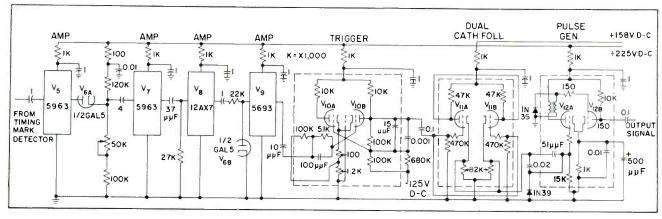
FIG. 4—Timing-pulse circuit. Negative pulses at 3-degree intervals are generated from capacitance variations between timing wheel and displacement pickup that are amplified and shaped to trigger the blocking oscillator output stage
