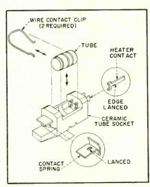
FIG. 4—Construction of 500 C socket for ceramic tube
