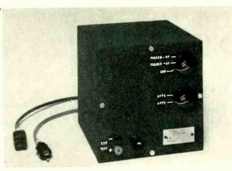
Compact keying unit contains all components except relays, which are mounted in signal generator cabinet
