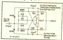
FIG. 3-One of three high-speed binary circuits used in gating unit
