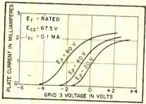
FIG. 8—Average plate characteristics for one section only
