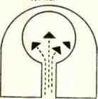
Now . . The Paraballoon is completely air supported — even lighter and more easily erected. Air supported structures as large as 65 ft. in diameter and over 100 ft. high are under study.
