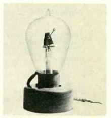
Developed by John Ambrose Fleming in 1904, the diode shown above constitutes the first practical application of the Edison effect and became the forerunner of basic detectors and rectifiers. It is part of a display by International Rectifier Corp.
