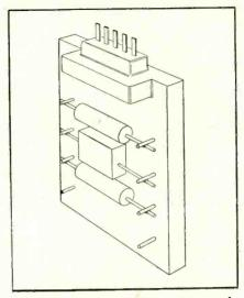
FIG. 5—Terminal arrangement in ceramic submodular chassis
