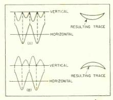
FIG. 3—Mouth generator waveforms, smiling (A) and frowning (B)
