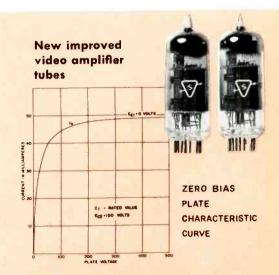
The sharp-cutoff pentode sections of the types 6AW8A and 6BA8A have been redesigned to exhibit a lower knee characteristic as shown in the graph. This permits a wider range of B+ supply voltages. In addition, pentode plates have been redesigned to increase dissipation from 3.0 to 3.25 watts.
