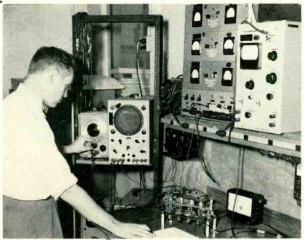
Breadboard version of electronic shutter under test. Author adjusts audio oscillator to deliver 24-cps signal to squaring amplifier at rear on bench whose 24-cps square-wave output simulates film exposure pulse. Another square-wave generator, on shelf It right, delivers 15,750 pps to simulate tv H pulses
