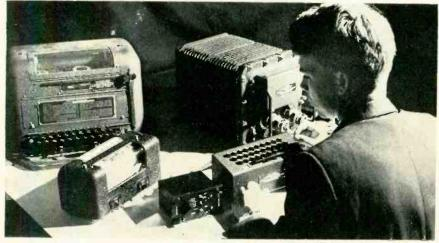
Airborne teletypewriter developed for Air Research and Development Command by Kleinschmidt Laboratories, Inc. is compared with standard machine (upper left). Printer section of the new machine is shown at left with control box (center) and keyboard (right). Terminal unit, which is the heart of the new teleprinter is at upper right. The new machine uses a type wheel and hammer on a pressure-sensitive paper
