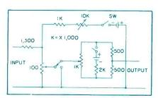
FIG. 6—Zero set circuit used with recorder. Variable resistor and potentiometer are helical type
