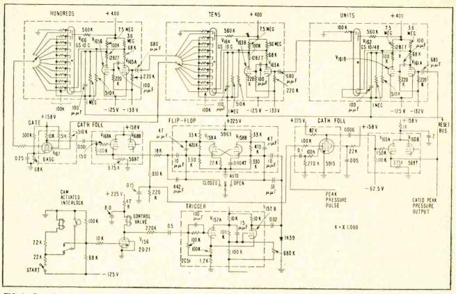
FIG. 6—Control and totalizer circuits show how peak pressure pulses are gated when particle control valve is actuated. Output is obtained when three-decade totalizer counter reaches its preset value which may be any multiple of 10 up to 10,000
