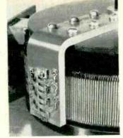
Six brushes in multiple, pigtail-equipped brush holders, readily removed for servicing or replacement - copper radiator nose and brush holder conducts current and heat to painted radiator, for maximum heat dissipation.
