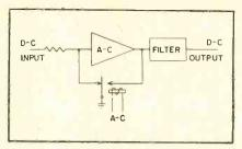
FIG. 2—Basic full-chopper d-c amplifier was adapted to missile instrumentation
