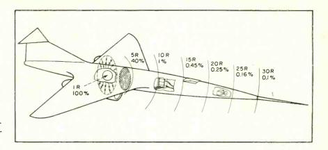
FIG. 1—Hypothetical arrangement of nuclear-powered aircraft shows relative radiation at distances in radii from reactor
