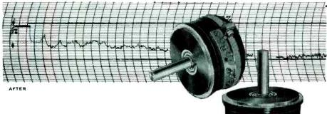
Take for instance a recent test report on the TIC Type ST20, a 2-inch, low-torque, ball-bearing precision potentiometer. The life test was conducted on a standard 6500 ohm unit. At 30RPM the ST20 was subjected to 700,000 eycles, reversing direction every 30 minutes. The linearity graphs shown above show the before and after of the ST20's independent linearity. As can be seen, the linearity change is imperceptible.
