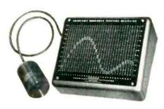
The VERNISTAT Adjustable Function Generator—a variation of the VERNISTAT a.c. potentiometer—permits quick and easy alteration of any nonlinear function. The adjusting mechanism provides a graphic display of the function which may be mathematical or empirical, including those with multiple slope reversals.
