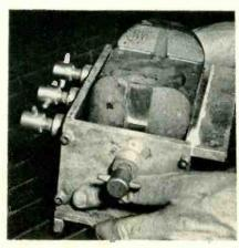
Placing jig in oven for curing bond
