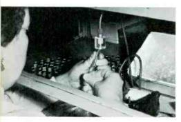
Visual inspection—visual inspection criteria as outlined in MIL-E-1C is applied to Guided Missile Tube production. This highly stringent and definitive spec helps to insure optimum reliability.
