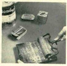
Rolling out Bondmaster M620 adhesive on palette just as it comes from can, to give uniform coating on application roller. Alnico magnets and lamination stack to be joined for Westinghouse recording wattmeter are shown in background
