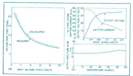
FIG. 3—First stage gain (A), output and age response (B) and frequency response curve (C) for transistor amplifier used for depth measurement
