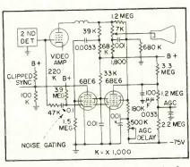
FIG. 5—Second type 6BE6 pentagrid tube is added for aga amplifier
