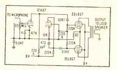
Amplifier for the delayed channel
