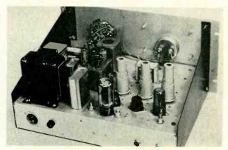
Speed indicating unit (left) is designed for rack mounting. Rear of chassis (right) shows plug-in units for squaring circuit, pulse amplifier and multivibrator at center of chassis. This design reduces instrument-repair downtime
