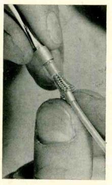
Pushing inner ferrule under shielding. Outer ferrule is temporarily over vinyl jacket, with two grounding wires under it. Grounds are made at the ferrules rather than at the connecting plugs
