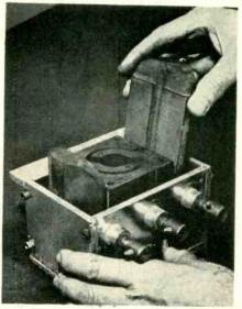
Assembling parts to be bonded in special jig. Thumbscrews on side and at far end provide all the contact pressure needed
