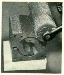
Applying cement to laminated core
