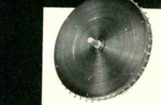
Special RL-270A-5 with 48 taps, shows maximum number. Allows 47 equal resistance sections, while maintaining guaranteed linearity af  $\pm 0.1\%$ . Total resistance of 500,000 ohms, resolution of 0.0075%.
