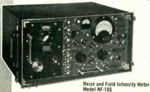
Empire Devices Noise and Field Intensity Meter Model NF-105 permits measurements of RF interference and field intensity over the entire frequency range from 150 kilocycles to 1000 megacycles. It is merely necessary to select one of four individual plug-in tuning units, depending on the frequency range desired. Tuning units are readily interchangeable...can be used with all Empire Devices Noise and Field Intensity Meters Model NF-105 now in the field.
