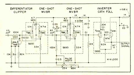
that is normally set to 20  $\mu sec$  by the pulse width control
