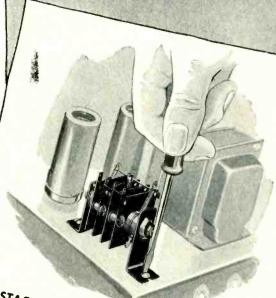
STACK INSTALLATION. A typical way of mounting General Electric Silicon Rectifier Stacks. Just two screws fasten the entire assembly in place.
