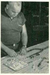
Placing identifying sleeves on leads. Adhesive-faced cardboard in front of operator serves as tote tray for sleeves
