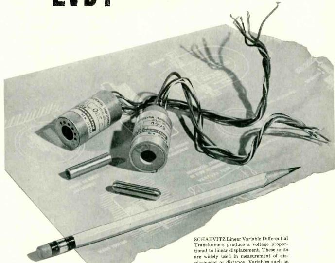
Transformers produce a voltage proportional to linear displacement. These units are widely used in measurement of displacement or distance. Variables such as force, weight, pressure and acceleration that can be expressed in terms of displacement can also be measured. Shielded and unshielded units are available in miniature and conventional sizes.
