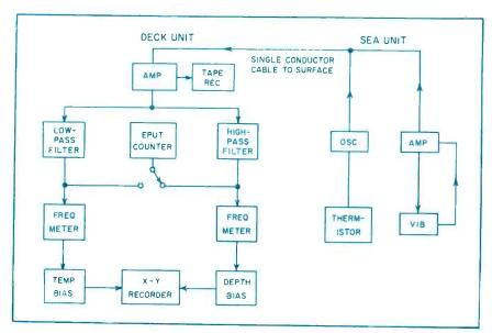
FIG. 1—Outputs of depth and temperature sensing systems are separated in high and low-pass filters for X-Y chart recorder
