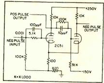
FIG. 2—Functional diagram of Schmitt trigger used in gating unit
