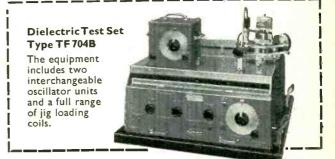
In addition to the investigation of dielectrics, the highfrequency performance of resistors, capacitors, cables, etc., can be determined over a wide range.
