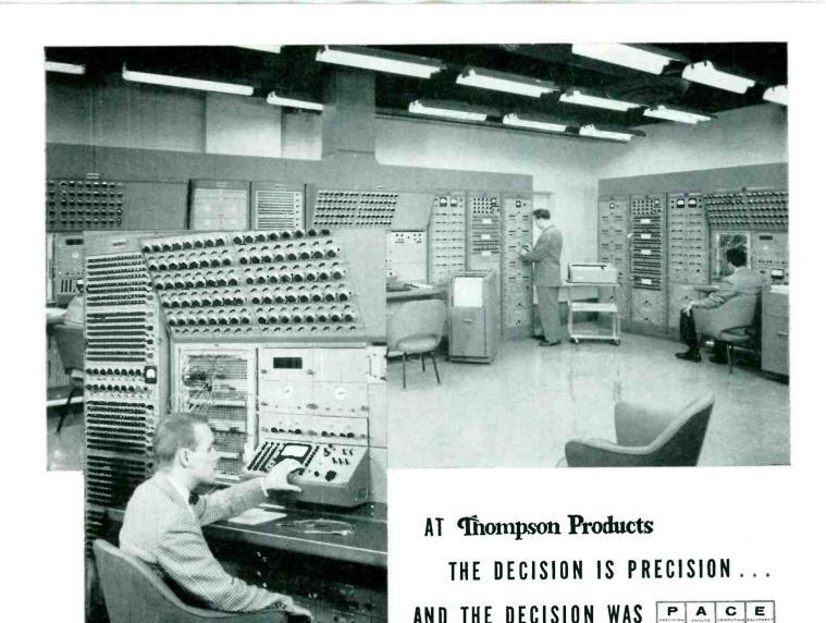
Another example of major industry breaking through the problem barrier: The New Device Research Department, a privately owned laboratory of Thompson Products, Inc., recently placed in operation one of the country's largest analog computing systems devoted to the solution of aeronautical control and nuclear control problems.
