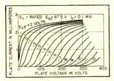
FIG. 9—Average plate characteristics (one section) with plate voltage plotted as abscissa
