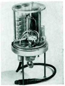
Depth sensing unit with cover removed to show vibrating-wire transducer (center)
