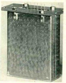
Subassembly encapsulated in alumina sand has high resistance to shock, vibration and nuclear radiation along with 500 C temperature rating. Component leads are welded to wire terminals cemented into holes in ceramic chassis
