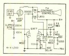
FIG. 1—Simple unprotected circuit for age and sync separation
