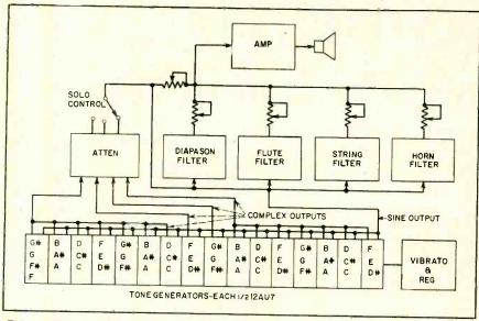
FIG. 1—Sixteen tone generators, each controlled by three adjacent keys, provide basic signals for modification by filters
