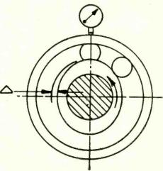
FIG. 2 — Inner raceway is out-ofround, although concentric with bore. ference between the maximum and minimum readings indicates the degree of out-of-round.
