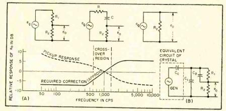
FIG. 3—Networks providing required frequency correction in low, crossover and high-frequency regions (A). Composite network (B) provides all-over correction shown in A
