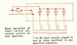
Interlock sequence: Two limit switches are operated alternately. This provides a safety feature. It insures that the movement of the machine has been completed before the Eagle step switch advances.
