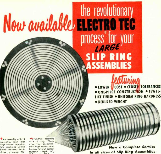
concentric, hard silver rings electro deposited into machined plastic blank. Dovetail locks rings in place. Machined blank insures accuracy. Diameter approx. 11", thickness арргох. 5/16".
