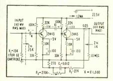
Schematic circuit diagram of the transistor preamplifier with RIAA equalization
