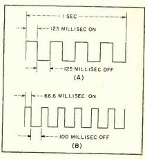
FIG. 1—Pulse times for four (A) and six pps repetition rates (B)
