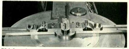
FIG. 5—Rectangular waveguide tubin<mark>g</mark> formed into 180-deg bend, with top plate removed after bending to show bend
