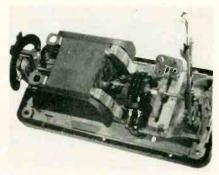
Completed wattmeter movement employing epoxy adhesive bonds in magnetic system
