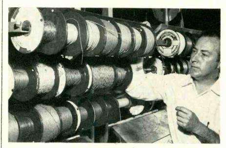
Strips of aluminum over rows of spools stop overrun and prevent wire from slipping over rim onto adjacent spool when operator reaches over harness board to pull down and cut off length
