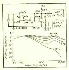
FIG. 6—Crystal pickup is matched through network to transistor preamplifier.
