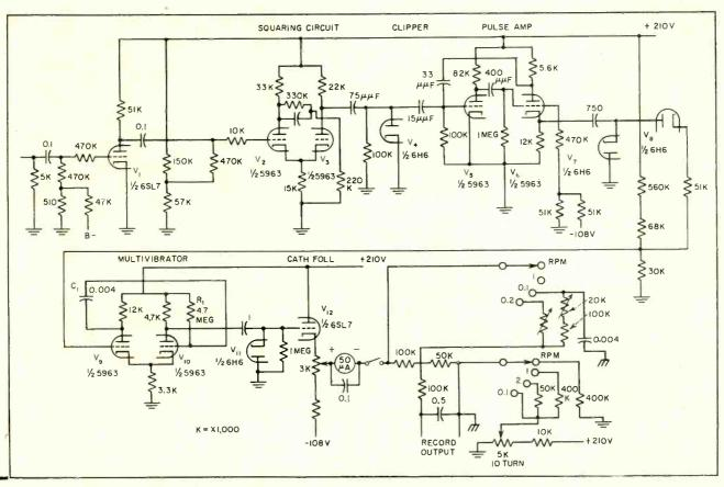
FIG. 2—Squaring circuit, pulse amplifier and multivibrator are constructed as plug-in units for rapid servicing
