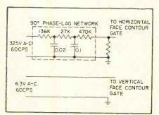
FIG. 2—Generation of face contour signals
