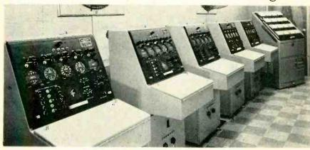
Five monitor consoles and address board (right) used for assigning identities to aircraft at Tacan data-link ground station. Each console displays complete information for a selected aircraft as well as ordered condition
