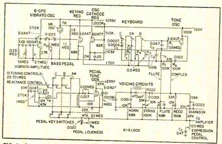
FIG. 2—Organ circuit shows keyboard control of oscillator for key of C. Other keys use similar circuit with different component values
