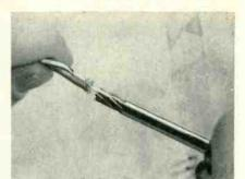
Shearing exposed strands of shielding with modified end mill after crimping ferrules
