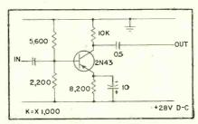
FIG. 7—Typical d-c amplifier circuit. The system employs three iterated commonemitter stages
