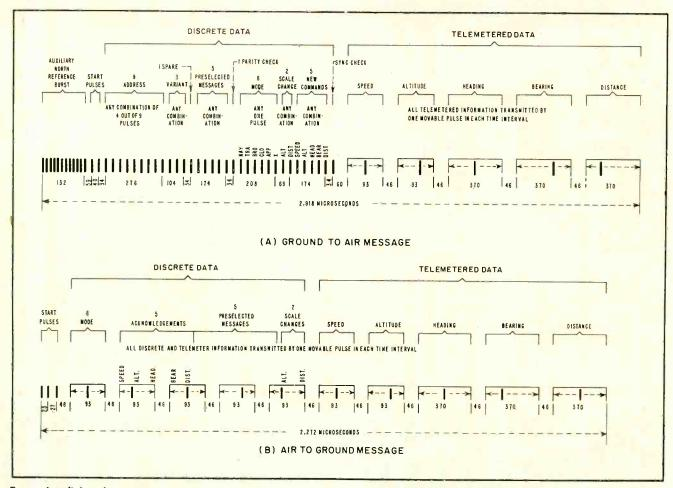
Tacan data-link code structure for ground-air and air-ground messages uses digital and analog codes
