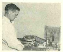
Prototype system developed by Stanford Research Institute duplicates from original text at the rate of 17,000 characters of elite type a second. Signals received on a cathode-ray tube charge a paper ribbon. When dusted with black powder, a sufficient amount clings to the charged areas. The powder is then heated and pressed into the paper to give a permanent record
