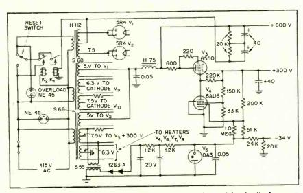
FIG. 3—Power supply for the 90-watt power source. Supply used for the final screens maintains constant screen voltage with a highly variable screen current
