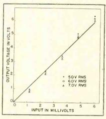
FIG. 4—Chopper drive variation for 5, 6 and 7 volts rms at 400 cps
