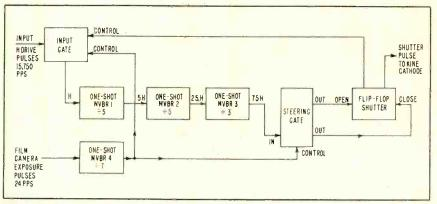
FIG. 1—Pulse from film camera initiates action by unblanking kinescope; multivibrator chain blanks screen after next 525 lines of television picture. Here H represents time of one horizontal line of picture
