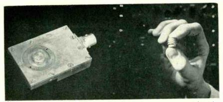
The voltage-tuned magnetron is shown inserted in the balun-ridge waveguide (left) while hand (right) demonstrates size of unit
