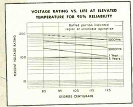
OPERATES FOR 1 YEAR AT 125 C Molded PVZ capacitors are designed for a minimum of one year's life at rated voltage and 125 C operation. Curves shown above are typical of performance.
