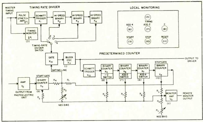
FIG. 1—Gating unit makes extensive use of plug-in circuits marked X in diagram. Panel of indicator box used for local monitoring is illustrated at upper right; lamp numbers correspond to outputs in block diagram
