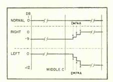
FIG. 3—Attenuation characteristic for solo control in its three positions
