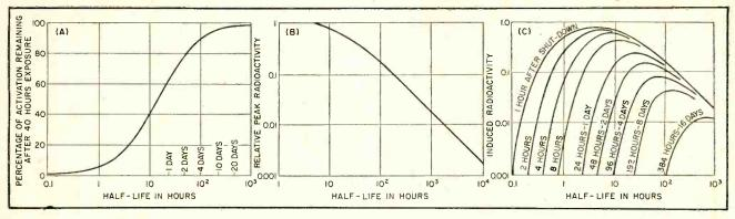
FIG. 2—Residual activation (A), radioactivity at shutdown (B) and relative radiation (C) of materials as a function of half-life
