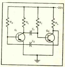
FIG. 2—Basic transistor multivibrator circuit for generator keyer
