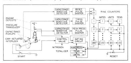
FIG. 2—Block diagram shows how crank angle is quantized into 20 channels that register distribution of peak pressure pulses occurring during ignition
