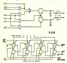
adaptable for use as a composite Grayto-binary code converter and shift register. For this use, the Gray number is read into the shift register in parallel form (for example, from a code wheel or flip-flop register), converted internally to a binary number, and then shifted out in serial form.
