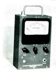
ference within electronic and electrical equipment and on secondary power lines. It will detect interference, between 0.075 mc and 35 mc, of sufficiently high intensity to cause malfunctioning of critical equipment, or to be a potential cause of malfunctioning. It may be used on production lines to compare the order of intensity of interference given off by samples of the same type and thus serve as a means of quality control.
