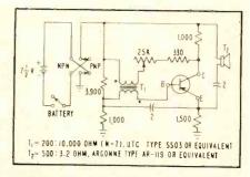
FIG. 2—Complete circuit of the transistor beta tester
