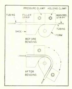
FIG. 3—Setup for bending tubing
