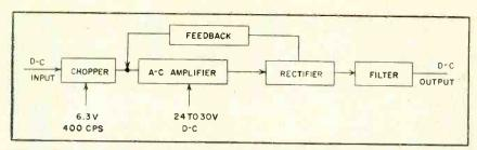
FIG. 1—Block diagram of transistorized chopper system utilizes synchronous modulation of d-c input and demodulation of output from a-c amplifier
