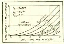
FIG. 11—Plate current plotted against grid-1 voltage shows transfer characteristics of the new tube
