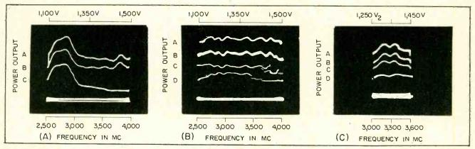
FIG. 1—Waveshapes show power output against anode voltage during wide-band operation in balun-ridge waveguide (A), tapered wave-guide (B) (breaks in C and D are from too-low control voltage) and during narrow-band operation in tapered waveguide (C)
