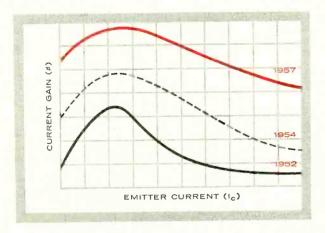
BETA Note the higher Beta or current gain (other factors being equal) derived from today's perfected CBS germanium crystals. Beta is used as just one concrete example of many important performance factors improved by CBS-Hytron's better crystal processing methods.
