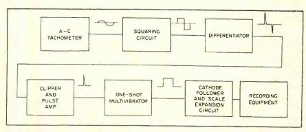
FIG. 1—Block layout of speed indicator, showing waveforms at various points in circuit
