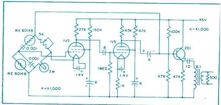
FIG. 4—Wien-bridge oscillator circuit used to measure water temperature. Units encapsulated in epoxy resin and sealed in pressure tight housing.
