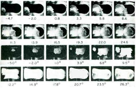
FIG. 1—Part of normal combustion sequence (upper two rows) as viewed through a quartz-headed engine and complex pattern resulting from particle-induced ignition (bottom rows). Numbers represent crank-angle position in degrees during power stroke
