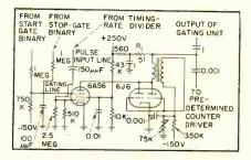
FIG. 5-Combined function diagram of plug-in gate and blocking oscillator
