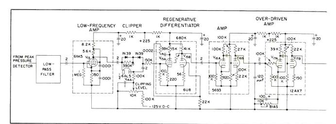
FIG. 5—Capacitor-type transducer detects cylinder pressure variation to drive peak pressure pulse circuit to produce output pulse
