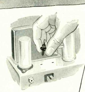
**STUD RECTIFIERS.** Fit them in whereever you need maximum current and temperature in minimum space with rigid chassis mounting.
