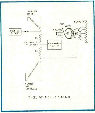
Figure 2. Principle of recorder operation. At the end of each counting period, the staircase voltage generated comes to rest on a step corresponding to the digit displayed by that decade. The number wheel rotates, generating its own staircase. At voltage coincidence, the number wheel is positioned by comparator and solenoid.
