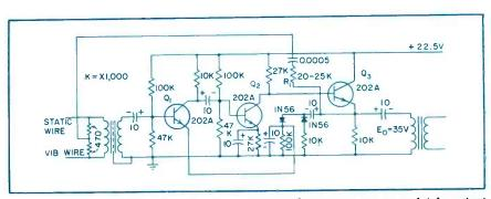
FIG. 2—Transistor amplifier for vibrating wire transducer uses age to maintain output level at constant amplitude
