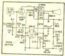
FIG. 7—New type 6BU8 tube simplifies circuit shown in Fig. 5
