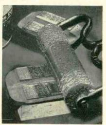
Applying cement to face of Alnico magnet
