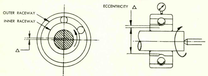
FIG. 1 - Measuring eccentricity of bore with respect to inner raceway.
