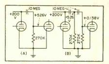
FIG. 3—Two coupling capacitors decrease effect of d-c leakage on grid bias
