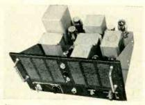
Chassis of 90-watt power amplifier indicates the simplicity and economy of construction, made possible because of the limited frequency applications
