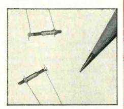
These small capacitors use TEFLON as the dielectric. Their degree of miniaturization is shown by comparison with end of lead pencil.
