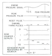
FIG. 3—Simplified timing chart. Pulse generated at peak pressure is gated through synchronized ring counter. Decade counters register coincidence between peak pressure and an open ring stage
