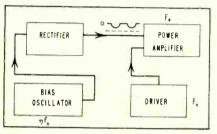
FIG. 2—Negative modulation of grid with high frequency
