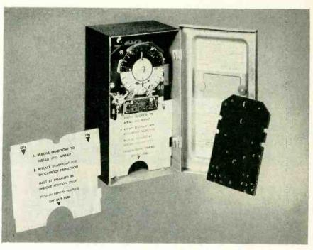
Time switch, made by the Tork Clock Co., uses two Taylor products . . . the deadfront is made of vulcanized fibre for its insulating properties, shock protection and printability . . . the mounting panel of the clock is made of Taylor laminate XP-1-231, chosen for high strength and good punchability.
