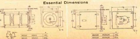
Motor Drives are available for all Type W50 Variacs. ALL motor-driven units include meter capacitor, adjustable-position microswitches to limit the arc of traverse to any desired position, and ball
