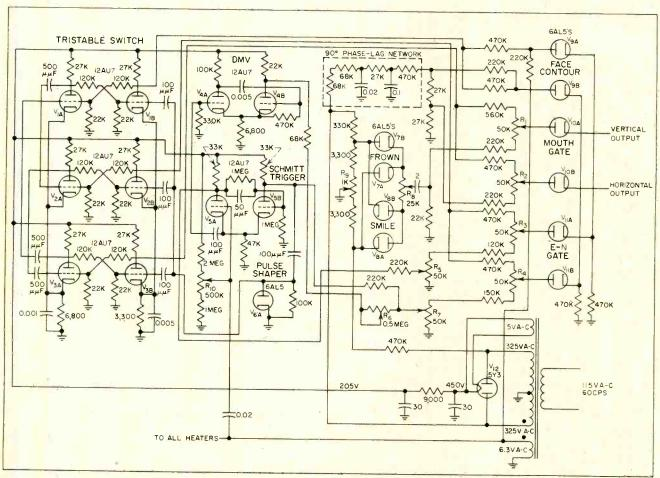
FIG. 7—Schematic diagram of the face generator used with standard oscilloscope
