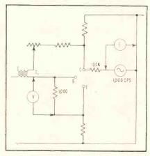
FIG. 3—Circuit shows procedure necessary for accurate calibration
