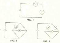
The first is a battery, a thermistor, and a micro-ammeter. The second, more sensitive, has a thermistor as one leg of a bridge circuit. The third incorporates two thermistors in a bridge, making possible even more precise temperature differential measurements.
