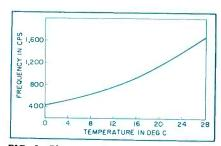
FIG. 5—Plot of oscillator frequency variation with temperature
