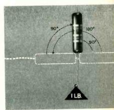
HIGH LEAD BEND RESISTANCE The new capacitors withstand one-pound-vertical-pull test moving the body of the unit 90°, then 180° in the opposite direction, then back 90°, to the original vertical position.
