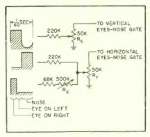
FIG. 5—Method of generating eyes and nose
