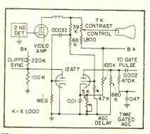
FIG. 2—Impulse noise is time gated but vertical sync output suffers
