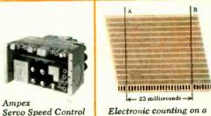
Servo Speed Control equipment as used on the FR-100 Recorder.
