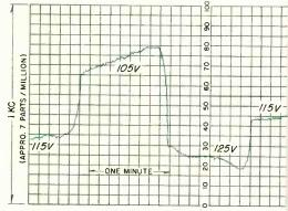
Figure 1. Frequency stability vs. line voltage; 150 MC oscillator
