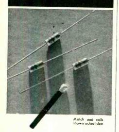
Here is a Standardized Series of Molded RF Choke Coils that make other coils look like giants—take up less than half of the space of the next smallest molded coil. Yet these midgets do a big job! Current ratings range to 1800 milliamperes; inductance ranges from 0.15 to 22.0 microhenries. 23 distinct coils (All RETMA standard values). All electrical perimeters are exactly defined.
