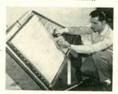
An 18 by 24-in. grid of transverse parallel wires spaced regularly over a conducting sheet comprises a flush-mount antenna developed for the Air Force by Stanford Research Institute. Used for radar, the antenna has a pencil-beam pattern with low side lobes. Mounted horizontally, it can be scanned over 40 degrees by changing frequency between 7 to 13 kmc
