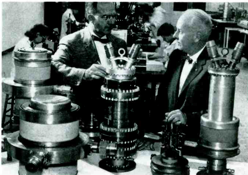
One megawatt c-w at 425 mc can be generated by the tube in the left foreground. On the extreme right is a 1.5 megawatt tube used in atom-smashing particle accelerators. Other RCA tubes shown are designed for delivering up to 15 kw at 500 mc in color television service
