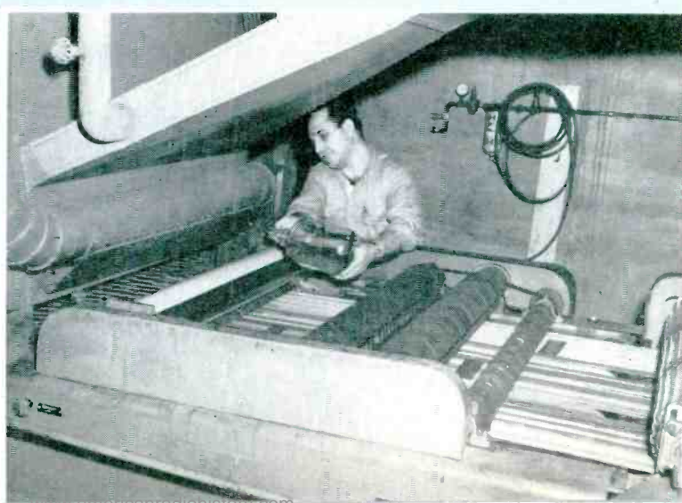
BOARD PROCESSOR —Punched boards loaded in racks at input of machine are transferred to open-mesh conveyor by vacuum fingers for spray degreasing, deoxidizing and washing, followed by hot-air drying. Boards are next realigned and spaced by cam disks and roll-coated with flux (lower right), then dried on fingers of vertical oven conveyor and ejected onto conveyor belt for stacking.
