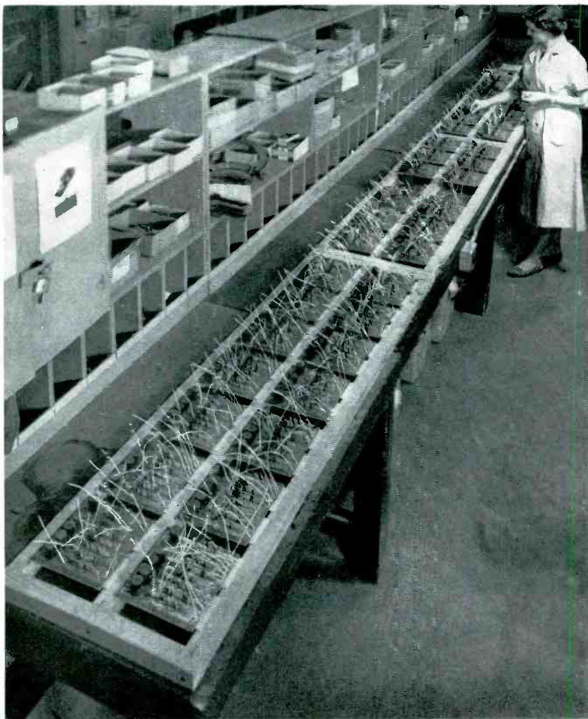
Wood frames hold wiring boards above surface of work table so that operator can walk along the table inserting the same component in each board in turn. Leads are not crimped because boards have wiring on both sides
