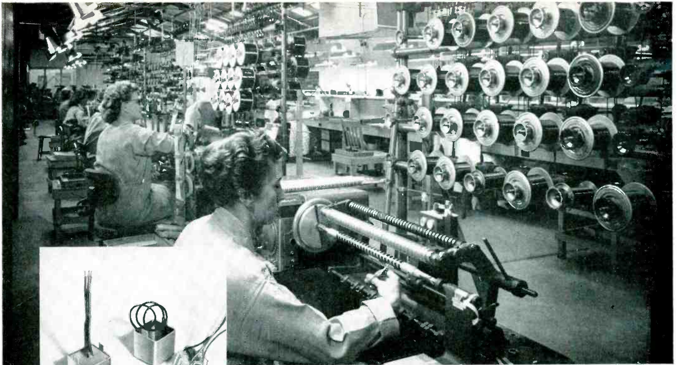
An Installation of Leeson Coil Winders in the Lenkurt Electric Company plant, San Carlos, Calif. Inset shows, left to right: a Lenkurt miniaturized high frequency transformer fully assembled; the transformer casing; and the transformer coil, precision-wound to extremely close tolerances on a fast Leeson No. 108 Hand Feed Coil Winder.
