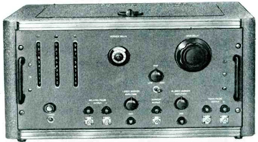
Time measuring equipment using interleaved pulse technique for accurate timing
