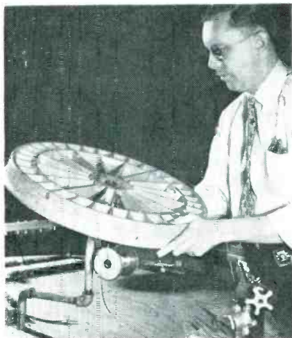
Placing tray on supporting pipe that comes up through hole in center of caster-mounted rotating assembly turntable. Tray here tilts toward operator
