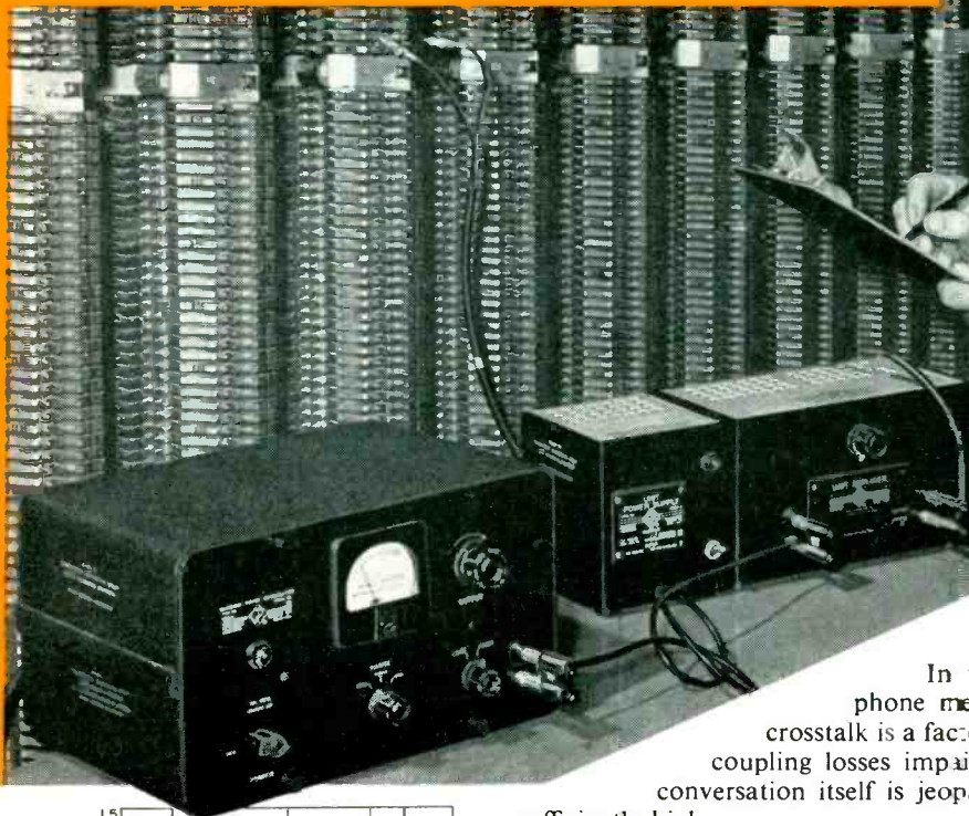
G-R Random Noise Generator and Unit Amplifier in toll-cable crosstalk measurements at General Telephone Company.
