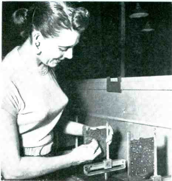
COMPONENT ASSEMBLY —Stacks of coated boards feed automatically through modified Malco wire-wrap terminal inserter. After sockets are put in, boards are loaded into United Shae assembly machine. Additional components are inserted manually on conveyor having vertical board holders that simplify clinching of leads with thimble
