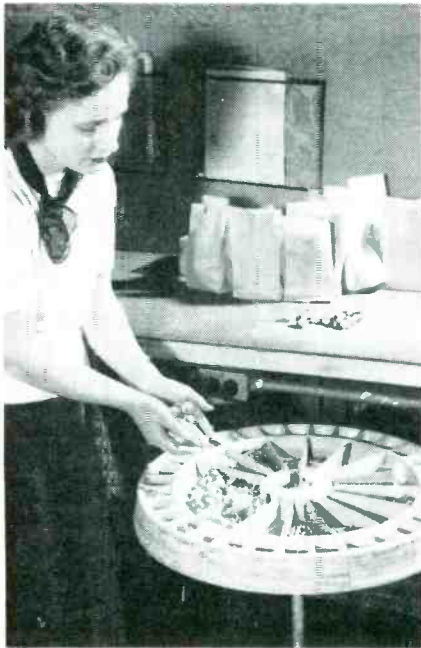
Loading parts into compartments of circular plastic tray. Plastic dividing strips in center section are removable
