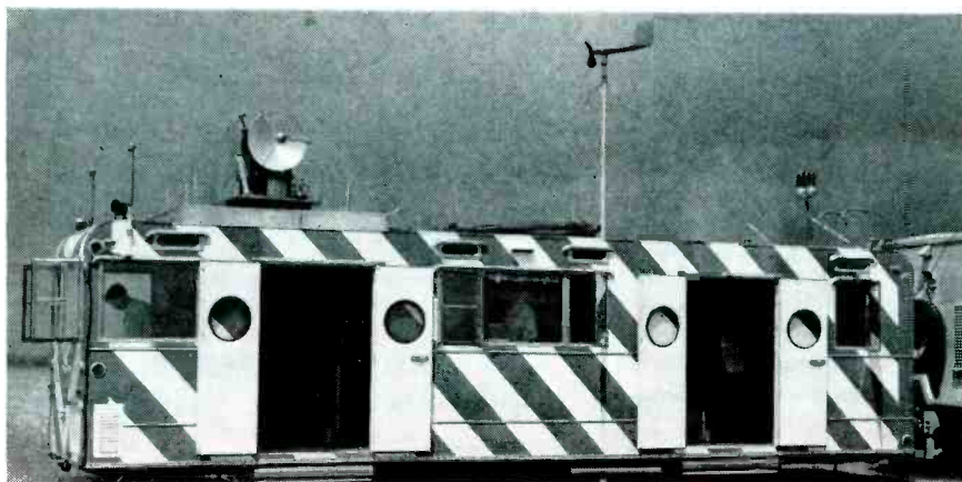
Automatic carrier landing system developed by Bell Aircraft uses radar and radio equipment for all-weather flights. Aircraft is located by radar on carrier and information on its location is fed into computer to show relationship to carrier deck. Automatic signals direct the craft down the proper path and land it
