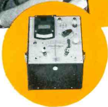
The Breathalyzer is an instrument for determining immediately the degree of alcoholic intoxication. This instrument is used widely by law enforcement agencies and Laboratories.
