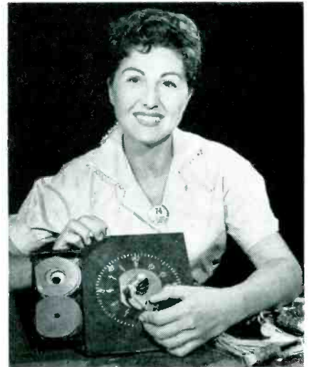
Plug-holding fixture, with calibrated dial, can be set anywhere on bench or on wiring harness board, to hold plug at correct angle. Removable inserts are stored in compartment alongside fixture
