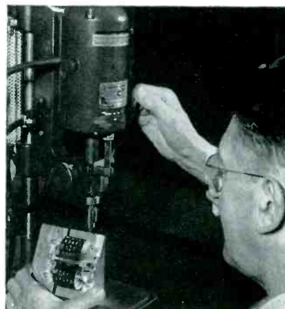
Universal holding fixture provides support and correct angles for many drilling operations on counter at Ford Instrument Co.
