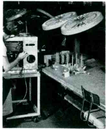
Circular trays mounted at an angle on tiny trolley cars riding on rails above bench can easily be moved to various work positions as heavy units on floor carts are moved along assembly bench
