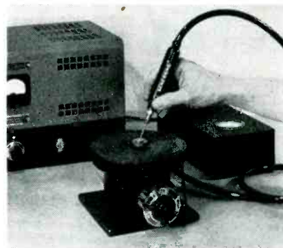
Soldering silicon disk with 12-watt ultrasonic unit. Heat is provided by electric hot plate
