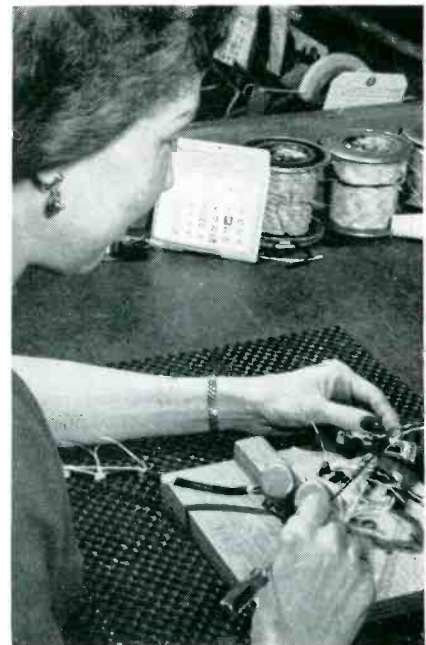
Screwdriver-handled version of needle is used here for pulling additional leads through short length of vinyl tubing during modification of completed harness
