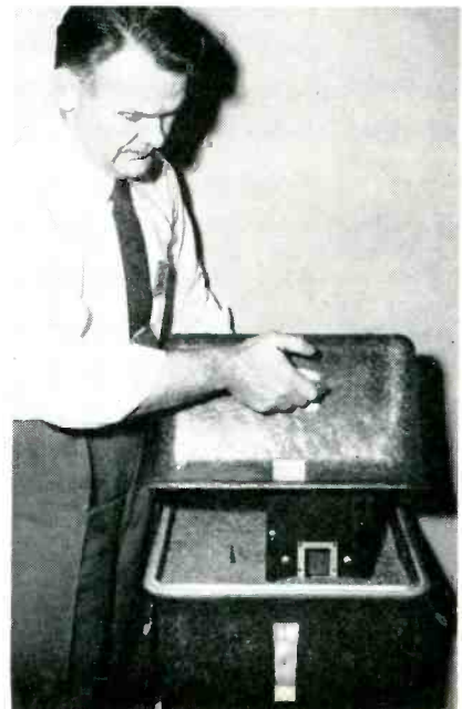
GE packaging engineer Richard H. Thomas demonstrates how top cover is closed after setting electronic unit in recess of rubberized fiber inner cushion
