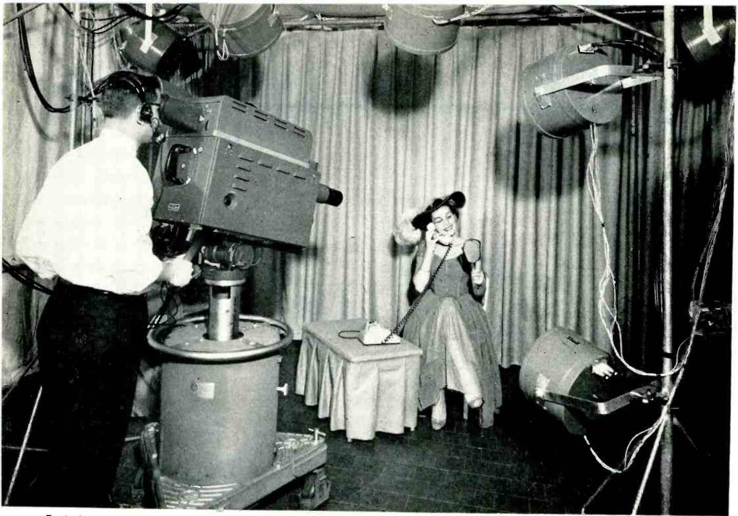
Typical studio setup uses conventional tv camera housing as flying spot source. Strobe units provide general lighting during blanking
