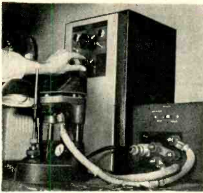
Operator adjusts spotwelder controls. Welding transformer is in box at right
