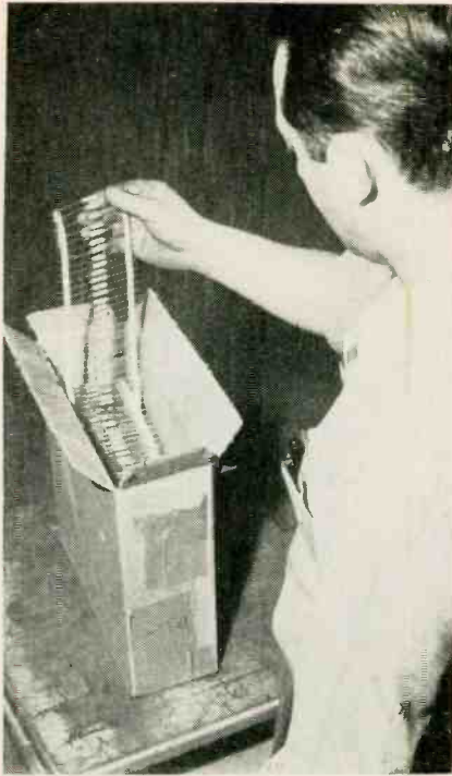
Experimental ammunition pack for video peaking coils having lead belting. Components stack automatically as belt is lowered
