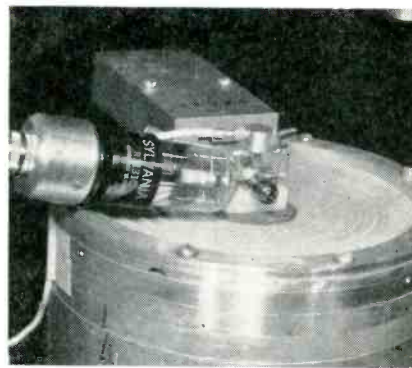
Miniature tube on vibrator is illuminated by glow modulator tube on left for examination under vibration conditions
