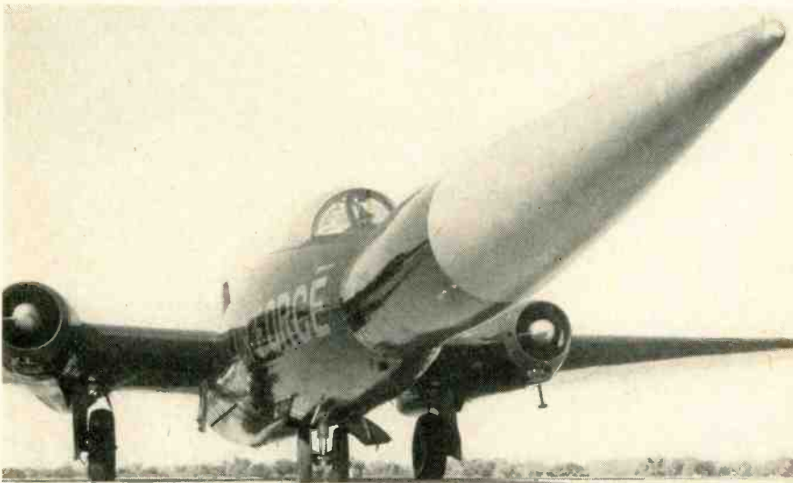
BOMARC-NOSED B-57 Canberra jet bomber, modified by Temco Aircraft, tests guidance system as . . .
