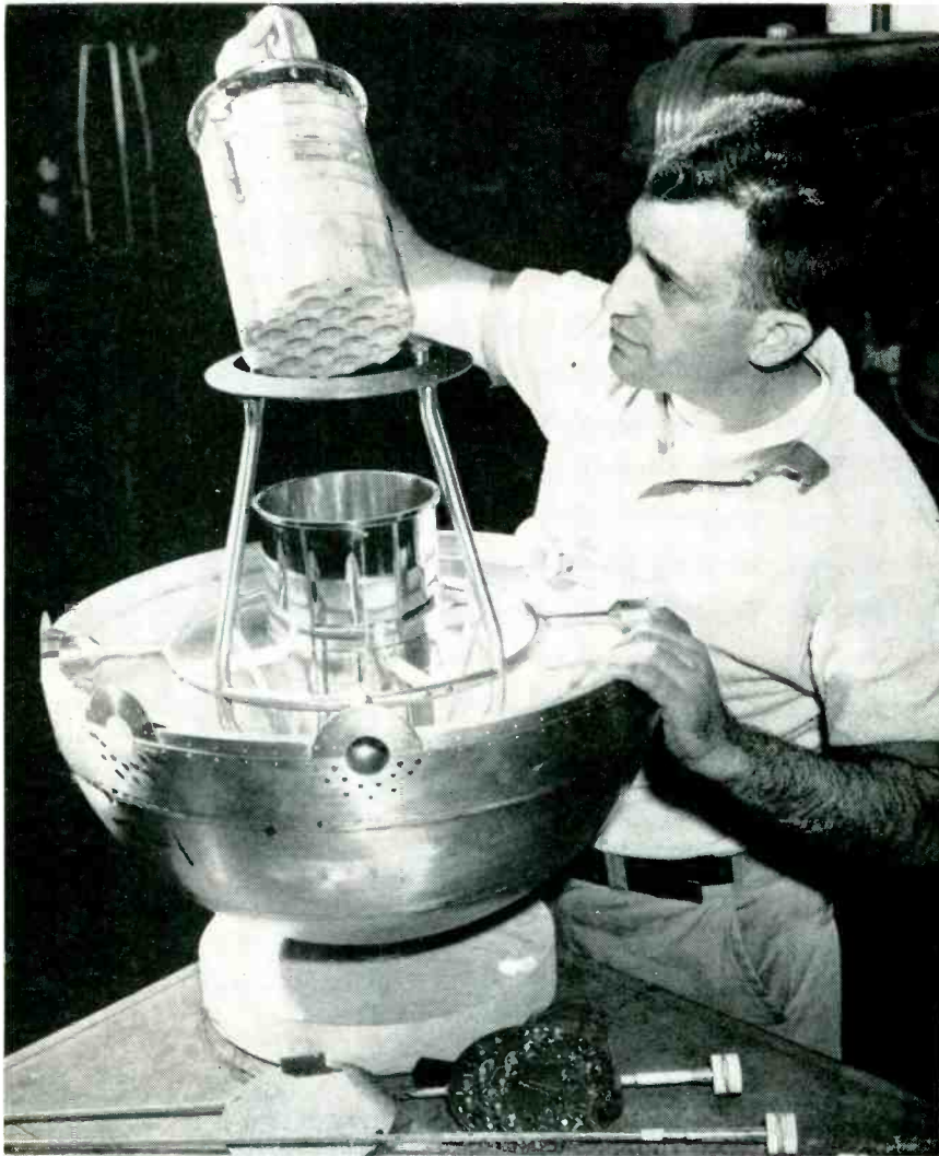
Electronic circuit package held by Naval Research Lab employee fits into baby-moon shell shown below. Printed wiring typical of that used can be seen on boards at bottom of picture. Eighteen units of this kind are now under construction. They will be launched from three-stage rockets during the International Geophysical Year
