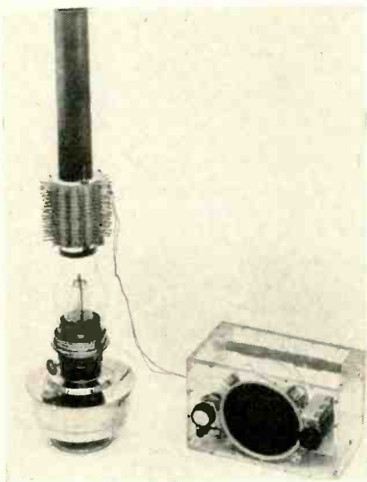
Metal tube and thermopile, mounted on glass chimney of paraffin lamp, utilizes wasted heat to operate transistorized radio. (ELECTRONICS, p 196, May, 1946) Receiver, developed by The Philips Industries, uses 7 transistors
