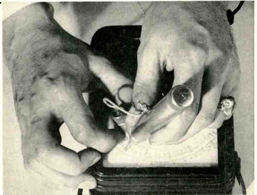
To read a meter the plastic card with embossed indices is placed over the glass face of the meter and the location of the pointer found and related to the raised marks. Any meter can be used without alteration
