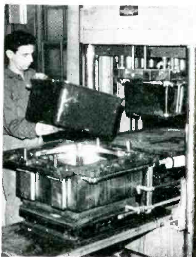
Removing container half from mold, completely finished and ready for attachment of hardware
