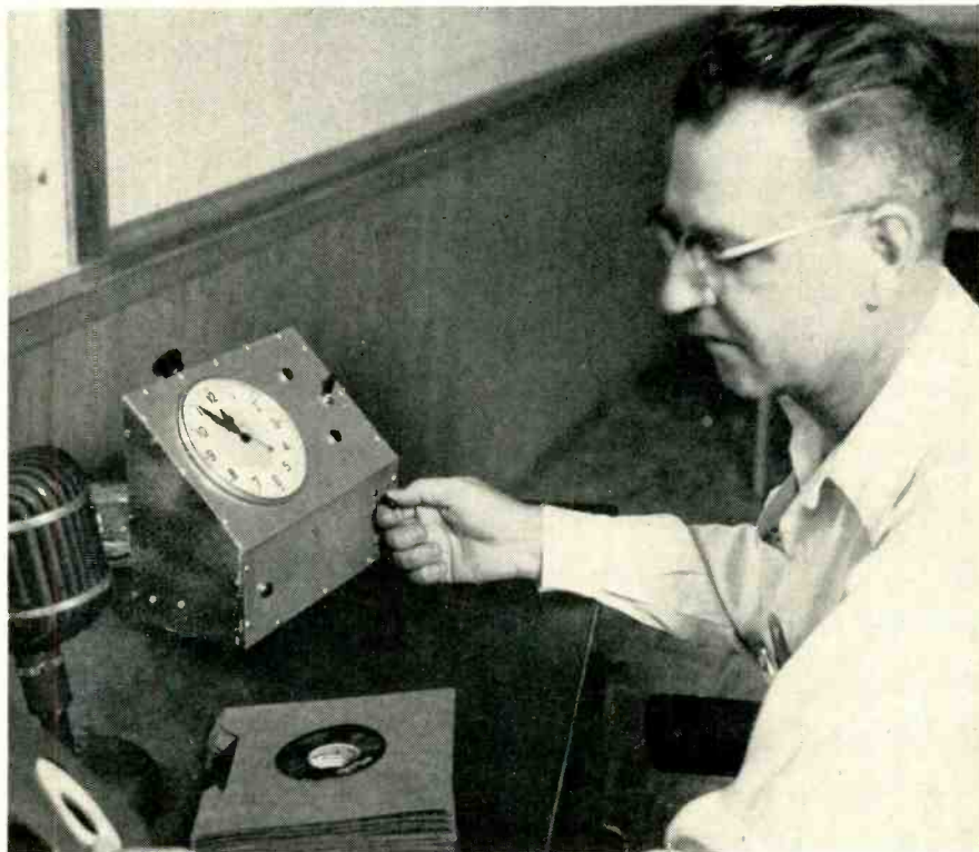
Small recording console controls tape recorder, inserts tones and indicates elapsed time during recording of announcements
