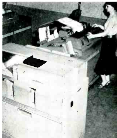
Mark sense reproducer machine in foreground converts pencil-marked cards into standard punched cards suitable for machine at rear that is printing data summary on special report sheet
