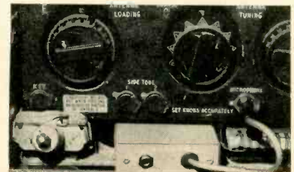
Speech compressor mounted beneath transmitter feeds microphone input
