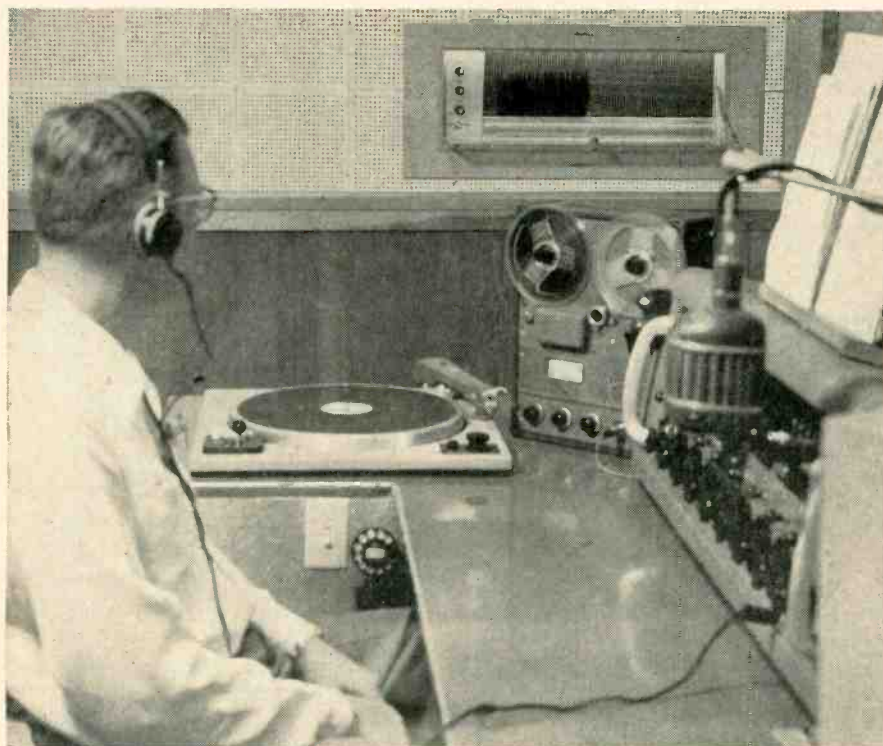
Automatic programming system uses portable tape recorder and automatic record selector-player mounted on wall
