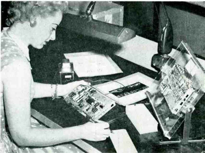
Inspection position at which defects in airborne unit of Tacan equipment are marked on inspection record card. Complete unit mounted in quick-flipover plastic enclosure provides convenient visual comparison guide
