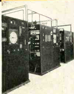
NITRONEAL® GAS GENERATOR economically and safely provides fully automatic furnace brazing and bright annealing of stainless steel.
