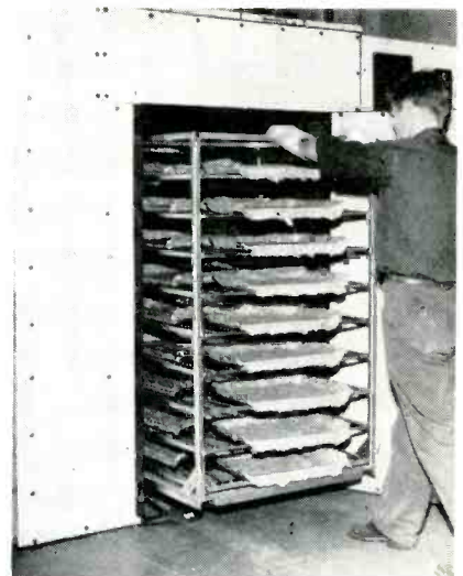
Preformed sides, tops and bottoms for containers are oven-dried for 65 minutes at 160 C
